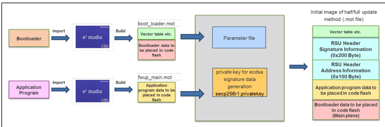
**Figure 5.5 Initial image of partial/ full update method**
