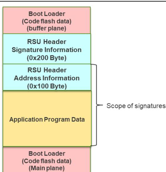
**Figure 5.4 Composition of initial image file (dual-bank(2-bank) method)**
