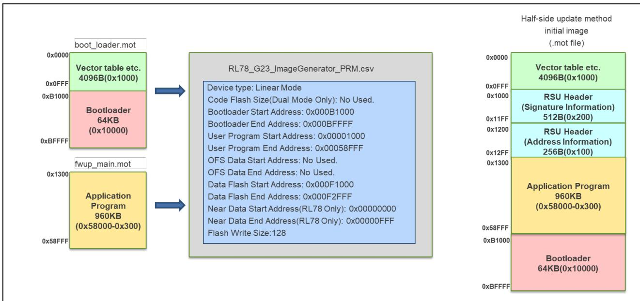
Figure 5.8 Example of parameters referred to when generating the initial image of RL78/G23 partial update method
