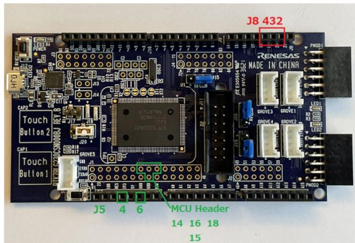
Figure 6.2 RL78/G23-128p FPB Device Connection Pin Information
