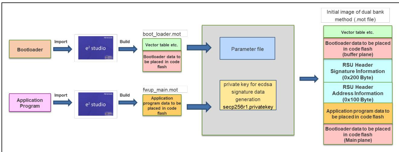
**Figure 5.6 Initial image of dual-bank(2-bank) method**
