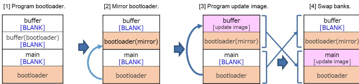
**Figure 1.9 Initial Firmware Update Settings Utilizing Bootloader (Example of Dual-Bank(2-Bank) Method)**
