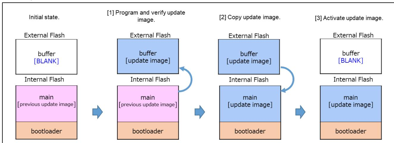
**Figure 1.5 Operation of Full Update Method (buffer plane is external flash)**
