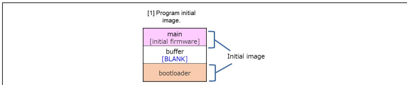
**Figure 1.7 Initial Firmware Update Settings Utilizing Renesas Image Generator (Example of Partial Update Method)**
