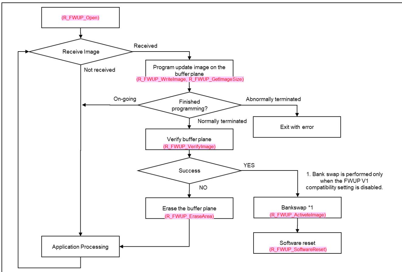
**Figure 2.2 Application Program Implementation Example of Dual-Bank(2-Bank) Method**
