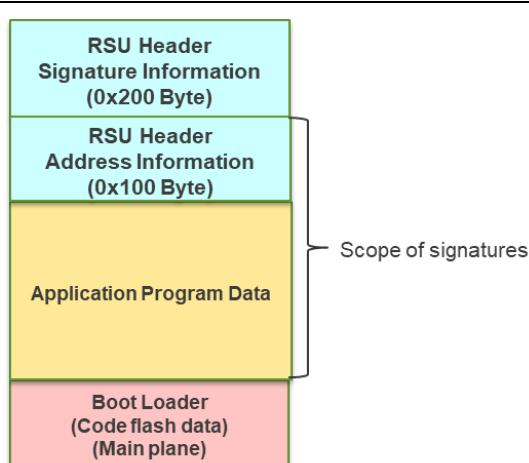
**Figure 5.3 Composition of initial image file (partial / full update method)**
