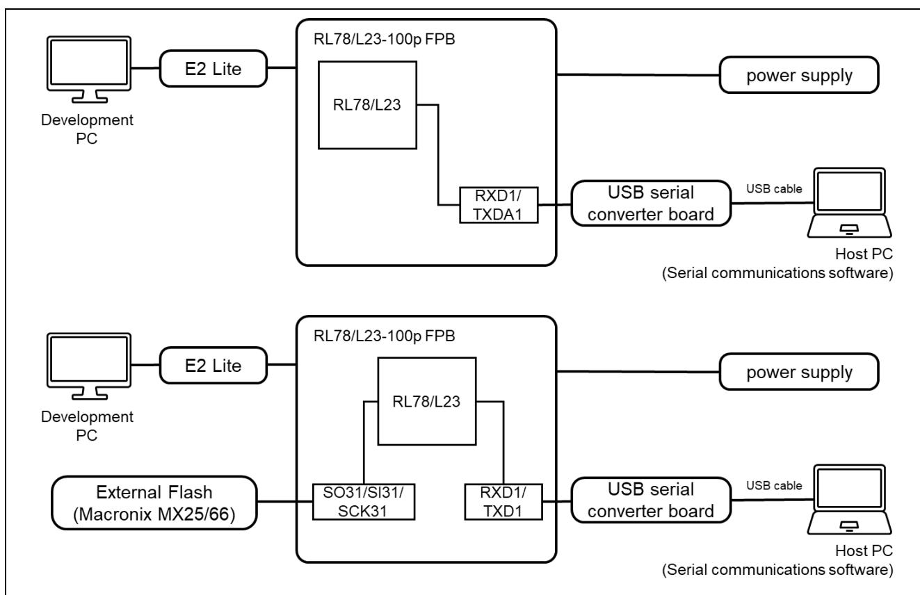
Figure 6.14 RL78/L23-100p FPB Device Connection Diagram
