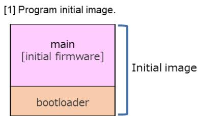
**Figure 1.8 Initial Firmware Update Settings Utilizing Renesas Image Generator (Example of Full Update Method)**
