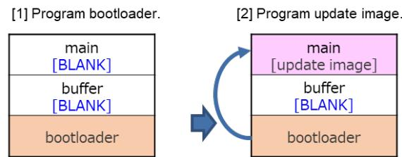
**Figure 1.10 Initial Firmware Update Settings Utilizing Bootloader (Example of Partial Update Method)**
