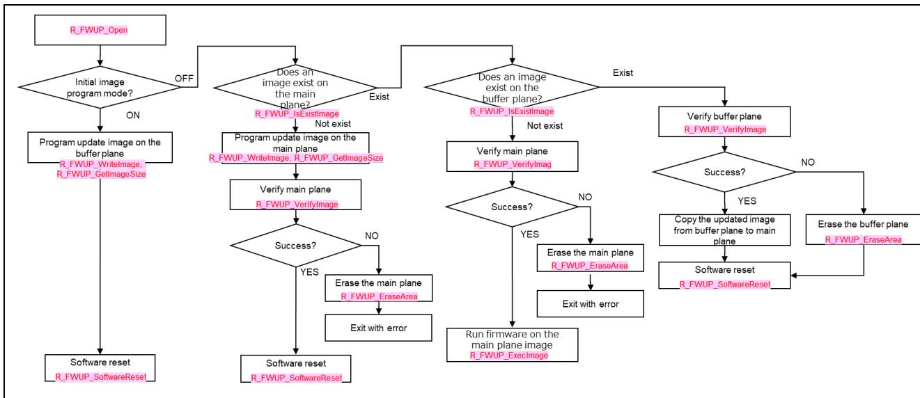
**Figure 2.3 Bootloader Implementation Example of Partial/Full Update Method (with buffer plane)**
