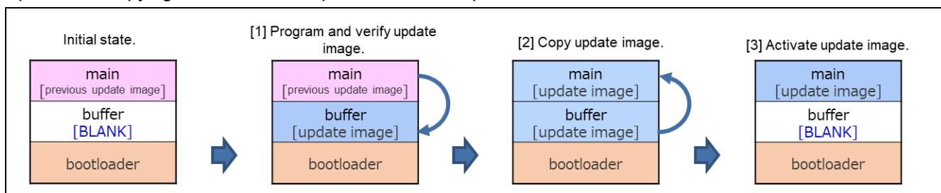
Figure 1.3 Operation of Partial Update Method (buffer plane is internal flash)
