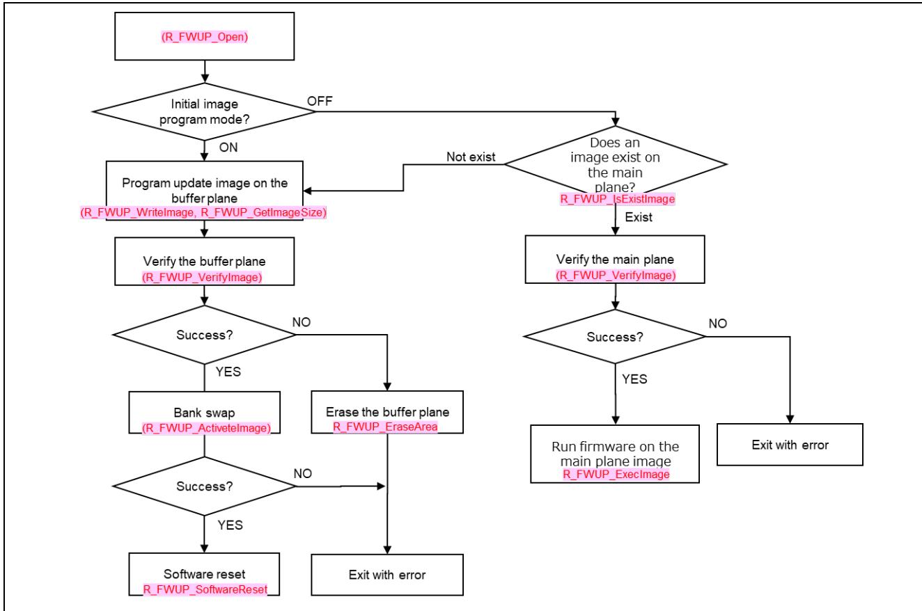
**Figure 2.1 Bootloader Implementation Example of Dual-Bank(2-Bank) Method**
