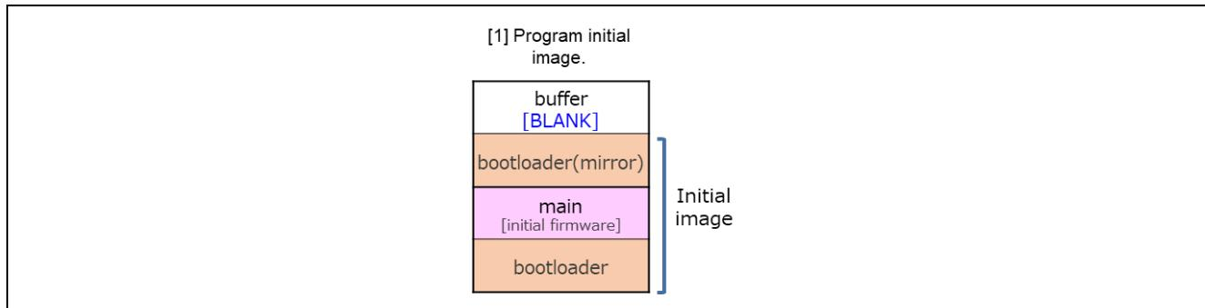
**Figure 1.6 Initial Firmware Update Settings Utilizing Renesas Image Generator (Example of Dual-Bank(2-Bank) Method)**
