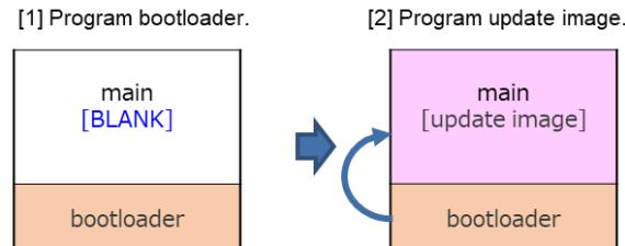
**Figure 1.11 Initial Firmware Update Settings Utilizing Bootloader (Example of Full Update Method)**
