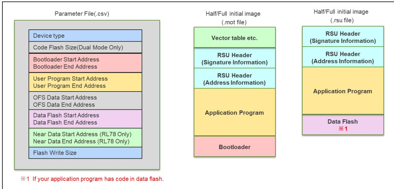
**Figure 5.7 Parameters referenced when generating image files**
