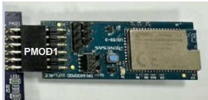
Figure 4-2 Connecting DA16600MOD to PMOD1 of the MCU Board
