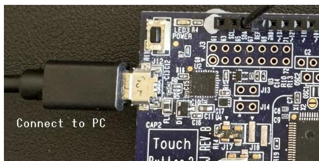
Figure 4-6 Supplying Power to the MCU Board
