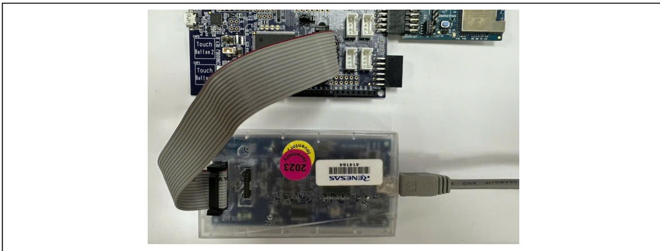
Figure 8-5 Connecting Emulator to MCU Board
