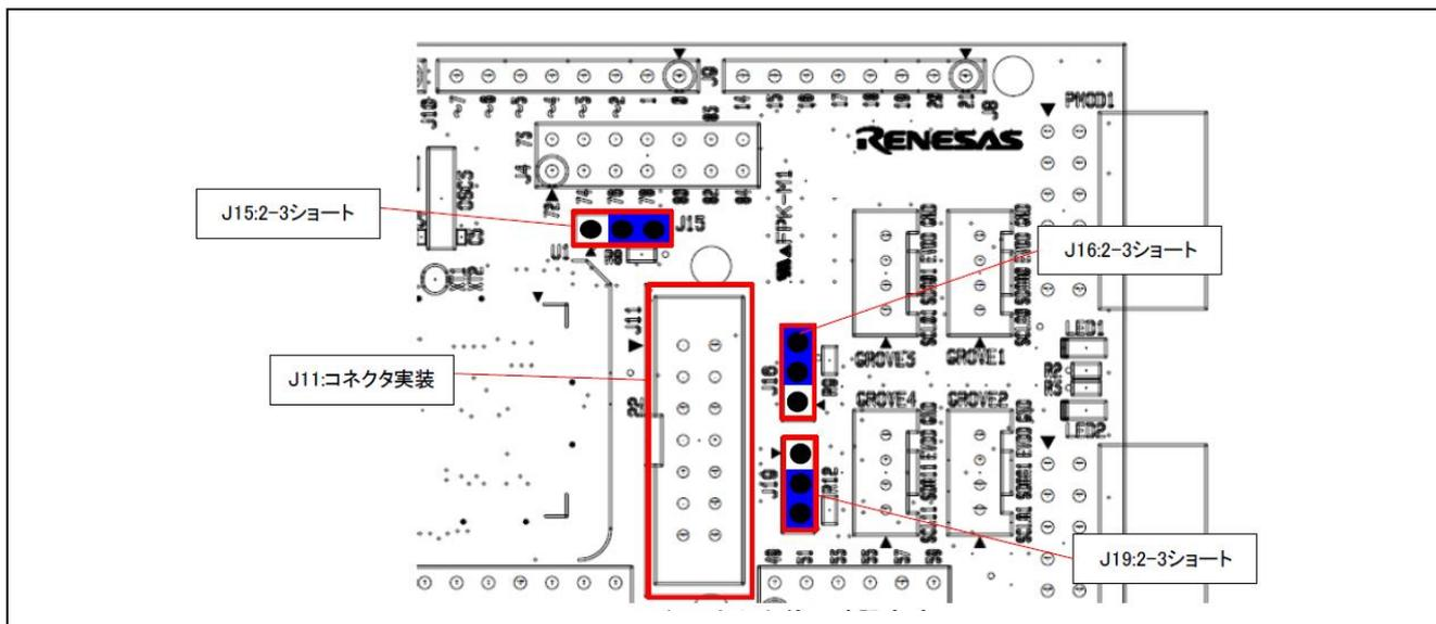
Figure 7-6 Settings for Using Emulator Connector (Top Side)
