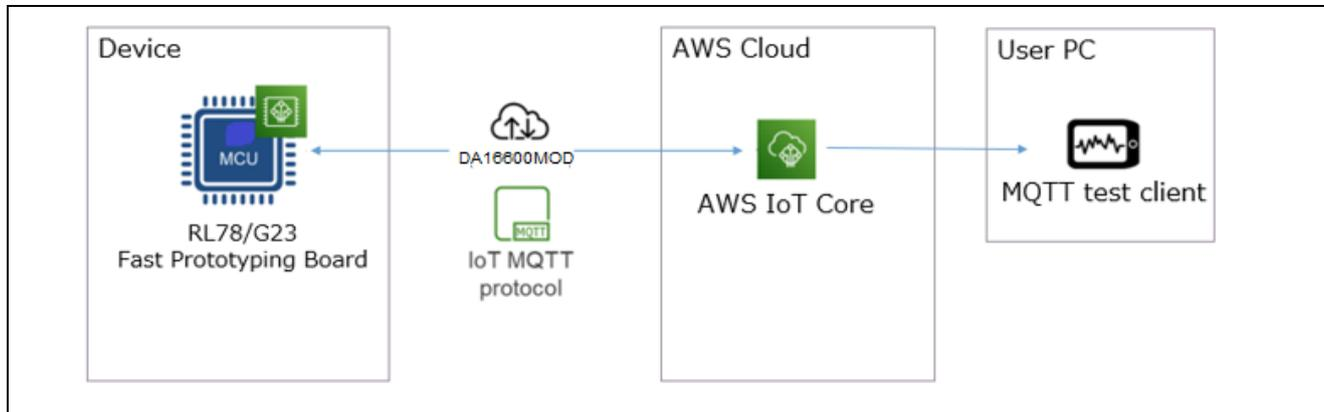
Figure 2-1 System Configuration of Demo Project (PubSub)
