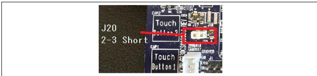
Figure 4-4 Setting MCU Board Power Supply to 3.3 V
