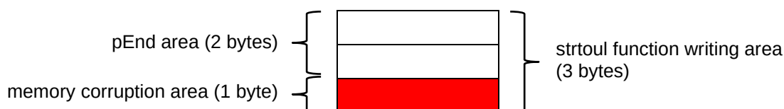
Figure 9-4 Memory corruption due to example of W0520167
