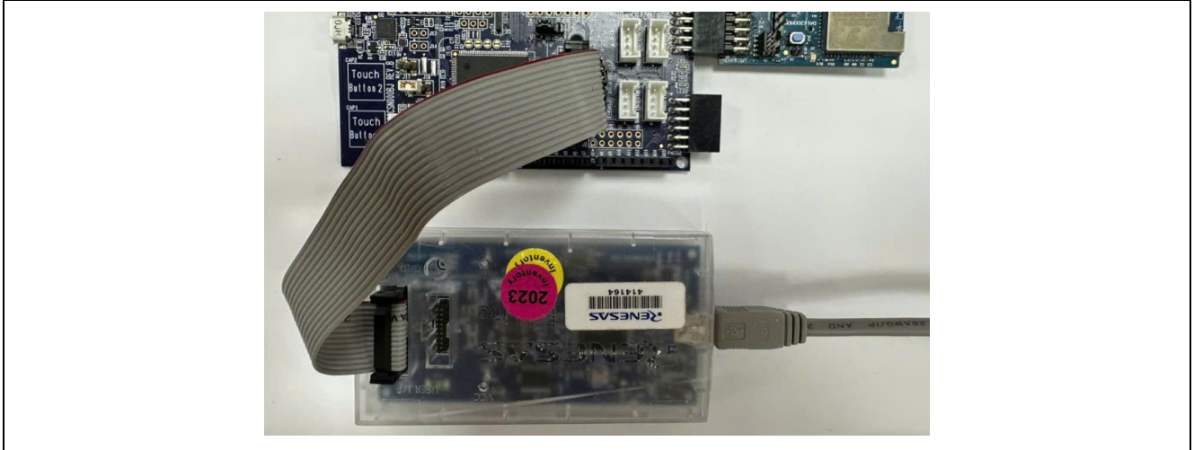
Figure 8-5 Connecting Emulator to MCU Board
