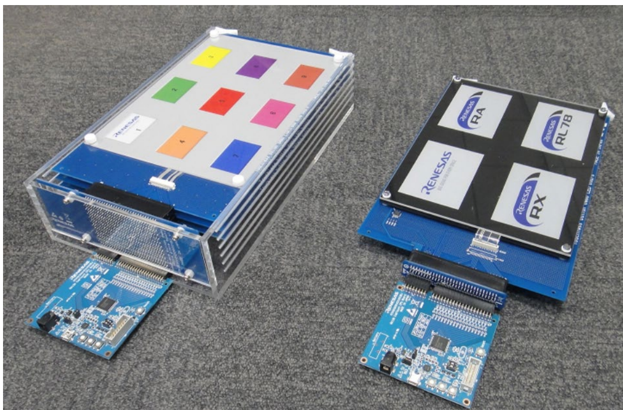
Figure 1.1 Touchless Button Electrode Board (Left: with housing, Right: without housing)
