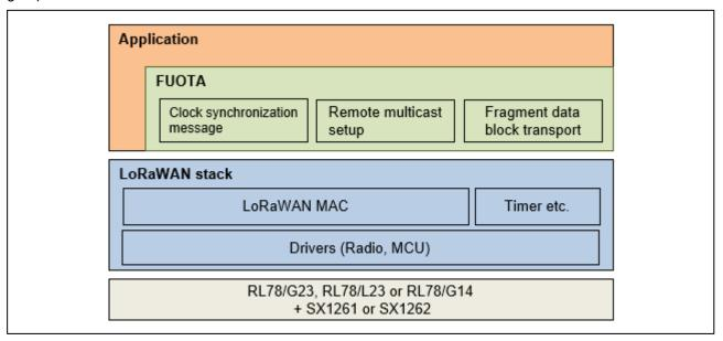
Figure 5 FUOTA Sample Application Block Diagram
