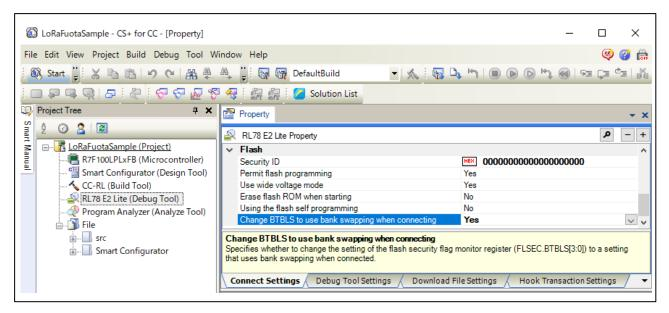
Figure 26 Configuration to Put into Bank Programming Mode in case of CS+ (Bank Swap Mode)
