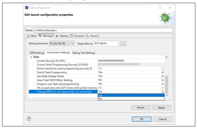
Figure 25 Configuration to Put into Bank Programming Mode in case of e2studio (Bank Swap Mode)
