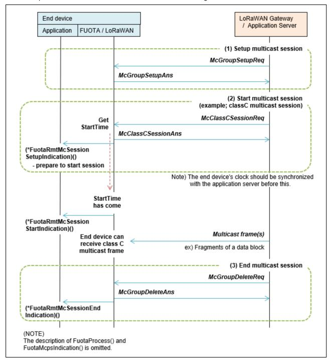
Figure 9 Remote Multicast Setup
