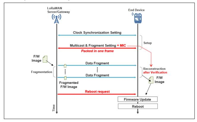
Figure 29 FUOTA V2.0.0 Message Exchange between LoRaWAN Network Server and End Device
