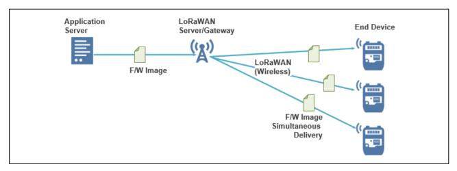
Figure 1 Overview of FUOTA in LoRaWAN Network Architecture
