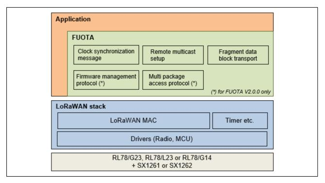
Figure 30 FUOTA V2.0.0 Sample Application Block Diagram
