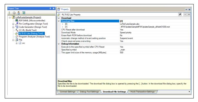
Figure 23 Configuration of Object Files to be Download in case of CS+ (Boot Swap Mode)
