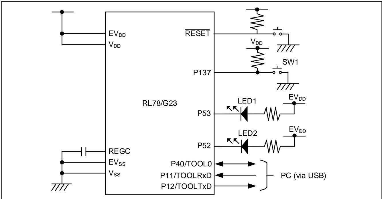
Caution 1. This simplified circuit diagram was created to show an overview of connections only. When actually designing your circuit, make sure the design includes sufficient pin processing and meets electrical characteristic requirements. (Connect each input-only port to  $V_{DD}$  or  $V_{SS}$  through a resistor.)
