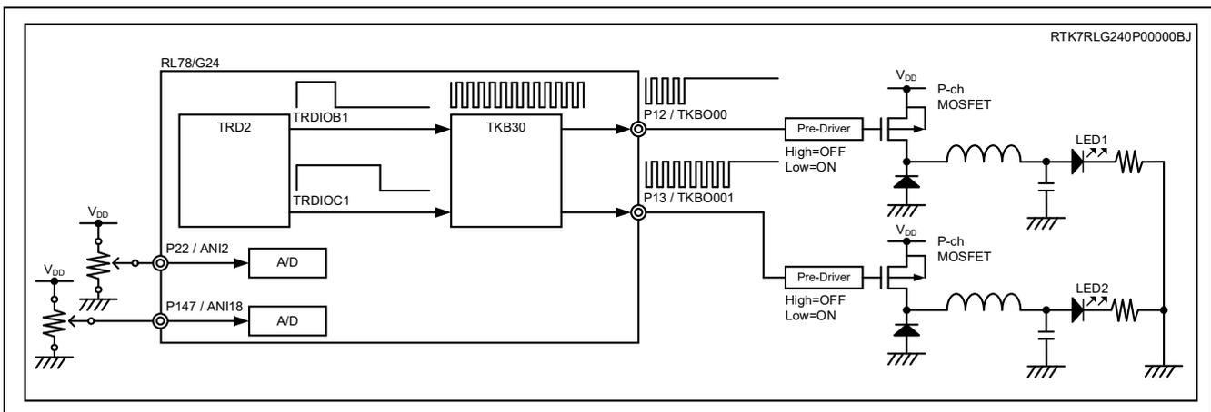
**Note** By using “RL78/G24 DC/DC LED DC/DC LED Control Evaluation Board”, it is possible to operate the evaluation board standalone without the need for circuit assembly. For details, please refer to “RL78 Family RTK7RLG240P0000BJ RL78/G24 DC/DC LED Control Evaluation Board User’s Manual”.
