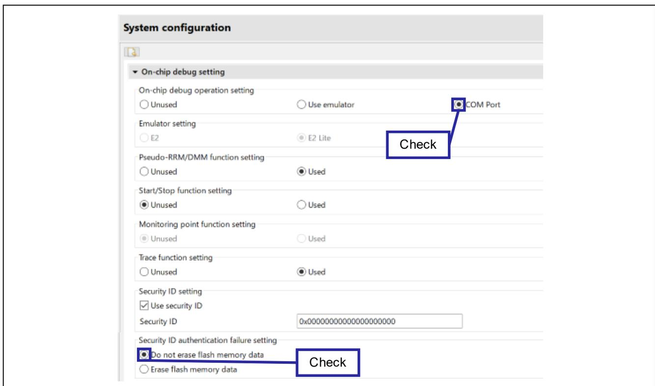
Figure 4-2 shows the system configurations used in this sample program for IAR.
