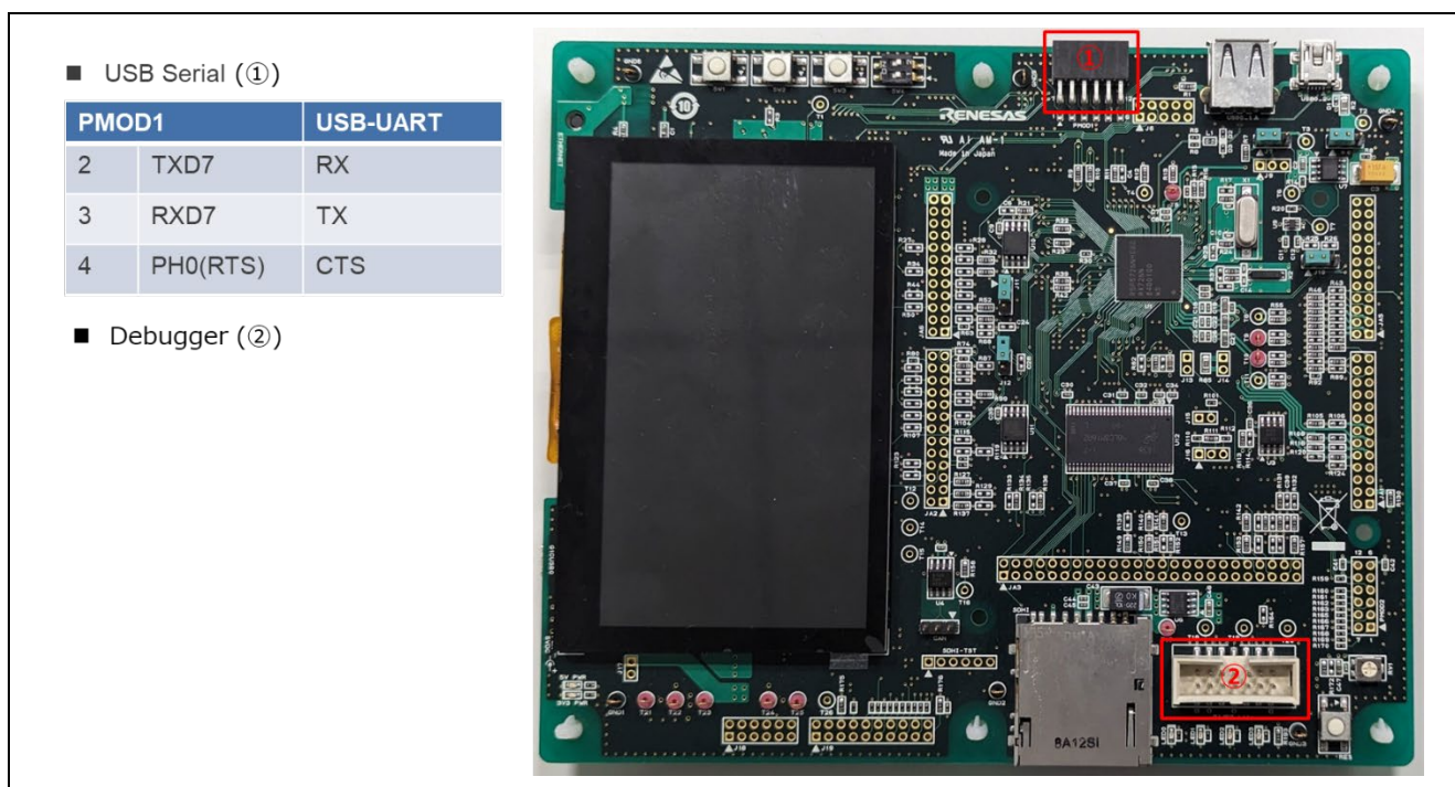
Figure 5-23 Information on Hardware Component Connections for the RSK-RX72N When the Update Method Uses Linear Mode
