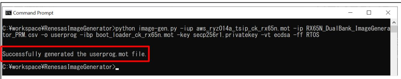
**Figure 6-17 Generating the Initial Firmware**
