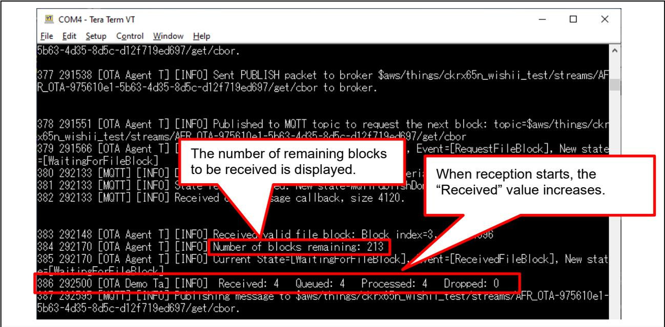
Figure 6-47 Log Data Displayed During Firmware Reception
