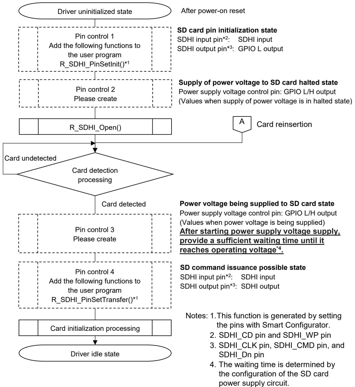
Figure 4.1 SD Card Insertion and Power-On Timing
