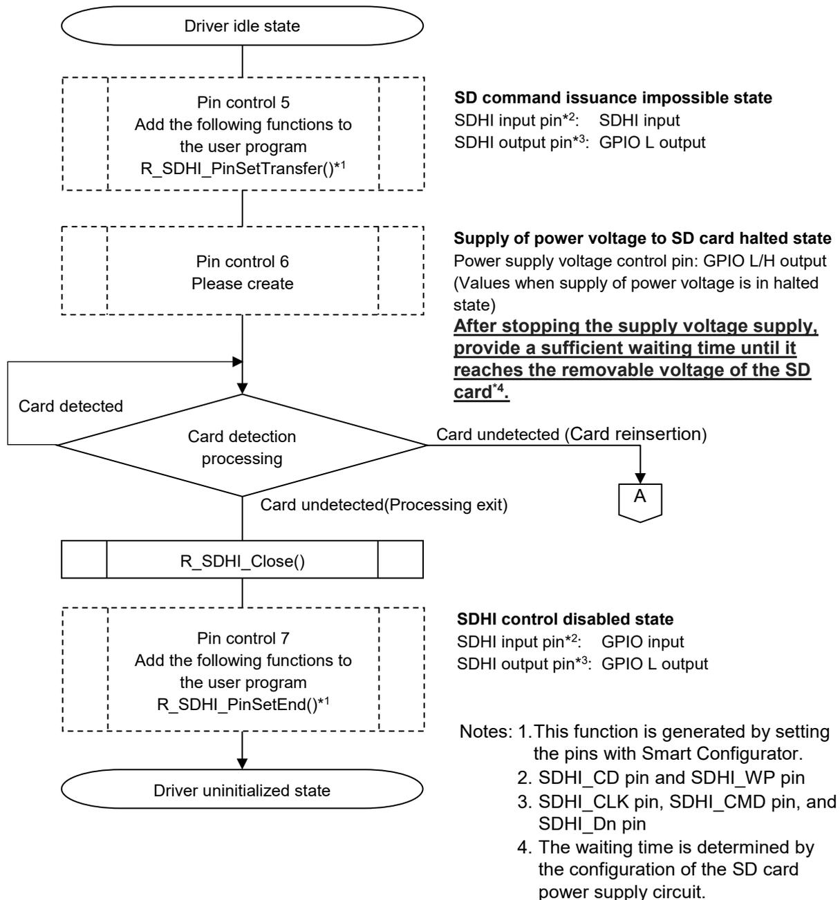
Figure 4.2 SD Card Removal and Power-Off Timing
