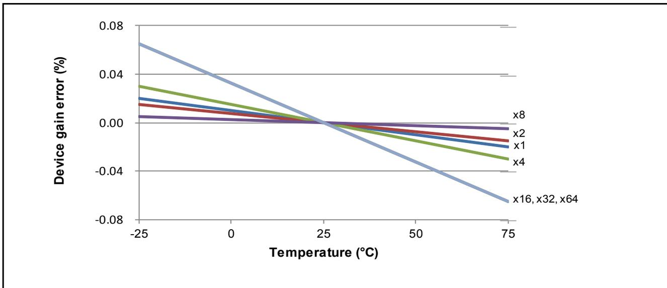
Figure 7.2 Theoretical Temperature Characteristics of the Device Gain When the Reference Voltage (VBG) Assumes to Have No Temperature Characteristics
