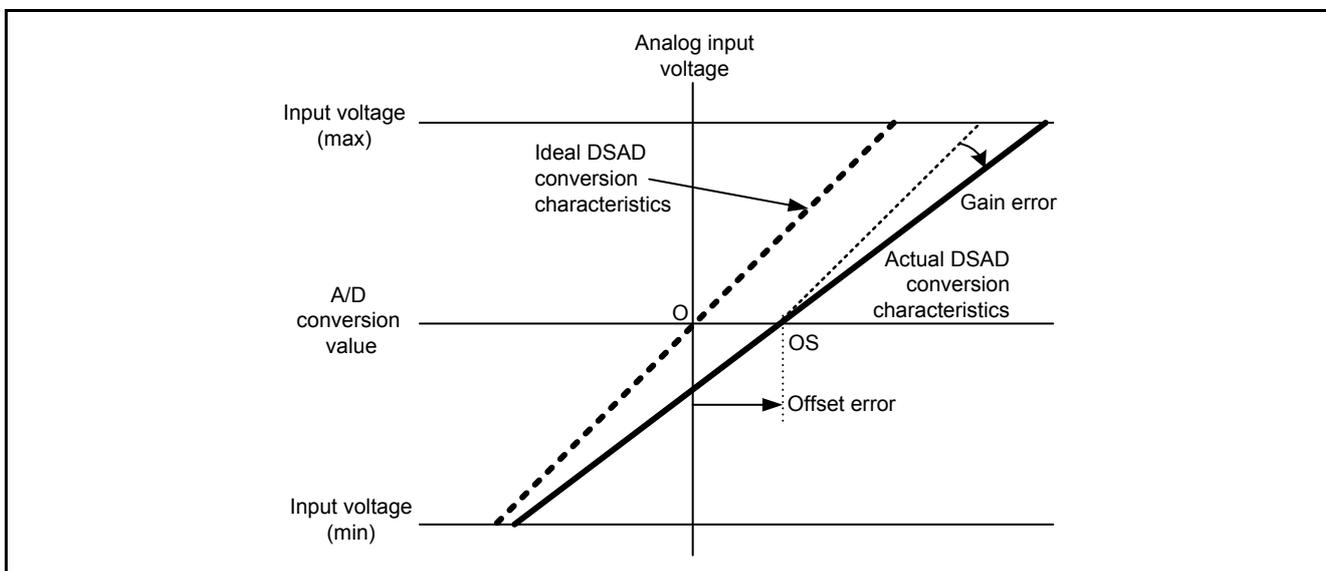
Figure 5.1 Example of the DSAD I/O Characteristics
