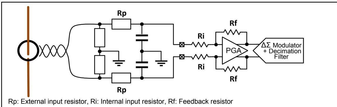
**Figure 6.2 Connection Diagram of the Differential Input Channel**
