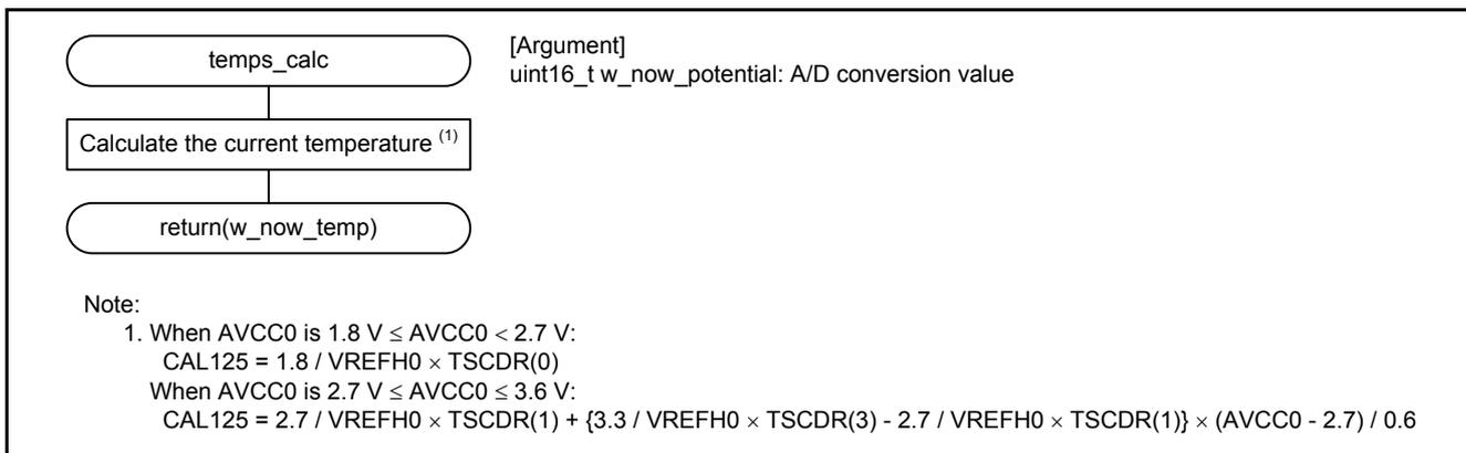
Figure 9.24 Current Temperature Calculation
