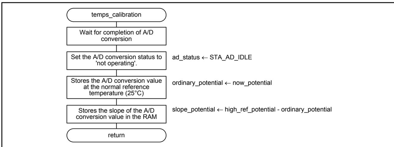
Figure 9.22 Temperature Sensor Calibration Processing
