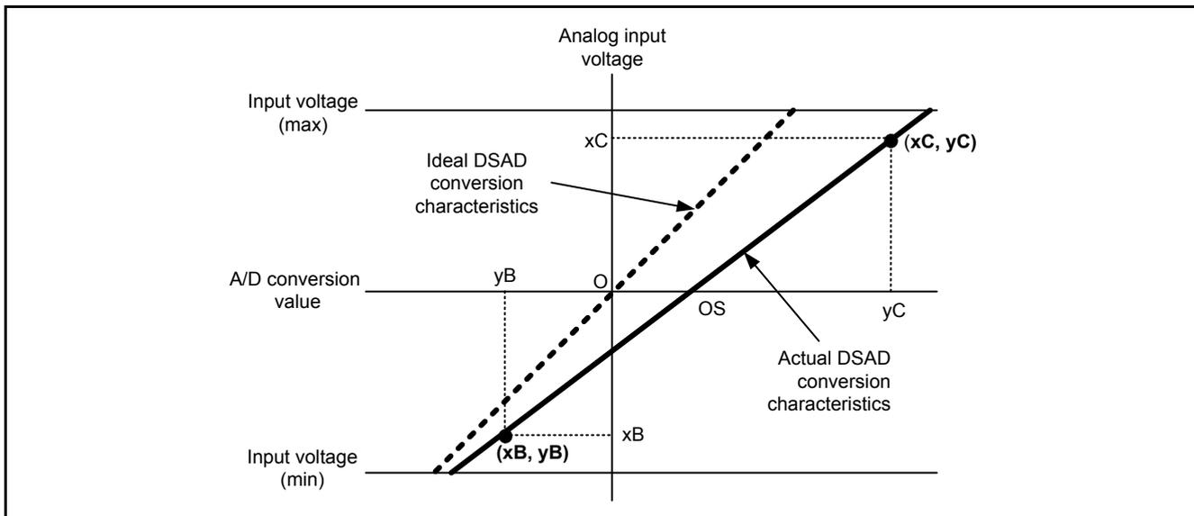
Figure 5.2 Method to Calculate the Calibration Values for Gain and Offset with DC Power Supply
