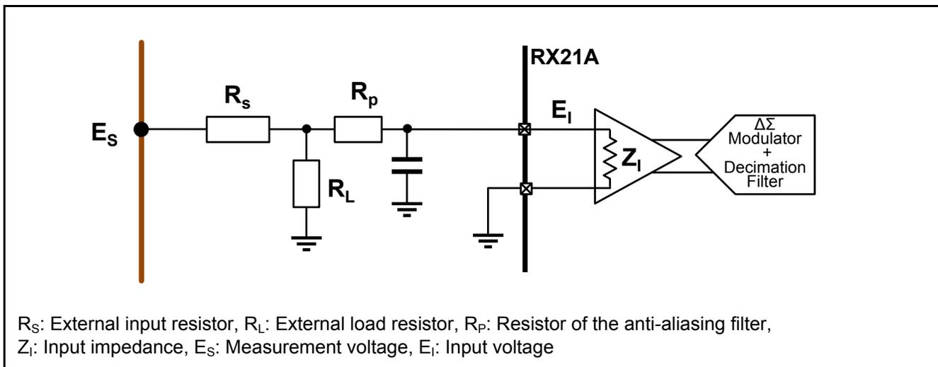
**Figure 7.5 Connection Example of Single-Ended Input**
