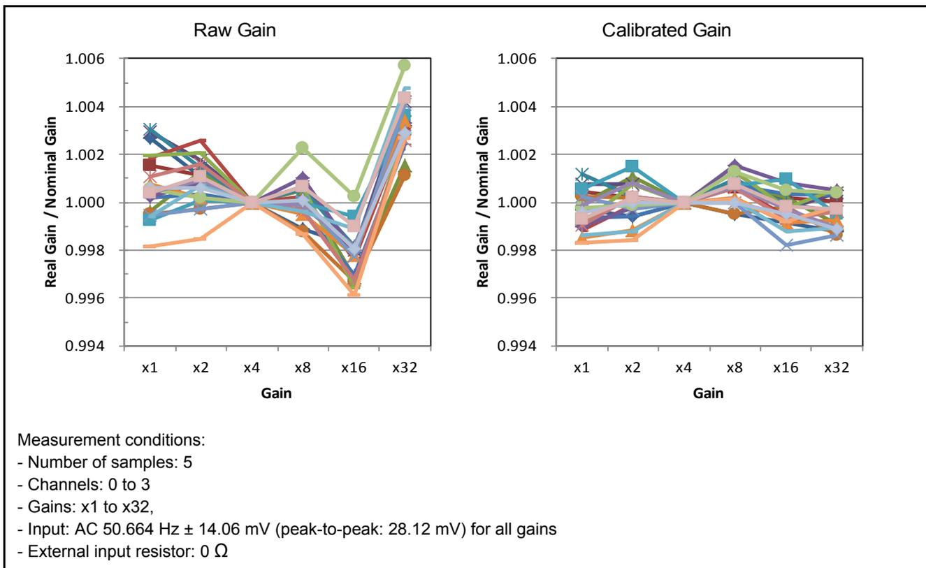
Figure 10.1 Result of the System Gain Calibration
