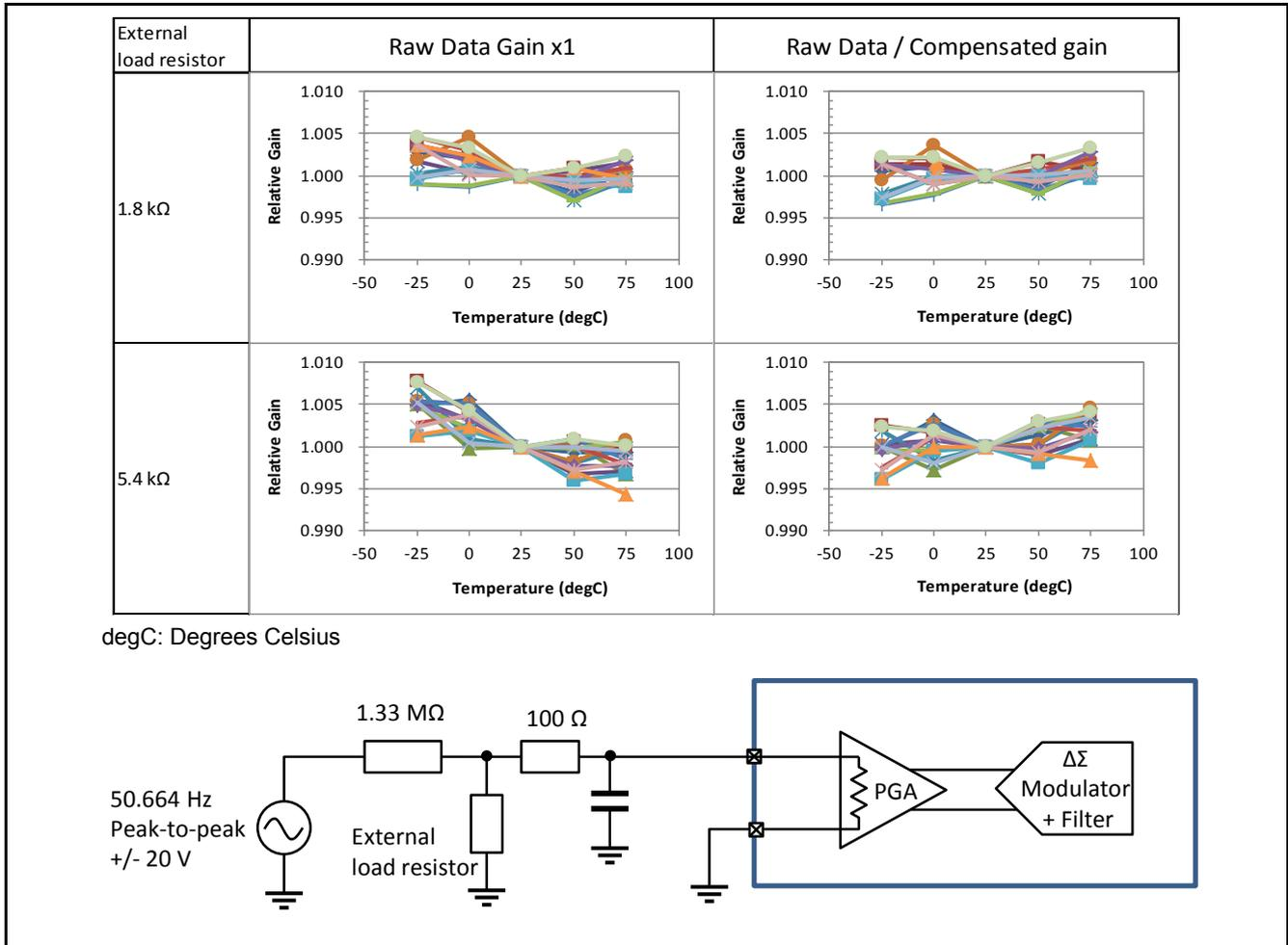
Figure 10.4 System Gain of the Single-Ended Input Pins
