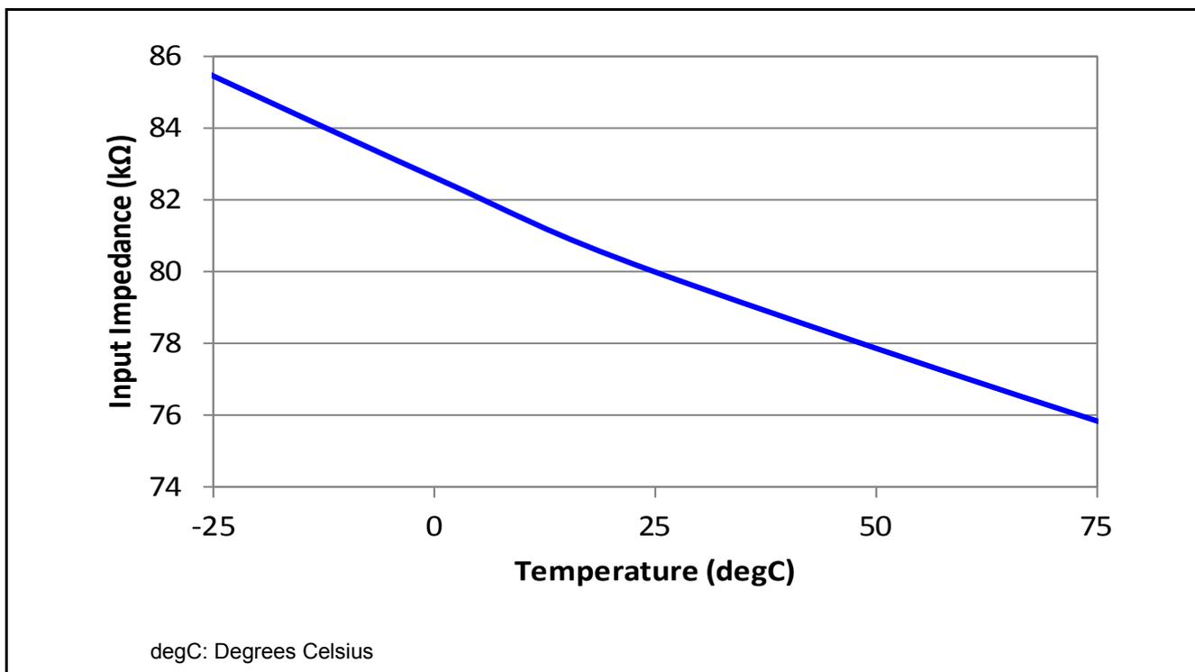
**Figure 7.4 Temperature Characteristics of the Input Impedance for The Single-Ended Input at Gain x1**
