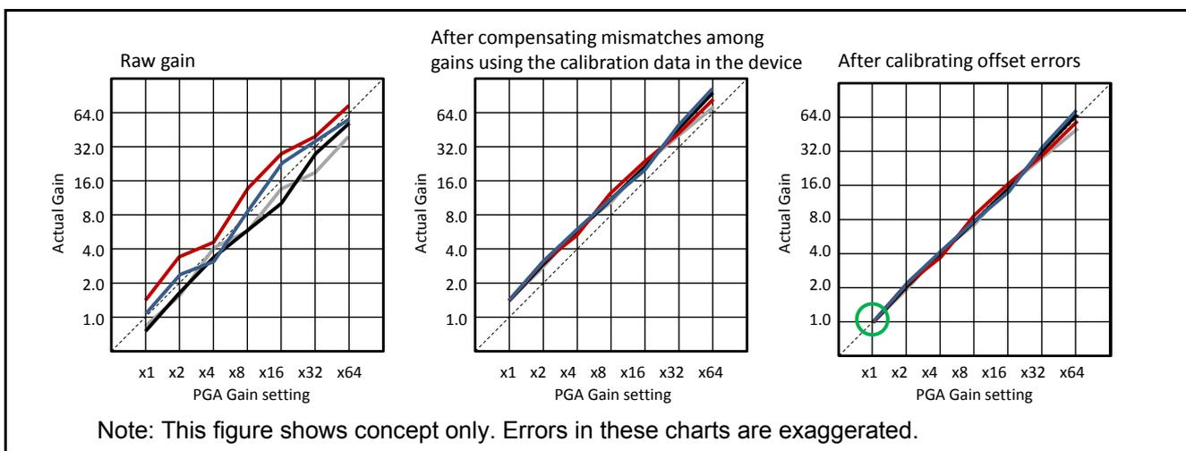
Figure 6.1 Gain Calibration
