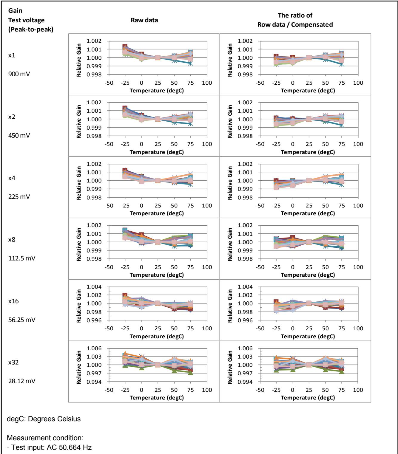
Figure 10.3 System Gain of the Differential Input Pins
