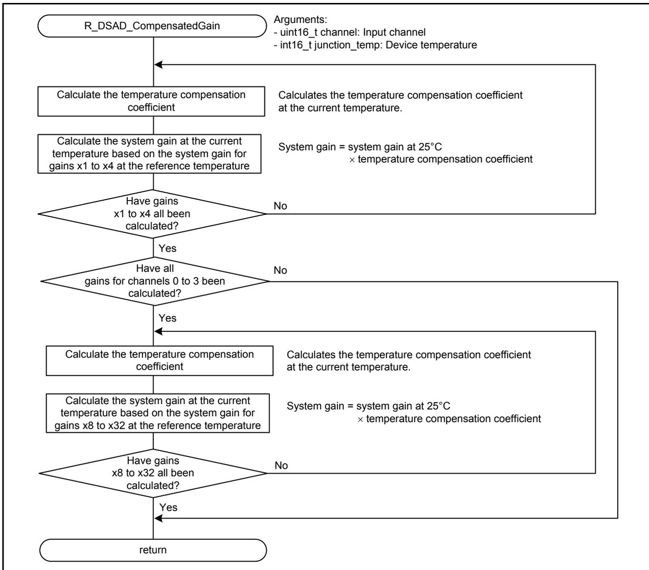
Figure 9.13 Temperature Compensation for the System Gain
