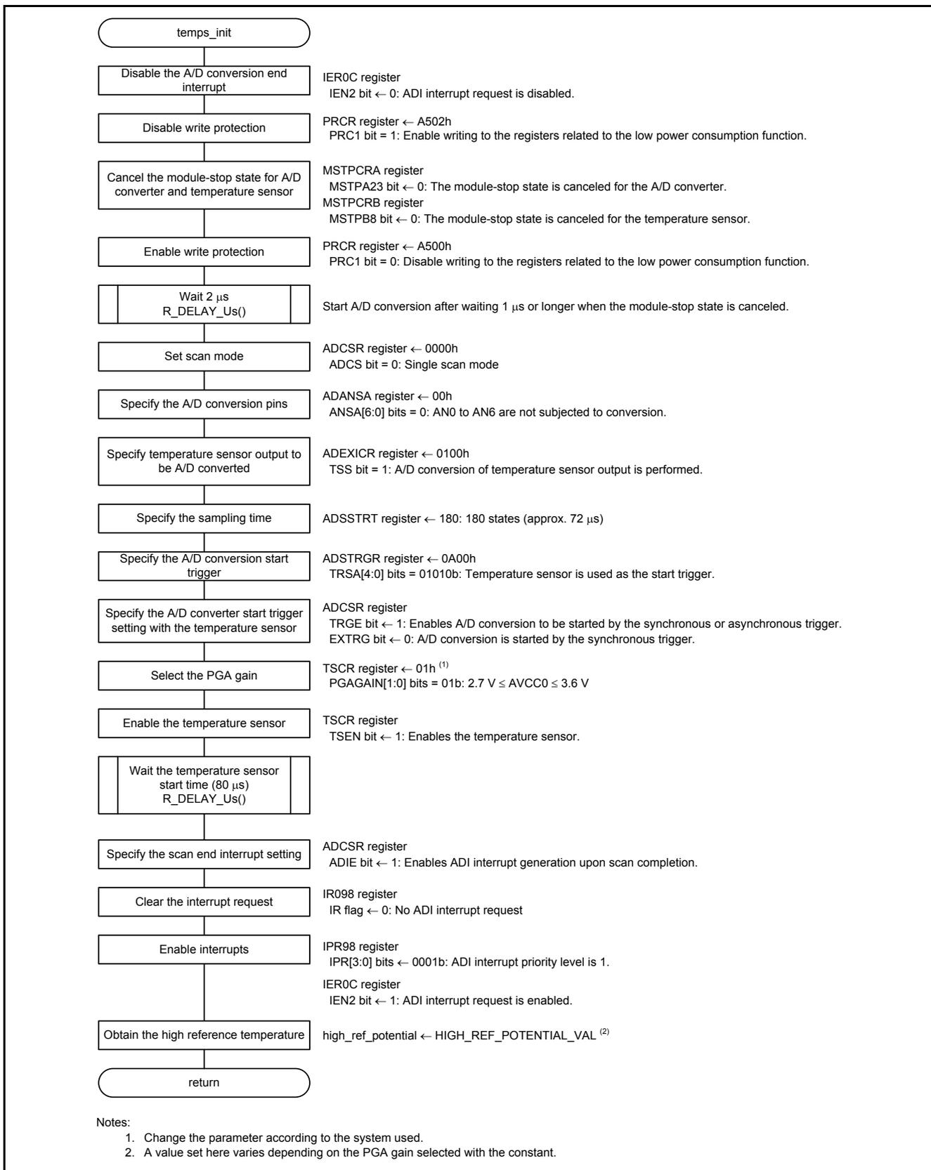
Figure 9.17 A/D Converter and Temperature Sensor Initializations
