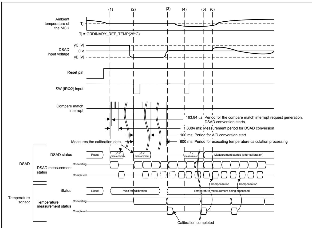
Figure 9.1 Operation Timing Diagram
