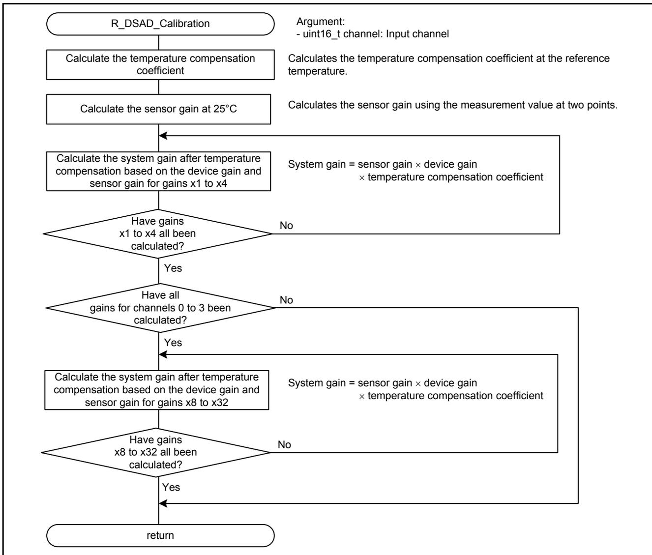
Figure 9.12 System Gain Calibration
