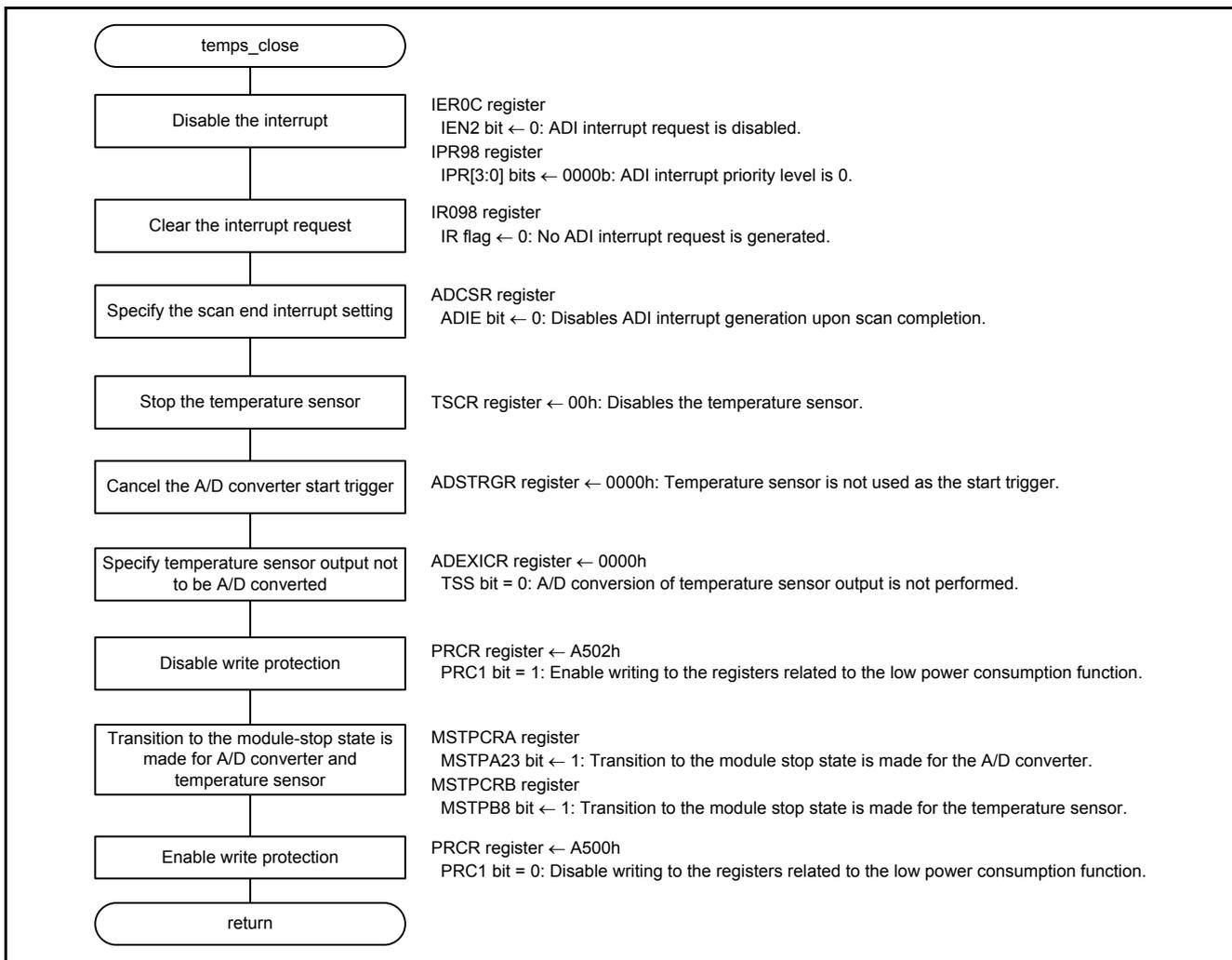
Figure 9.18 A/D Converter and Temperature Sensor Stop Processing
