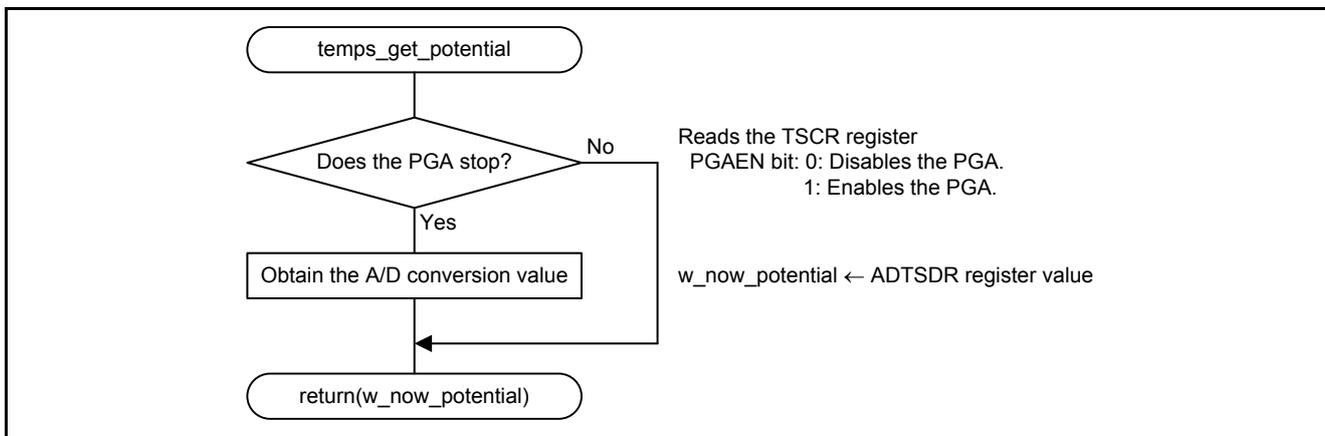
Figure 9.20 Obtaining Temperature Sensor Measurement Result
