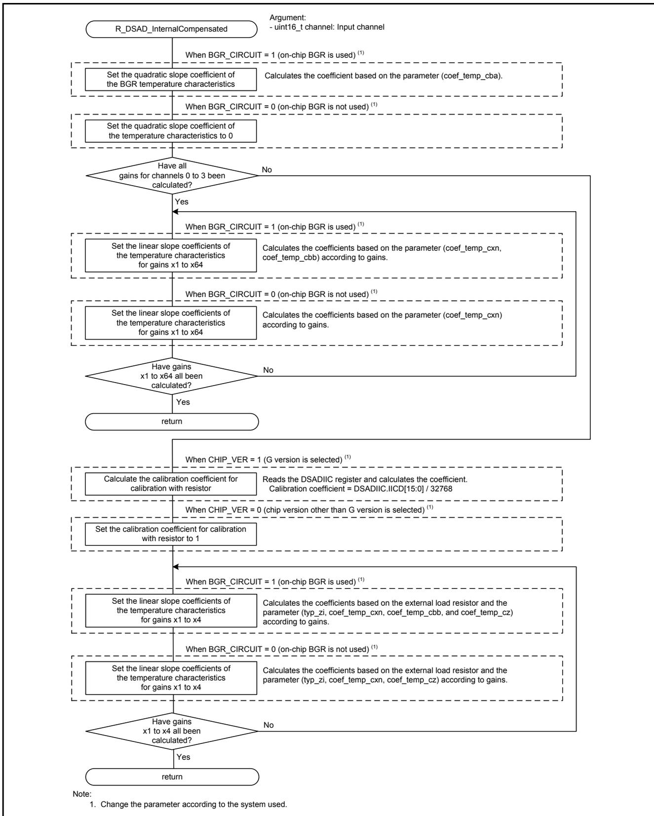
Figure 9.11 Coefficient Initialization for Gain Temperature Compensation
