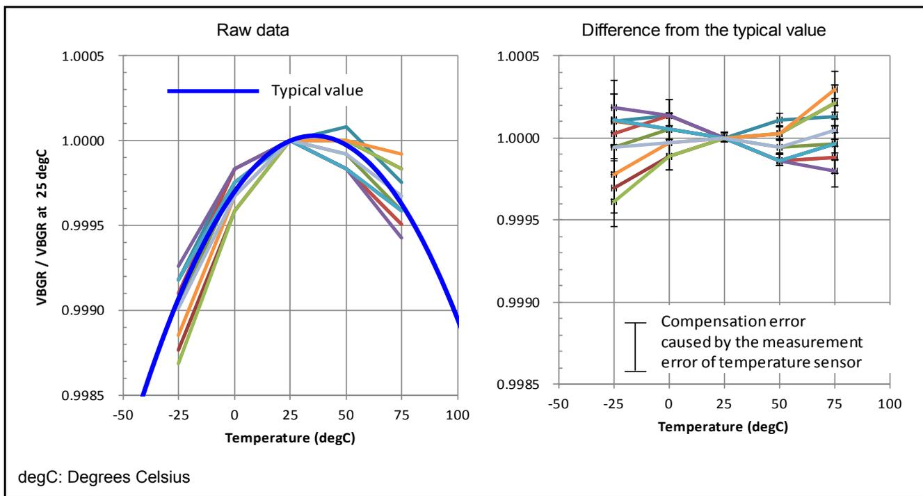
**Figure 10.2 Temperature Characteristics of the VBGR (Difference Between the Measured Values and Typical Values)**
