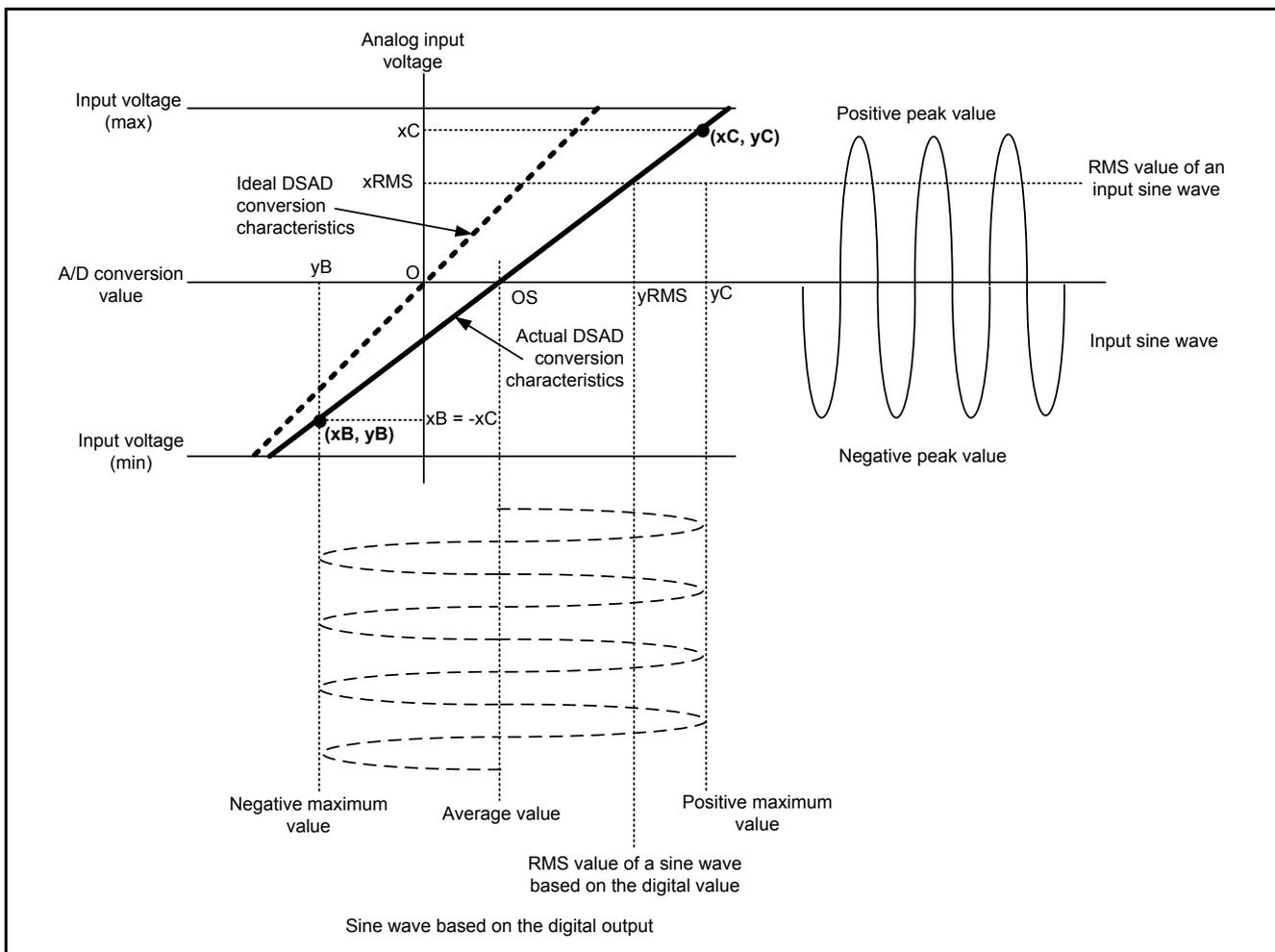
Figure 5.3 Method to Calculate the Calibration Values for Gain and Offset with Sine Wave AC Power Supply
