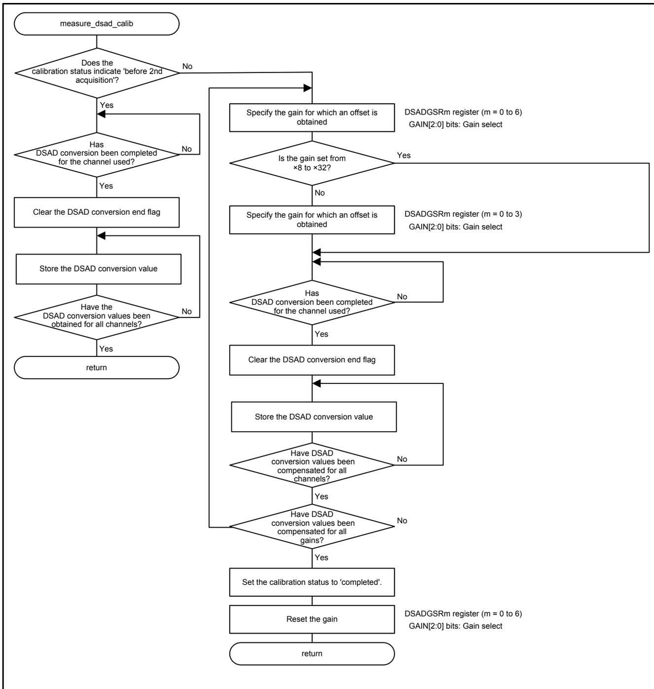
Figure 9.14 Obtaining DSAD Conversion Result at Calibration
