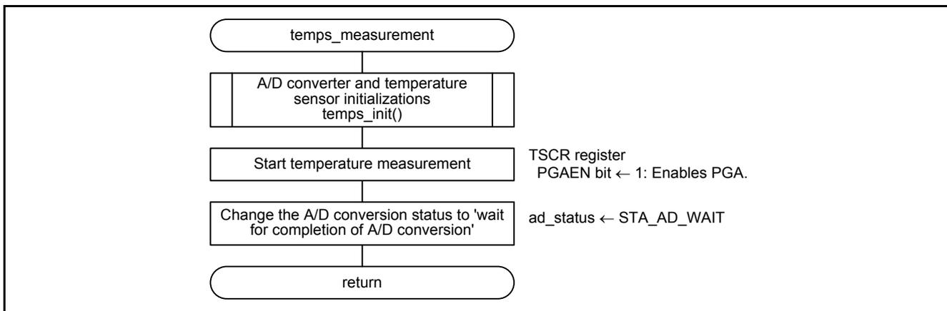
Figure 9.23 Temperature Sensor Measurement Processing
