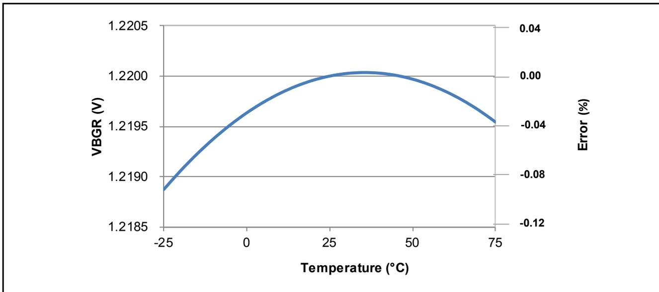
Figure 7.3 Temperature Characteristics of the VBGR
