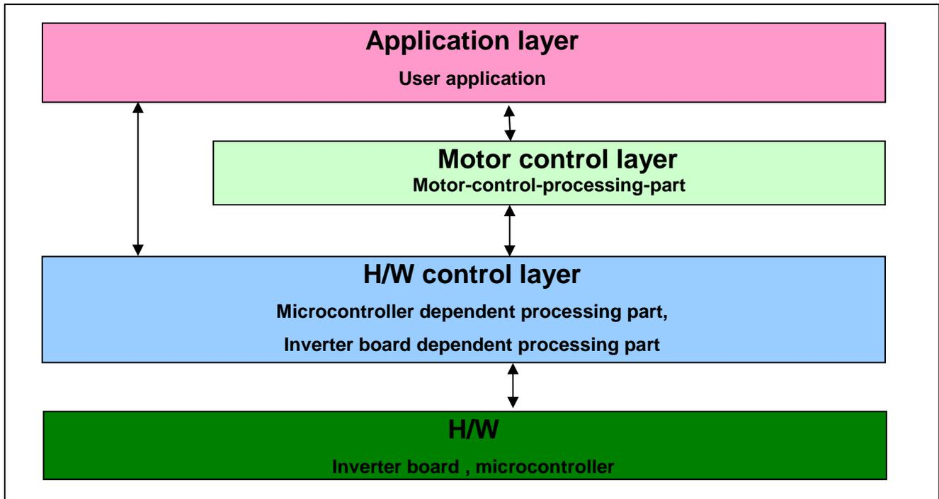
Figure 2-2 Module Configuration of the Sample Programs
