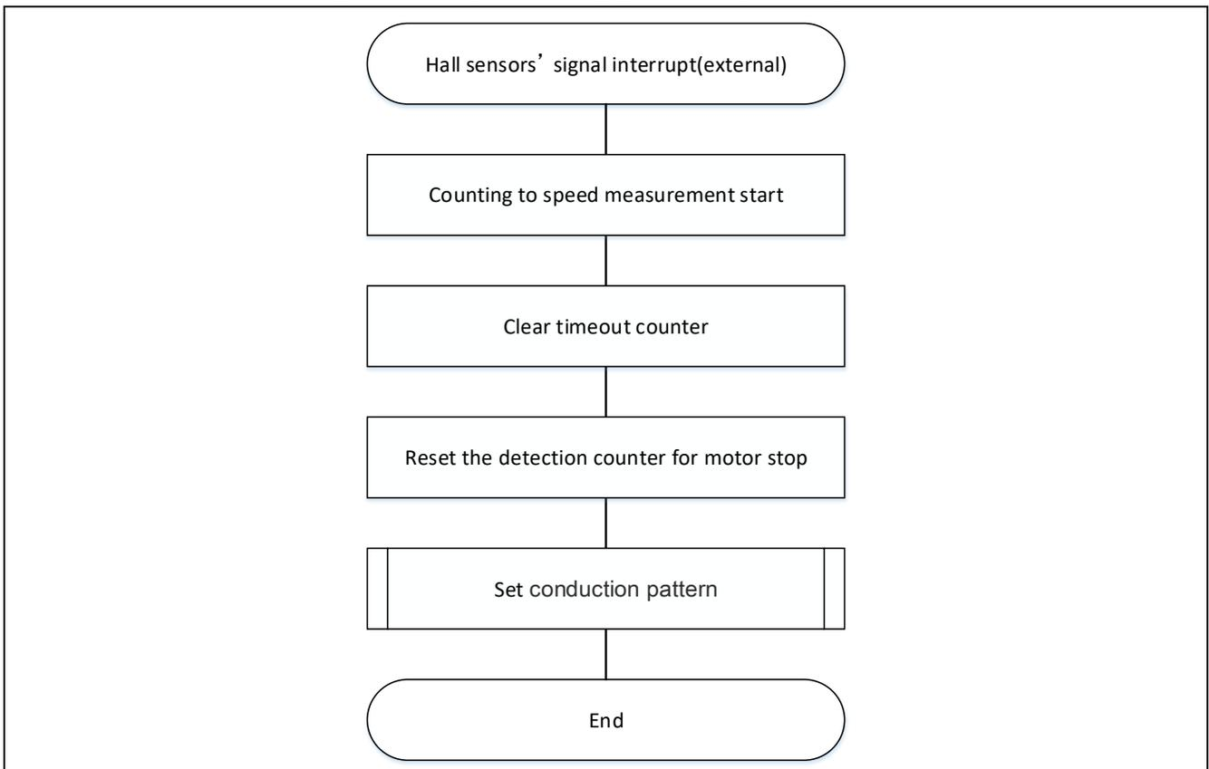
Figure 3-11 Hall sensors' signal Interrupt Handling (common process)
