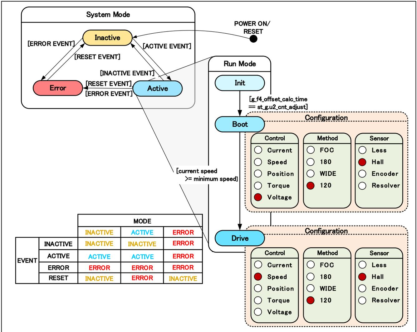
Figure 3-5 State Transition Diagram of 120-degree Conducting Control using hall sensors Software
