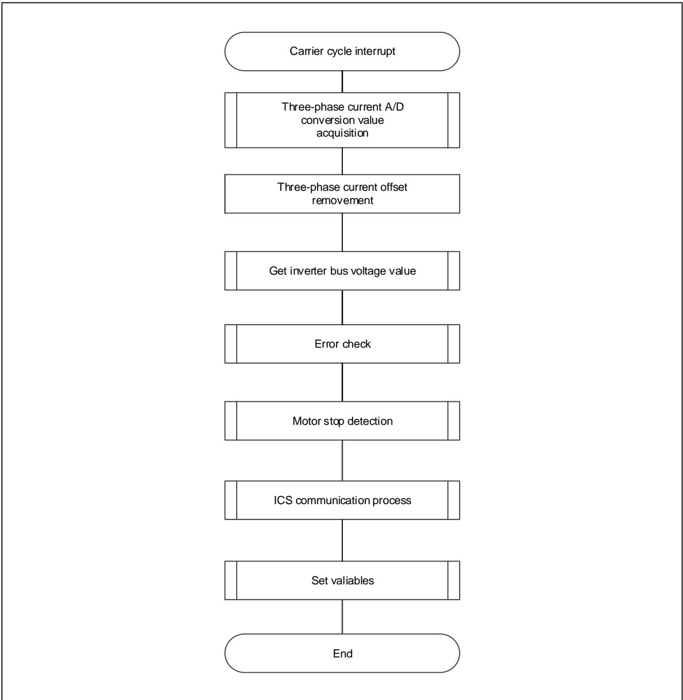
Figure 3-8 Carrier Cycle Interrupt Handling (120-degree Control using hall sensors)
