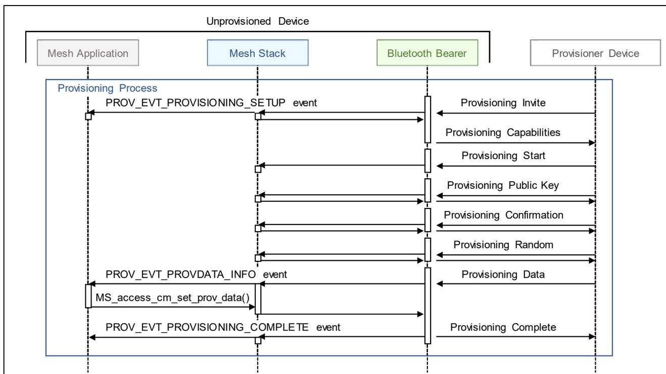
**Figure 3-5 Provisioning Process**
