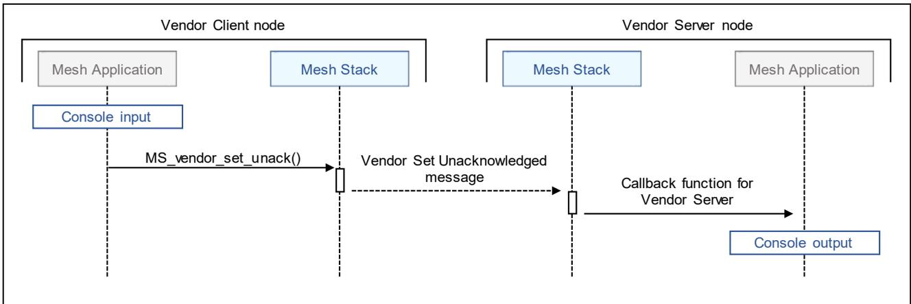
Figure 3-17 Vendor Model Operation of Mesh Sample Program
