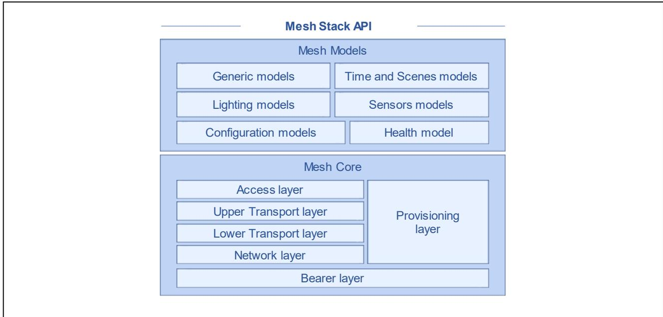
**Figure 2-3 Internal Architecture of Bluetooth Mesh Stack**
