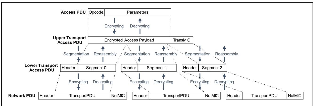
**Figure 1-4 Segmentation and Reassembly of Access PDU**
