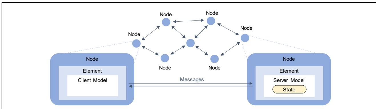
**Figure 1-1 Basic Composition of Bluetooth Mesh Network**
