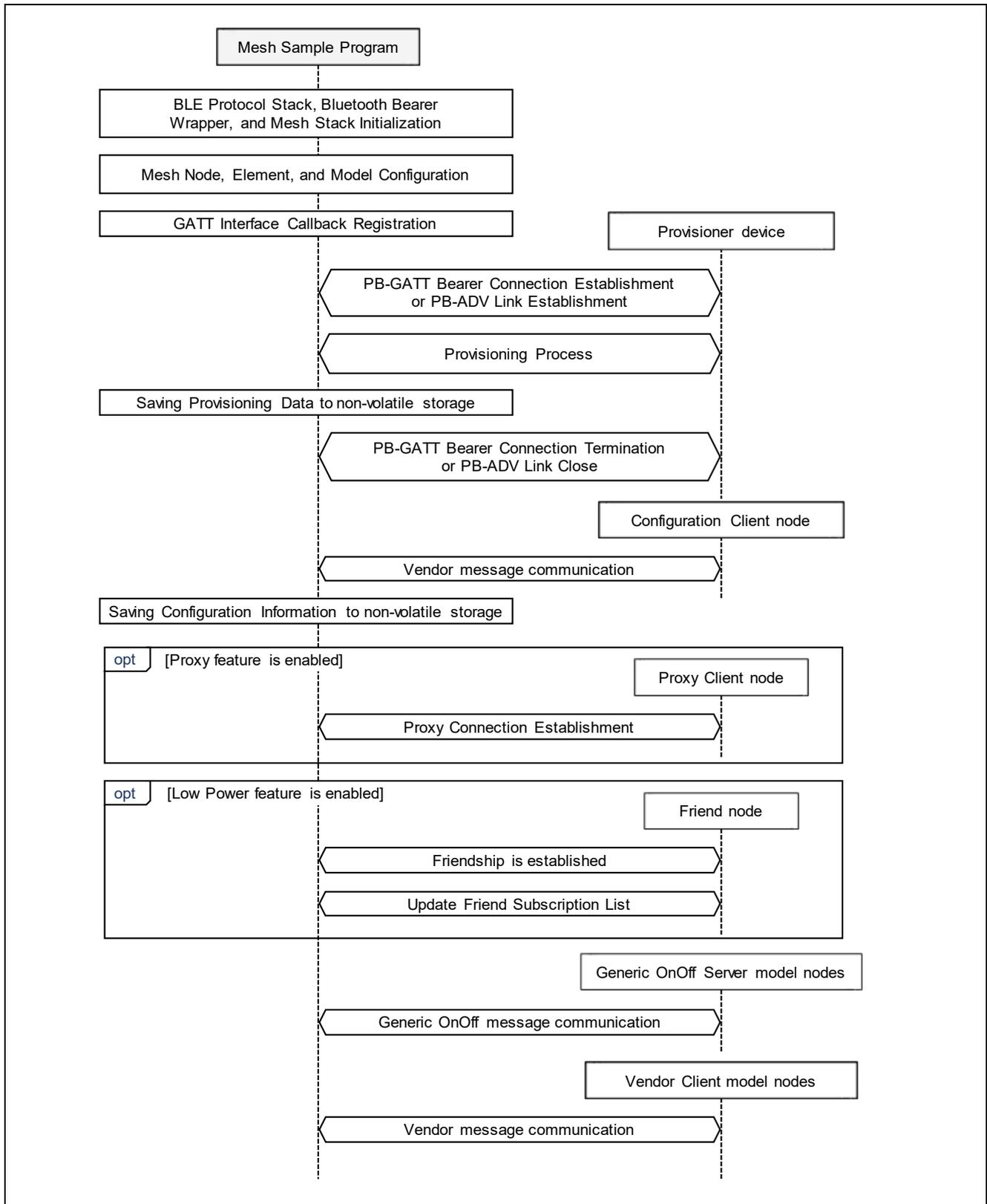
Figure 3-1 Sequence Chart of Mesh Sample Program
