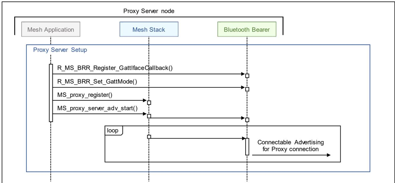
Figure 3-7 Proxy Setup
