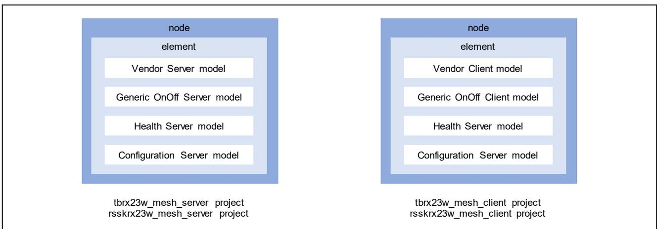
Figure 2-2 Model Composition of Mesh Sample Program
