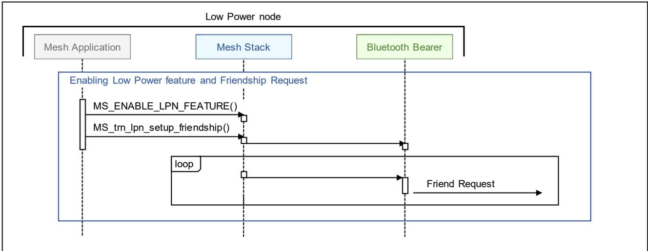
Figure 3-9 Enabling Low Power Feature and Friendship Request
