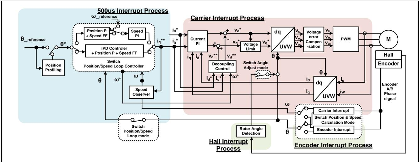
Figure 3-8 System Block of Vector Control with Encoder
