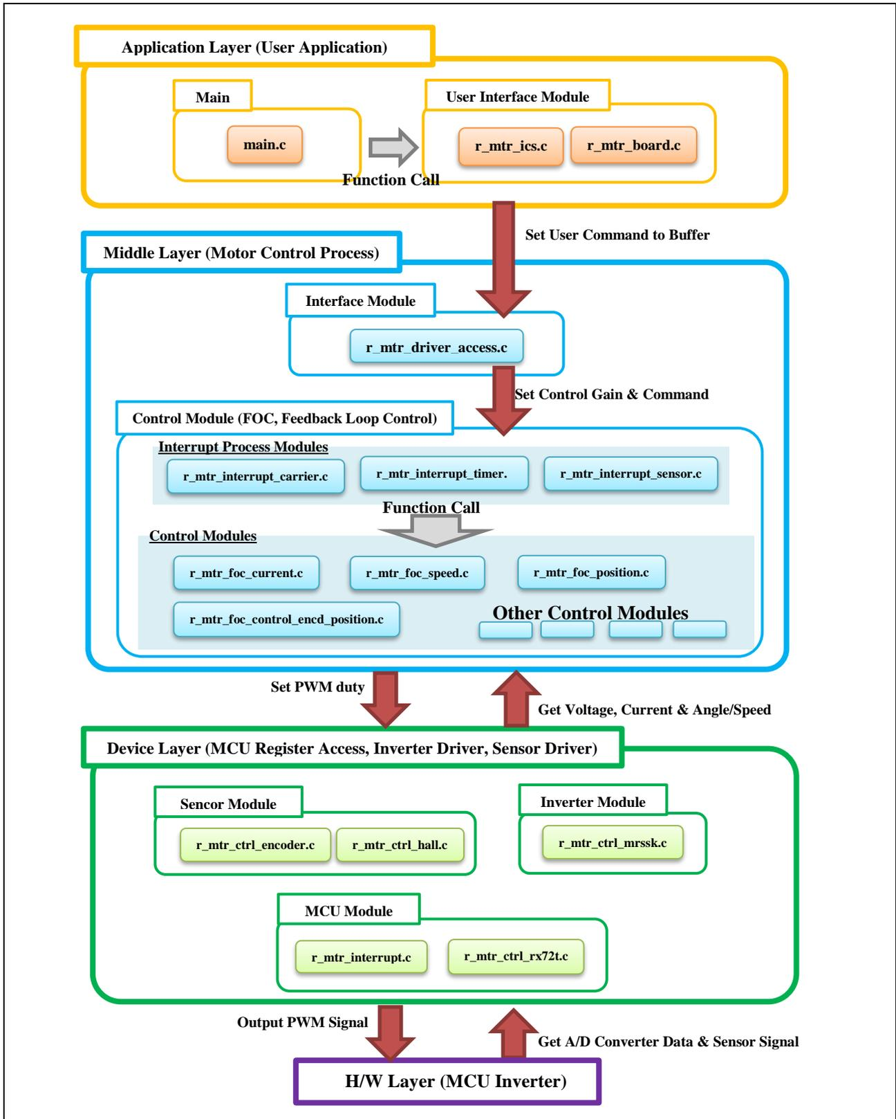
Figure 2-3 Module Configuration
