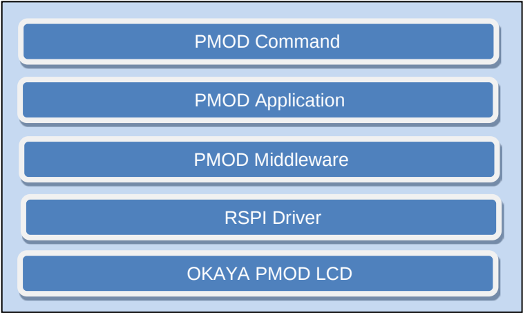
Figure 4-5 PMOD Hierarchical Software Layer
