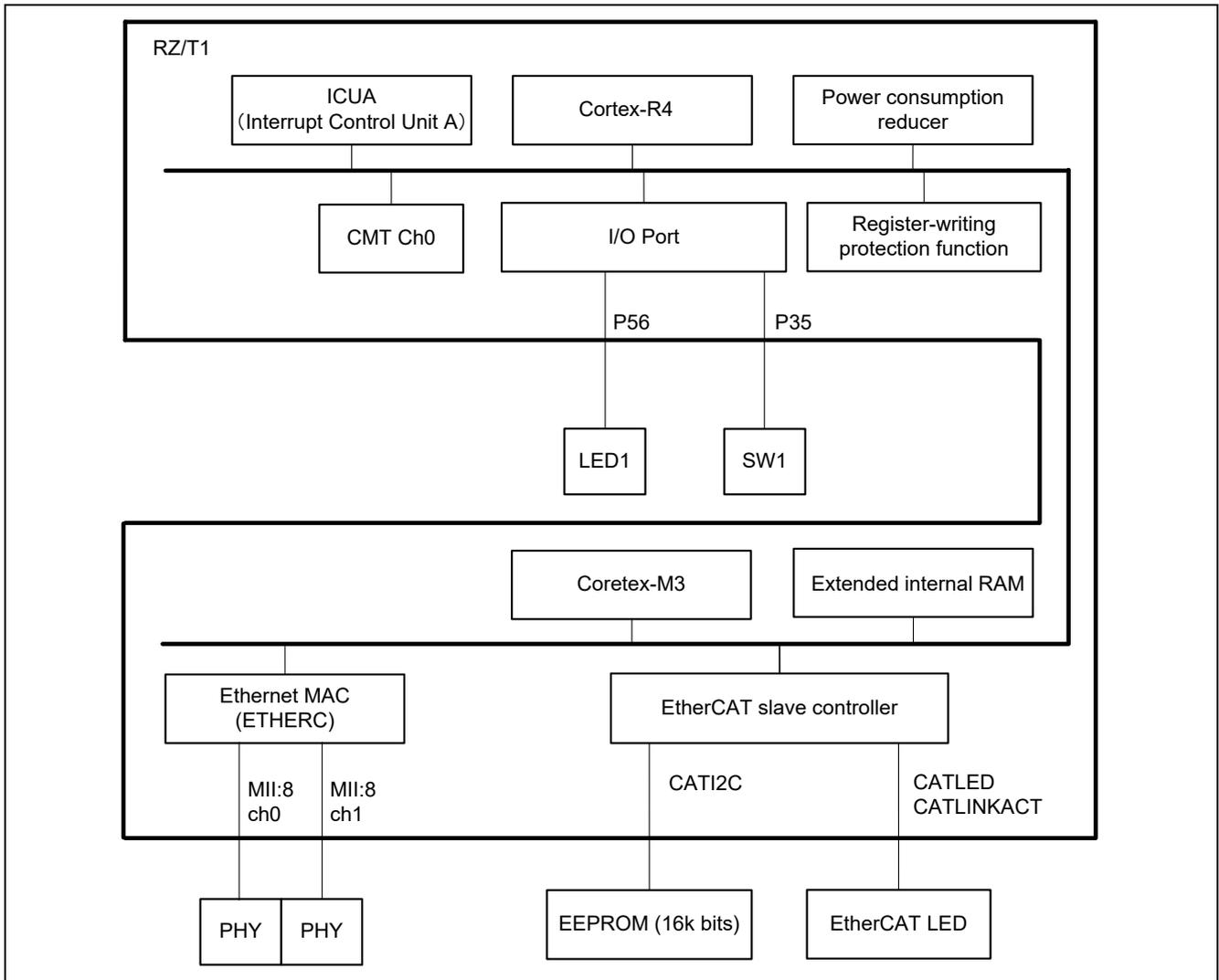
Figure 4.2 Example of the Hardware Structure for the CiA402 Sample Program
