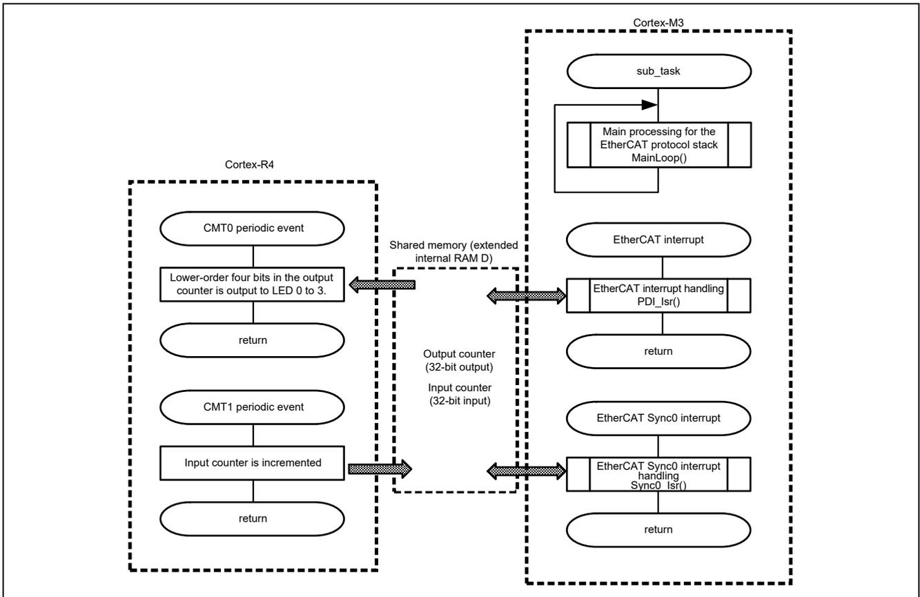
Figure 5.3 Simple Flowchart of the I/O Controller Sample Program (2)
