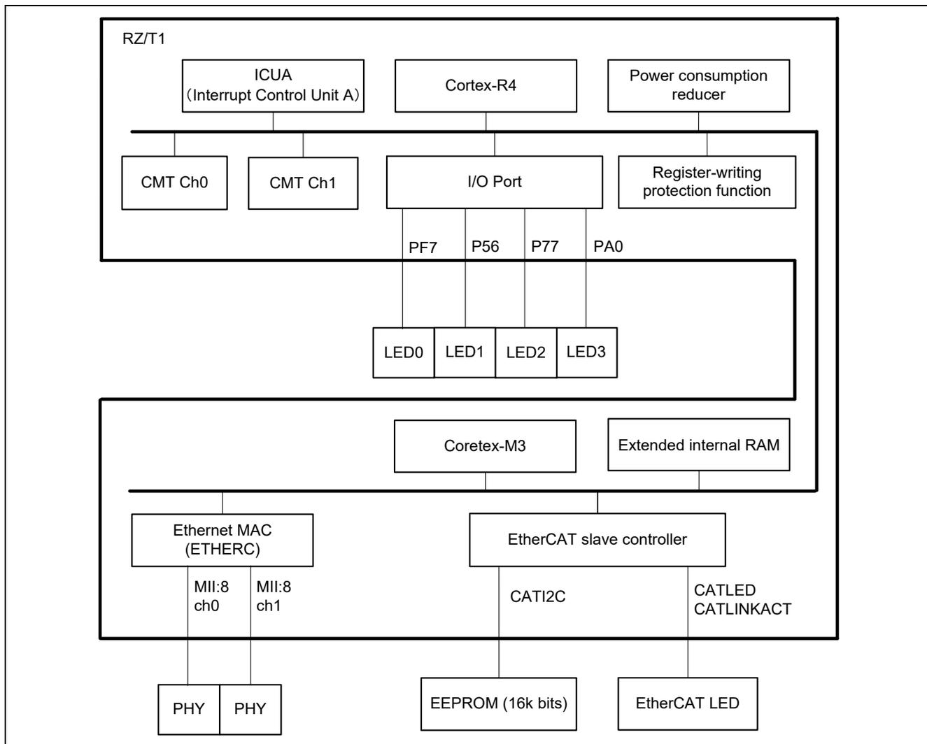
Figure 4.1 Example of the Hardware Structure for the I/O Controller Sample Program
