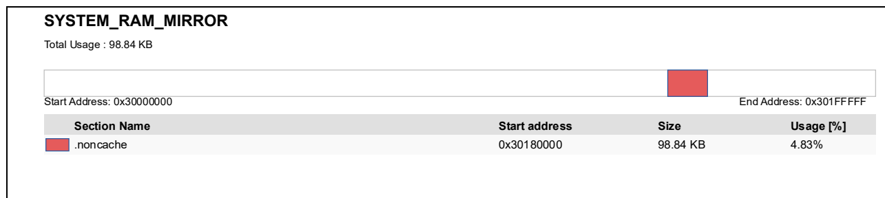
Figure 8.16. SYSTEM_RAM_MIRROR footprint of the RZ/T2M Secondary project (e 2 studio)
