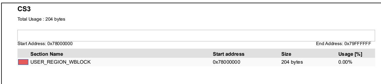
Figure 8.23. CS3 (SDRAM) footprint of the RZ/T2M Primary project (EWARM)
