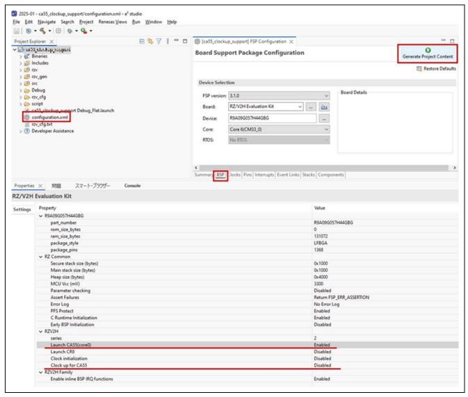
Figure 5-5. CM33 project setting for CM33 cold boot
