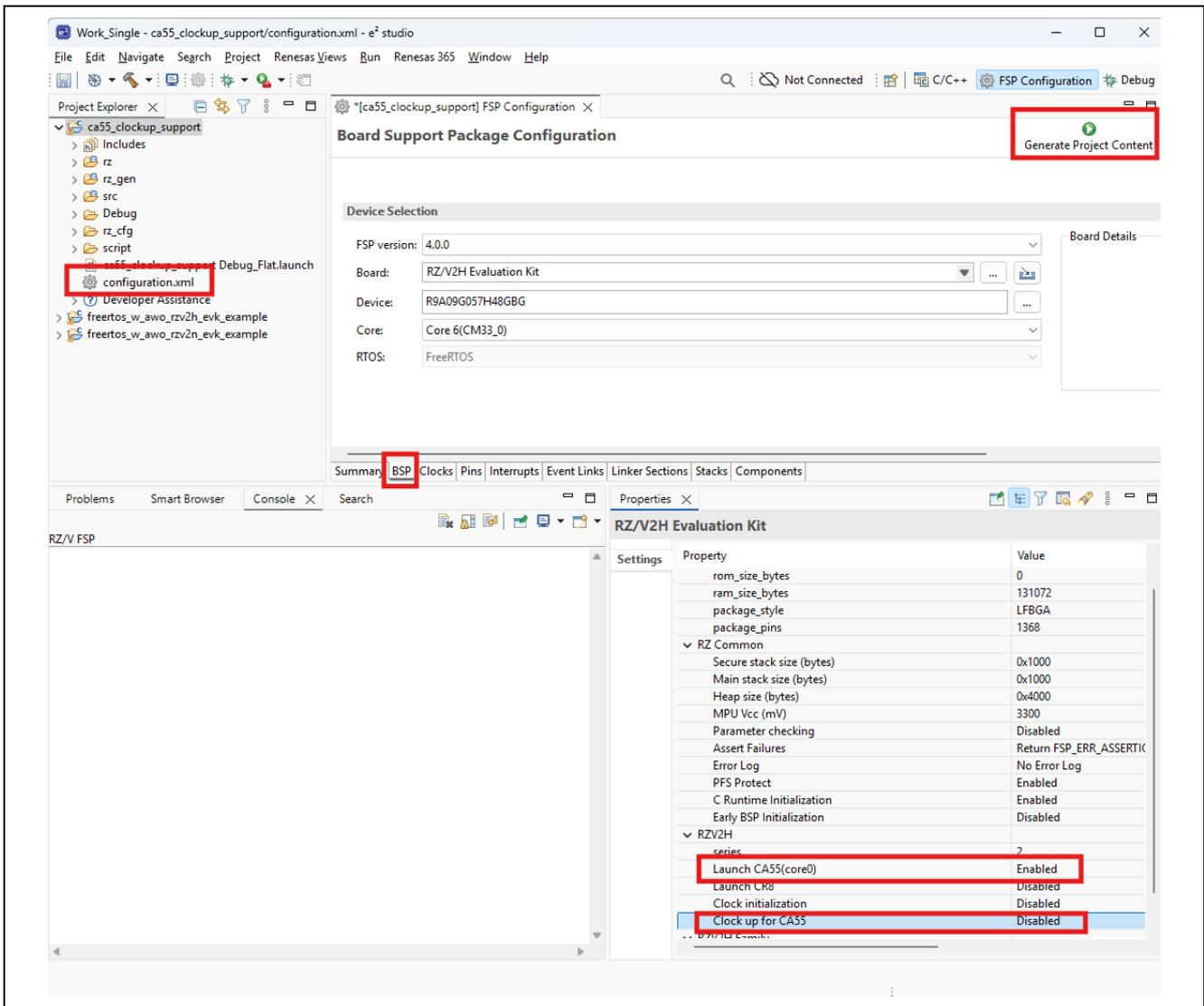
Figure 4-5. CM33 project setting for CM33 cold boot
