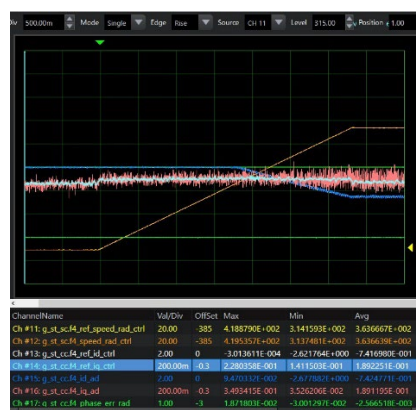
Figure 12-7 Example of Waveforms during Operation under Flux Weakening Control
