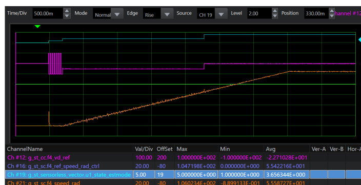
Figure 12-3 Waveforms Indicating the Characteristics during Start-up under Sensorless Control
