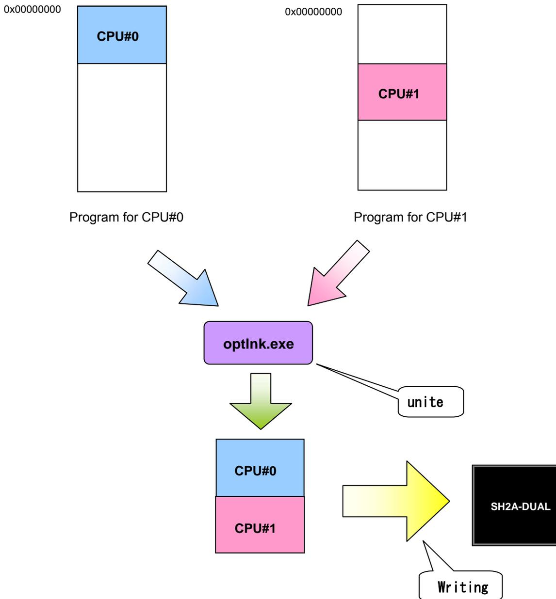
fig.1-1 Example of constructing object for SH2A-DUAL
