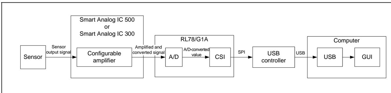
**Figure 2-2      Function Block When Using SPI Communication**
