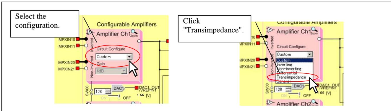
Figure 3-15 Specifying the Amplifier Configuration
