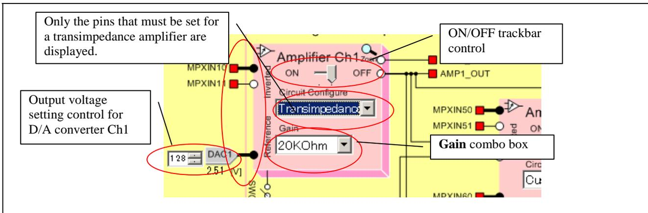
Figure 3-9 Screen After Transimpedance Amplifier Is Selected
