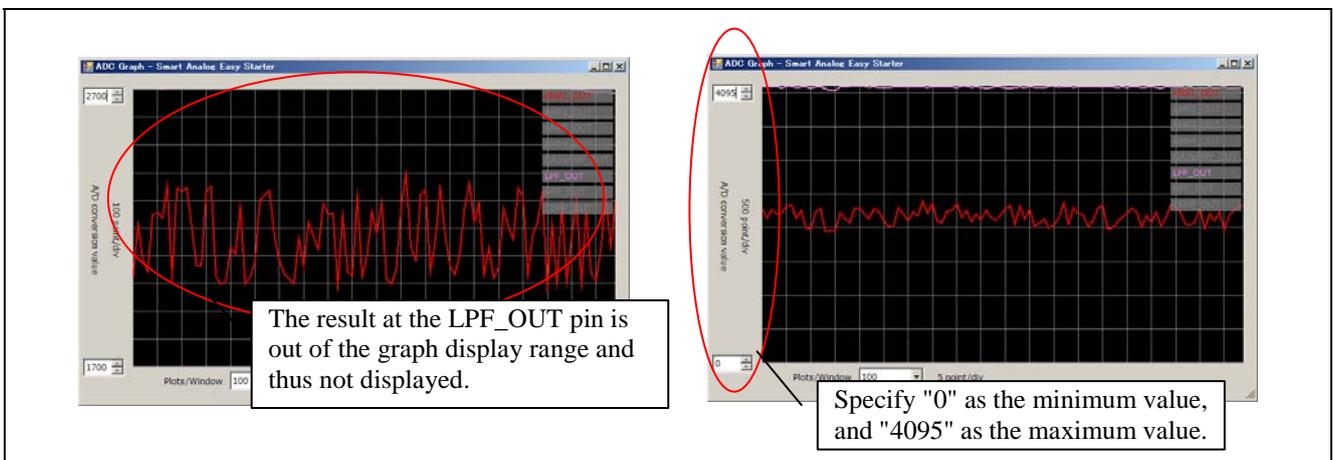
**Figure 3-41 Checking the LPF Output Waveform**
