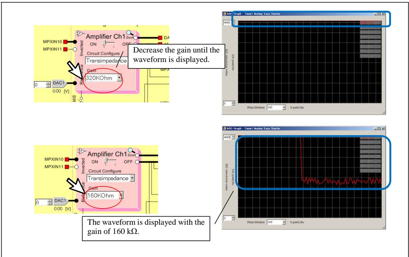
Figure 3-29 Setting the Gain
