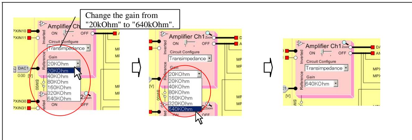
Figure 3-27 Setting the Gain
