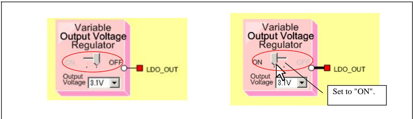
**Figure 3-21 Setting the Variable Output Voltage Regulator**
