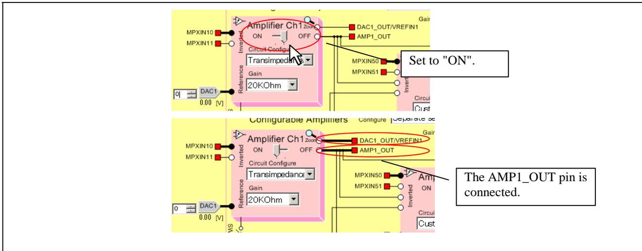
Figure 3-12 Enabling Operation of the Configurable Amplifier
