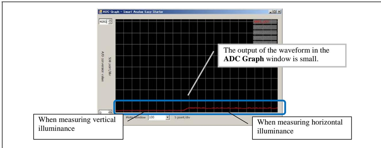
Figure 3-26 Displaying the Output Signal Waveforms
