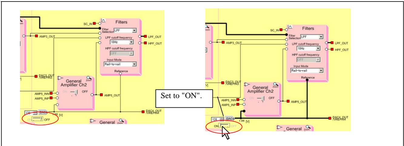
**Figure 3-39 Supplying the Reference Voltage to the Filter**
