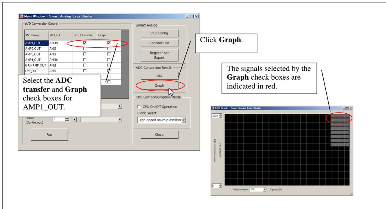
Figure 3-22 Specifying the Output Signal
