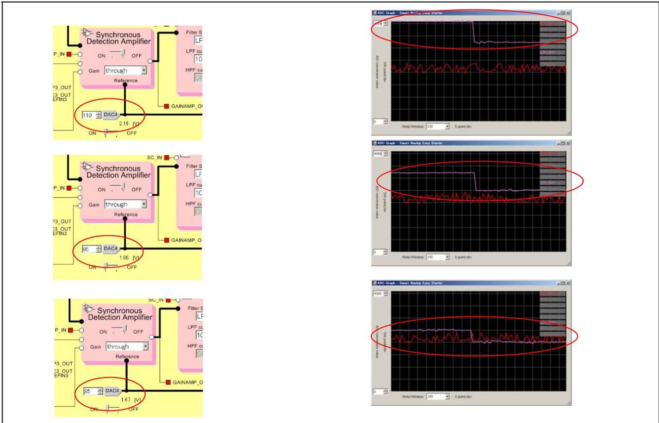
**Figure 3-35 Adjusting the Voltage Level at D/A Converter**
