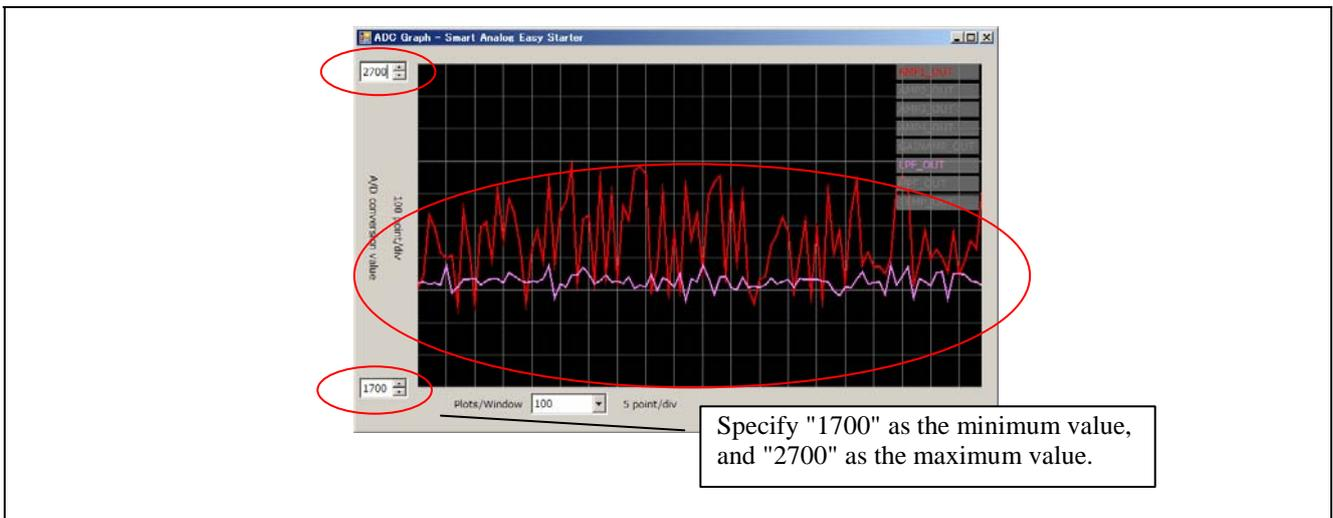
**Figure 3-43 Checking LPF\_OUT**
