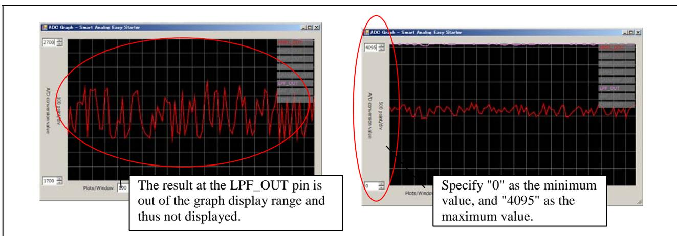
**Figure 3-34 Checking the LPF Output Waveform**
