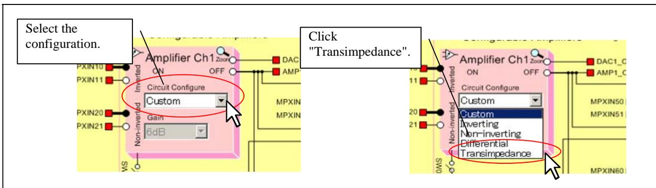
Figure 3-8 Specifying the Amplifier Configuration
