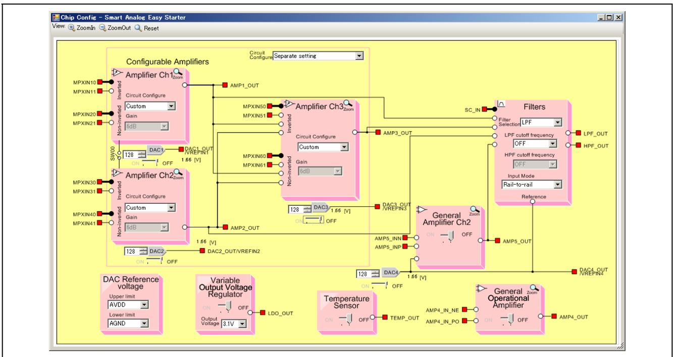
Figure 3-7 Chip Config Window When Using Smart Analog IC 300
