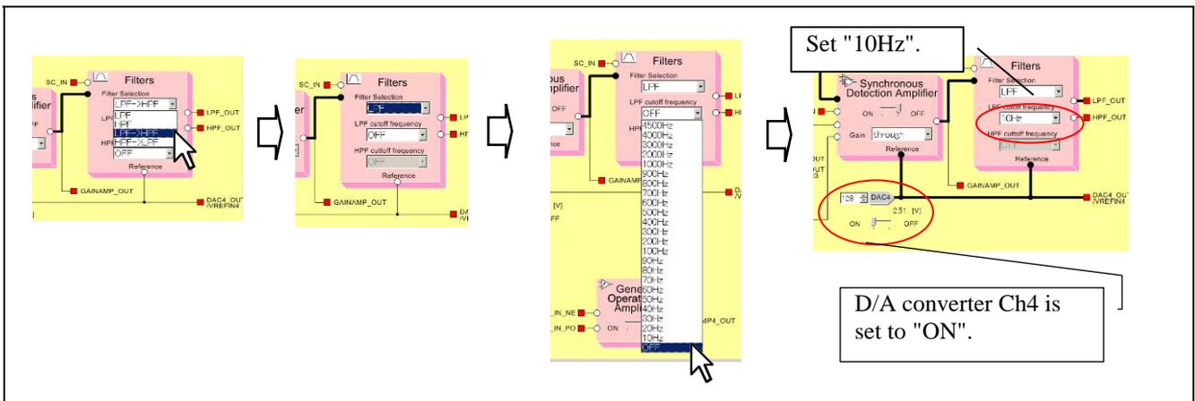
Figure 3-32 Selecting the Filter and Specifying the Cutoff Frequency
