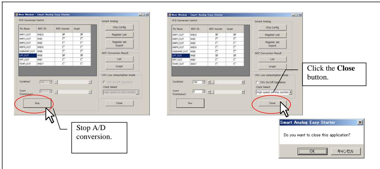
Figure 3-44 Terminating Easy Starter and Saving the Settings
