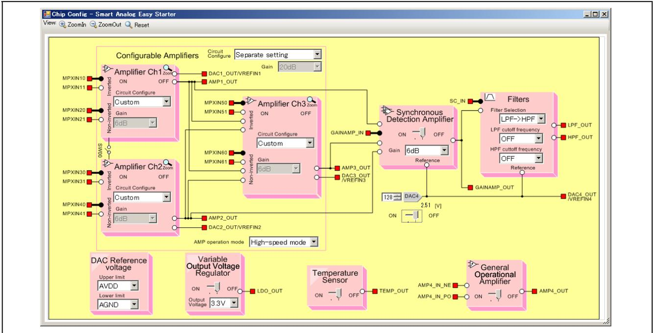
Figure 3-6 Chip Config Window When Using Smart Analog IC 500
