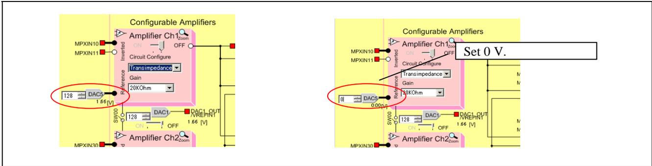
**Figure 3-17 Specifying the Configurable Amplifier Reference Voltage**
