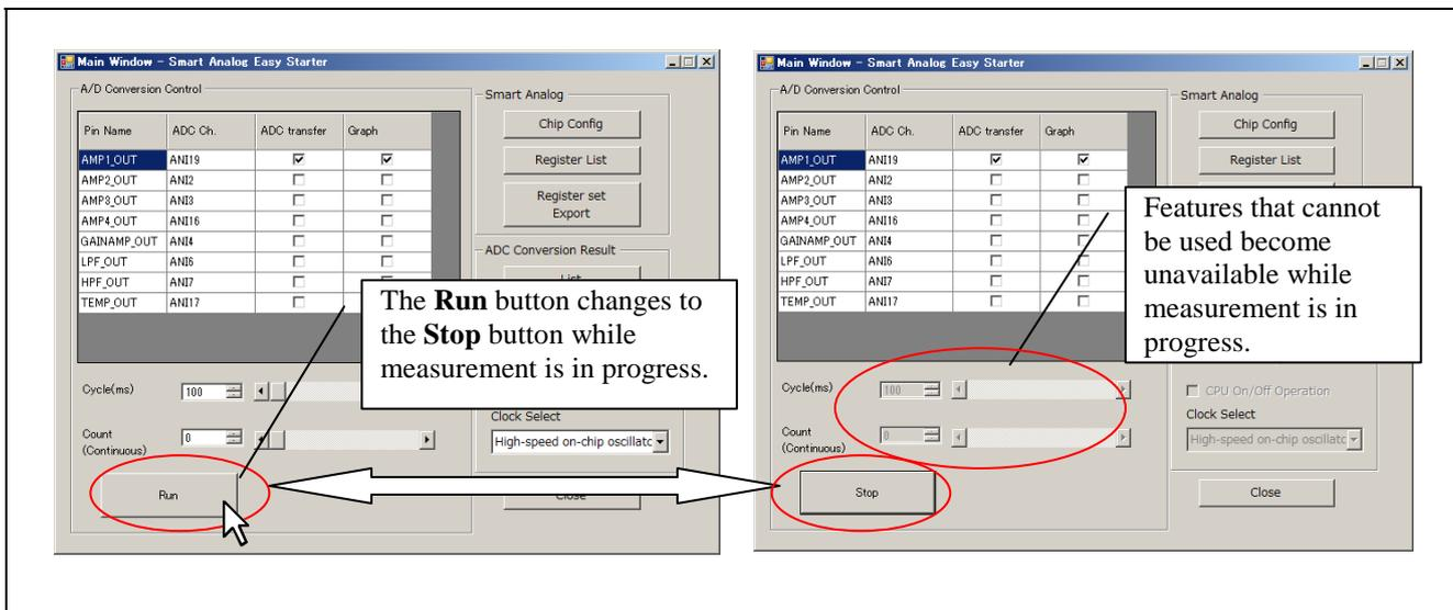
**Figure 3-24 Measuring the Output Signal**
