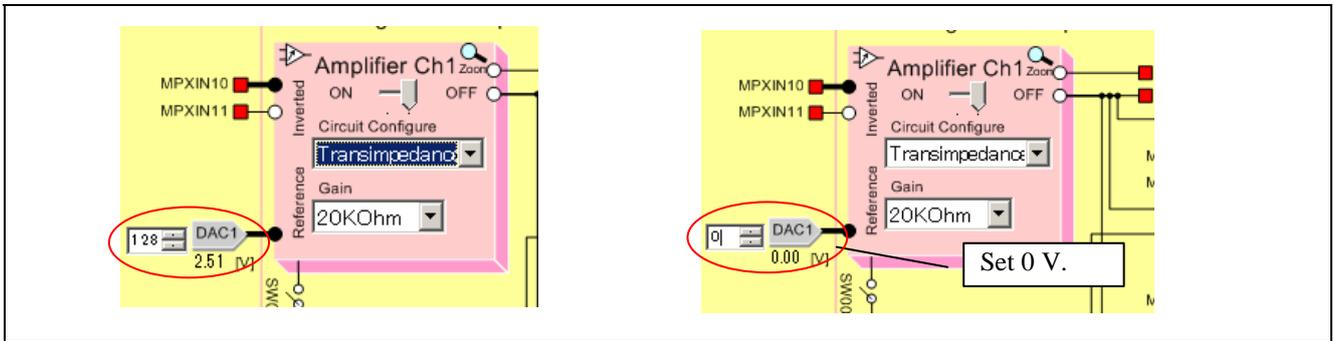
Figure 3-10 Specifying the Configurable Amplifier Reference Voltage
