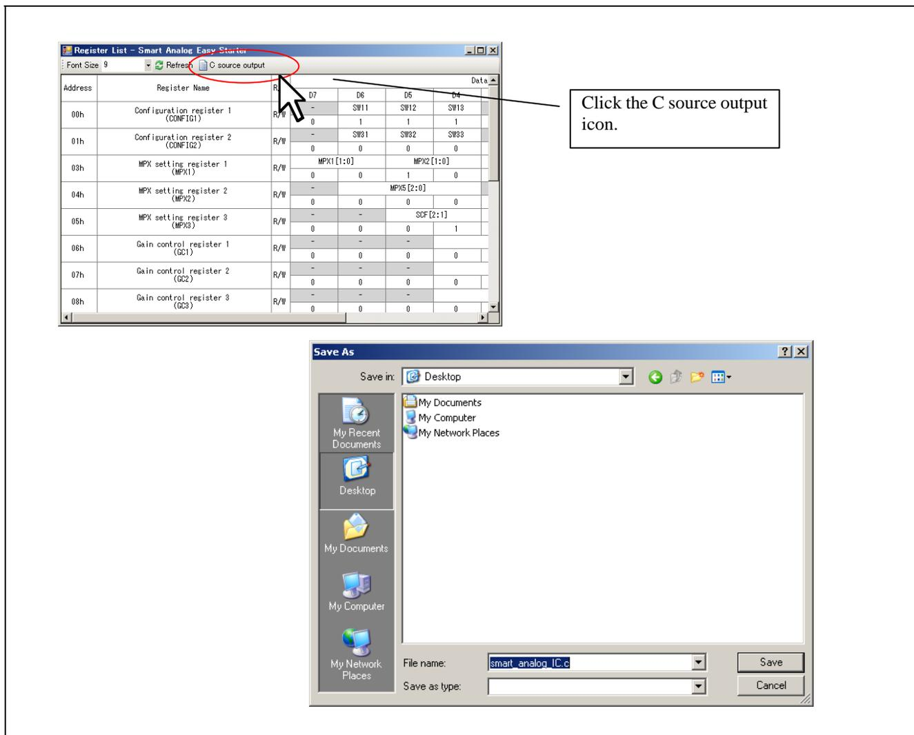
**Figure 3-53    Outputting the C Source**
