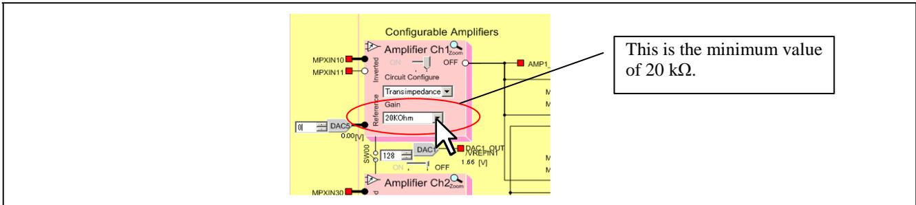
**Figure 3-18 Specifying the Configurable Amplifier Gain**
