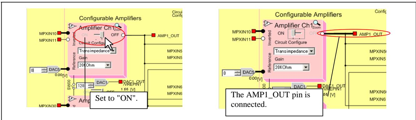
**Figure 3-19 Enabling Operation of the Configurable Amplifier**
