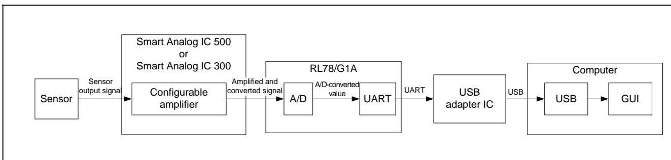
**Figure 2-3      Function Block When Using UART Communication**
