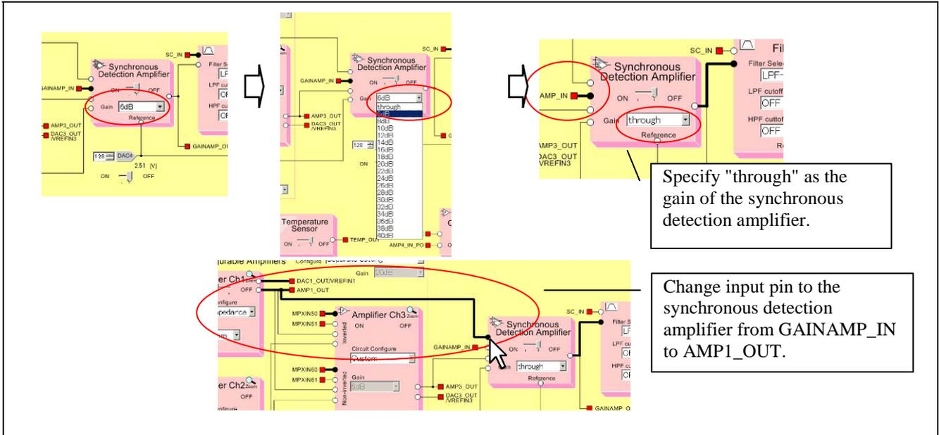
Figure 3-31 Connecting the Pin to the Filter
