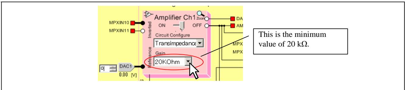
Figure 3-11 Specifying the Configurable Amplifier Gain
