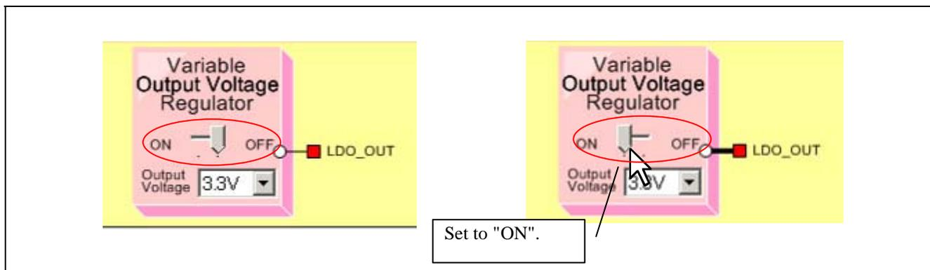
**Figure 3-14    Setting the Variable Output Voltage Regulator**
