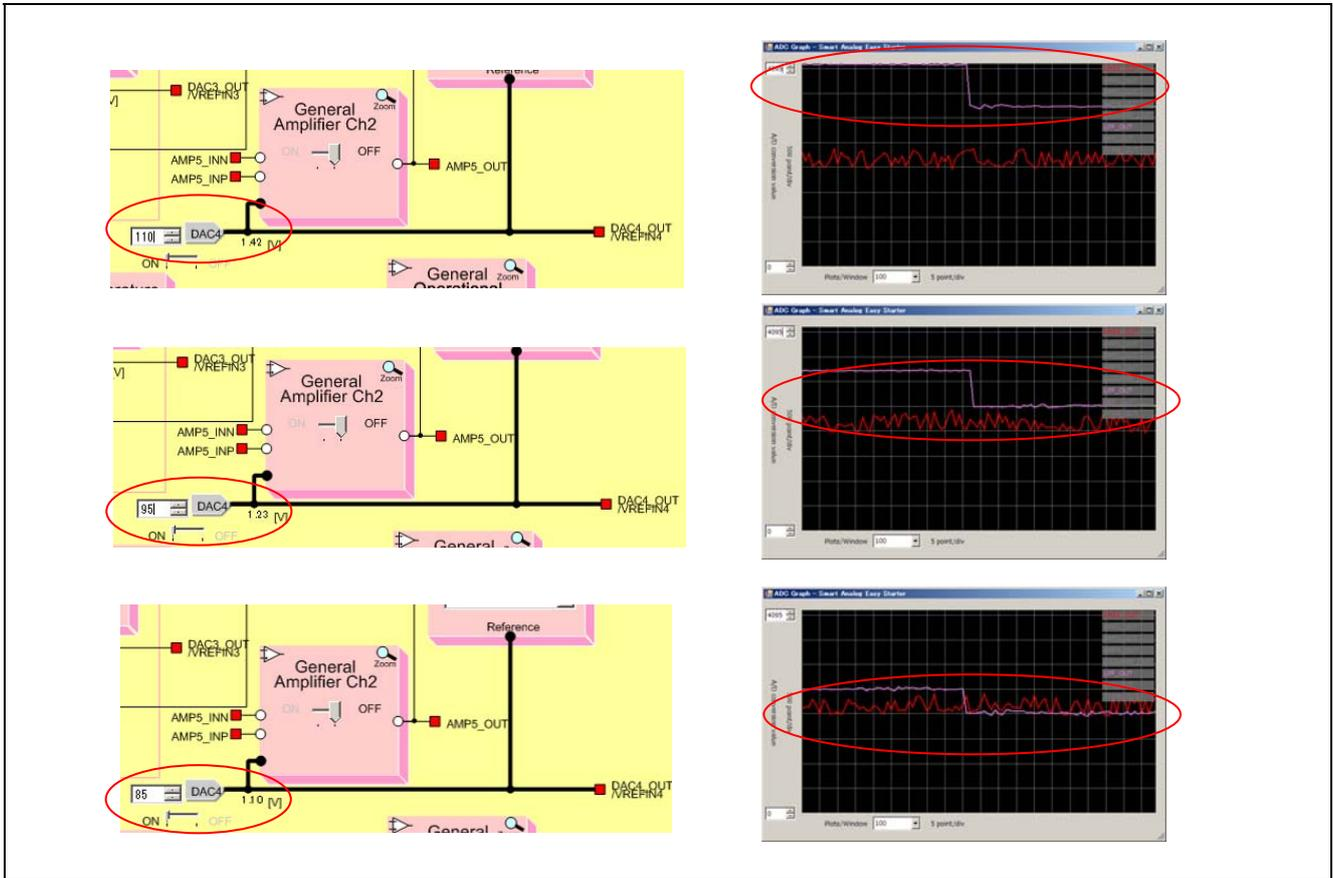
**Figure 3-42 Adjusting the Voltage Level at D/A Converter**
