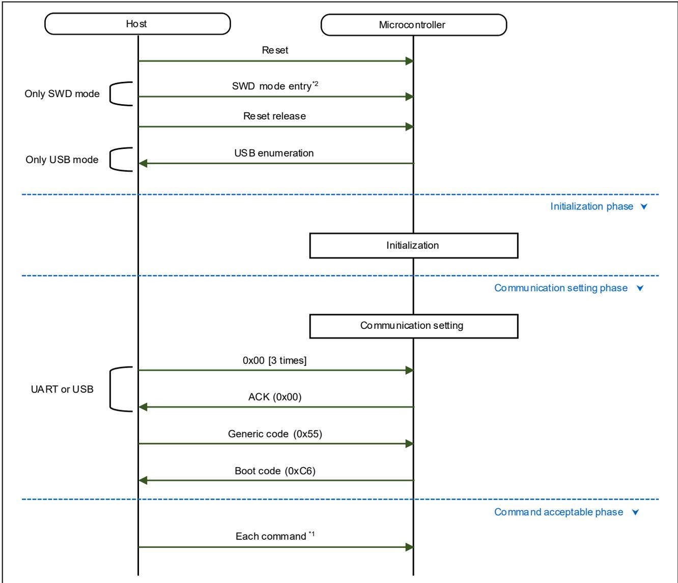
\*1 From the Command acceptable phase, the host and microcontroller send data in turn unless otherwise noted. The host executes data transmission after data reception from the microcontroller.
