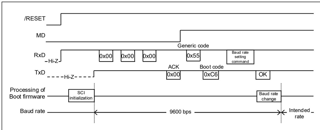
\* Boot firmware of GrpA, GrpB, and GrpC outputs High from TxD after SCI initialization. Boot firmware of GrpD enables pull-up of TxD after SCI initialization, and outputs High from TxD after 3-byte 00h reception. After SCI initialization, the boot firmware outputs High from TxD.
