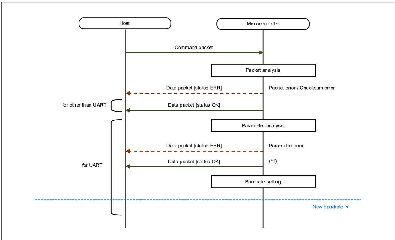
\*1: After this packet receiving, next command packet waits tBRT for keeping the baudrate setting time.
