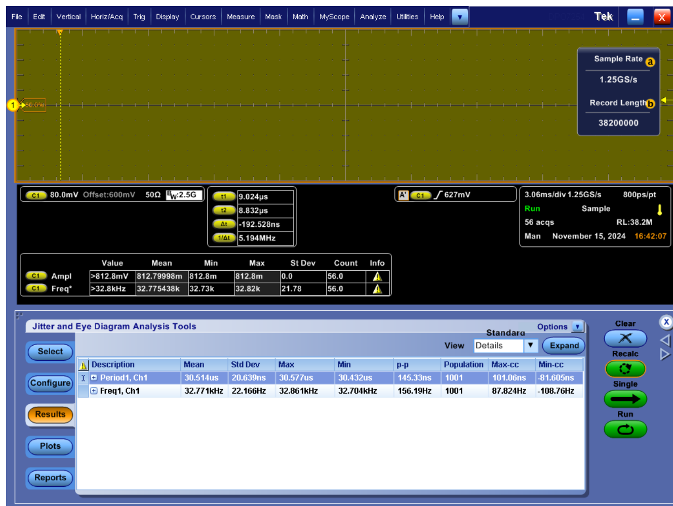
Figure 2. 32.768kHz with Low-Power DCO Mode
