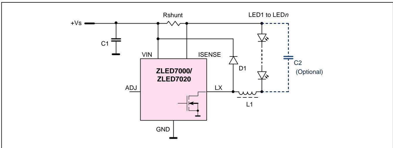
The current levels for the power transistor to turn on and off are determined by the voltage drop across Rshunt. An internal hysteresis comparator detects this voltage with an initial threshold of 95 mV (typical) with a symmetrical  $\pm 15\%$  hysteresis. The average LED current is defined as
