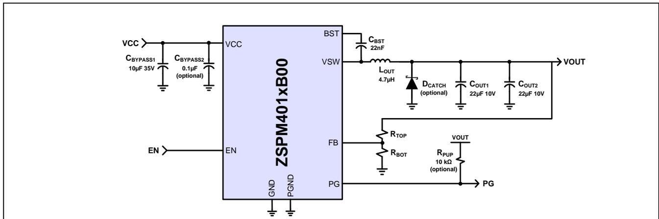
Figure 2.2 ZSPM4011/12/13 Application Schematic for Fixed Voltage Output
