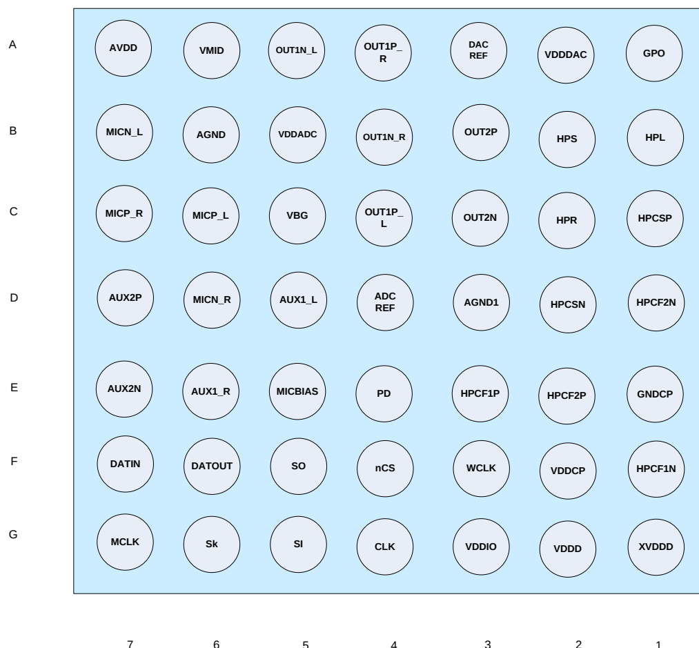
Figure 1: DA7210 pad arrangement for WLCSP version (Bottom view ball side up)
