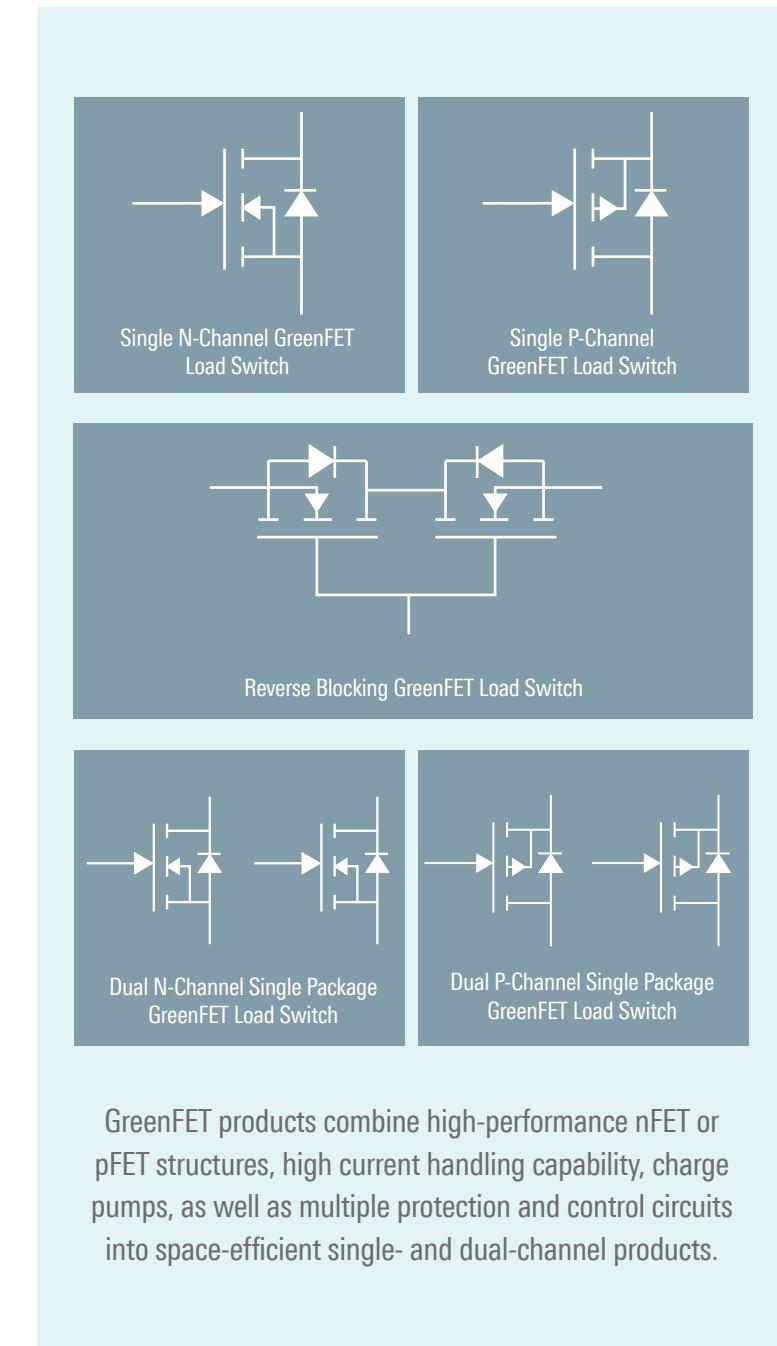
GreenFET products combine high-performance nFET or pFET structures, high current handling capability, charge pumps, as well as multiple protection and control circuits into space-efficient single- and dual-channel products.
