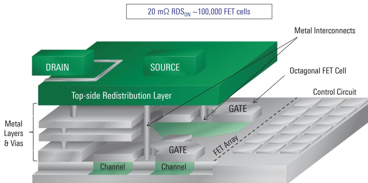
Combining Renesas' proprietary MOSFET IP and advanced assembly techniques, these advanced state-of-the-art products are available in ultra-small PCB footprints from 0.56 mm<sup>2</sup> to 4 mm<sup>2</sup> and exhibit low thermal resistances for high-current operation.
