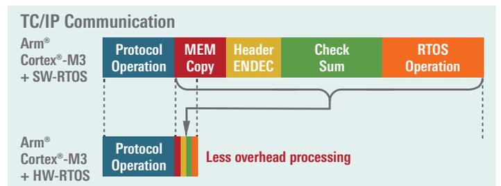
Effects on Ethernet Frame Processing: Drastic Reduction of Overhead Processing
