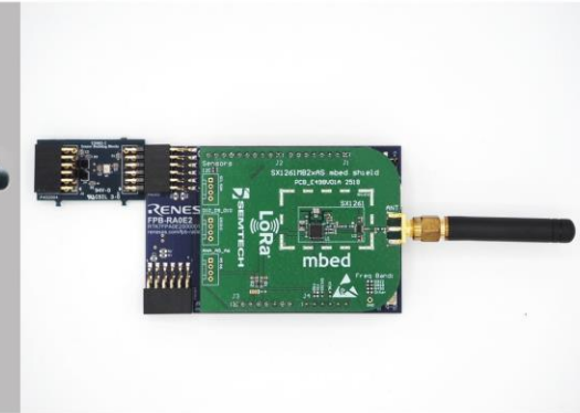
FPB-RA0E2 (RA0E2 Fast Prototyping Board) + SX1261/SX1262 Shield + HS3001 Humidity Sensor
