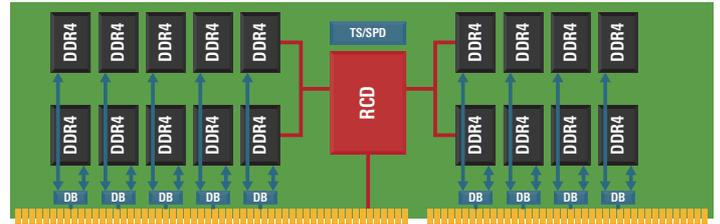
Renesas' DDR4 registered clock driver, data buffer and temp sensor make up the industry's first complete chipset for DDR4 registered dual inline memory modules (RDIMMs) and load reduced dual inline memory modules (LRDIMMs). With DDR4 data rates climbing to 3.2Gb/s and higher, the clear advantages afforded by RDIMM and LRDIMM as a speed-scalable memory technology are expected to drive adoption across a broad array of memory-intensive computing and storage applications.
