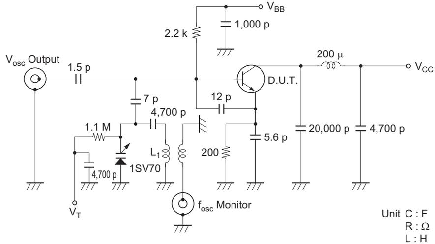
L<sub>1</sub> : Inside dia φ3 mm, φ3 mm Enameled Copper Wire 12 Turns
