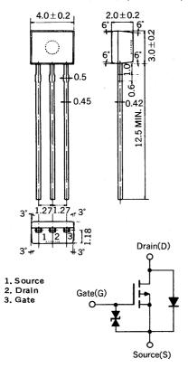
(Diode in the figure is the parasitic diode.)
