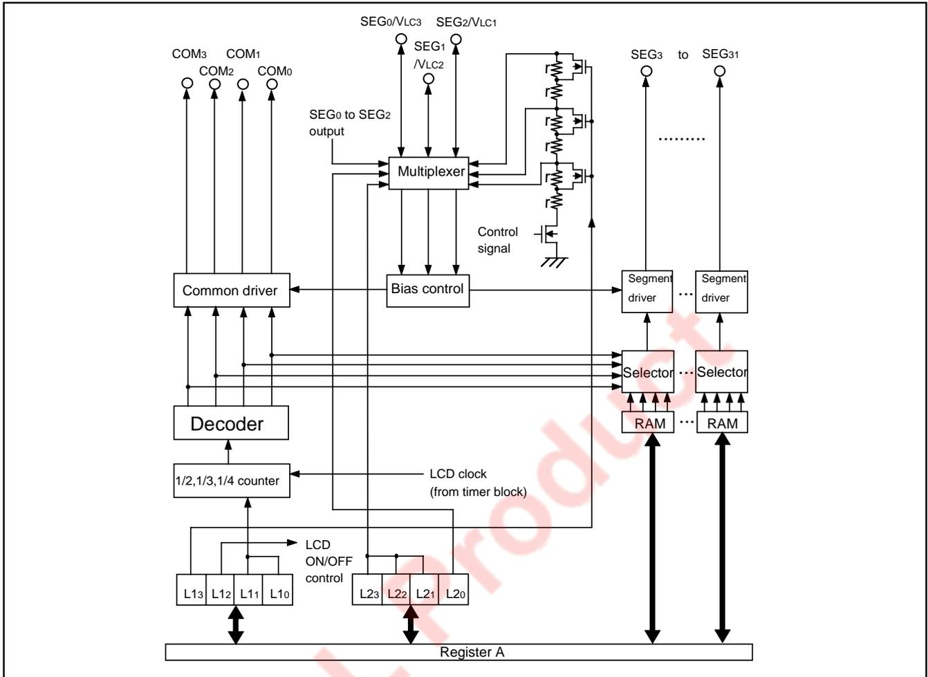
Fig. 34 LCD controller/driver
