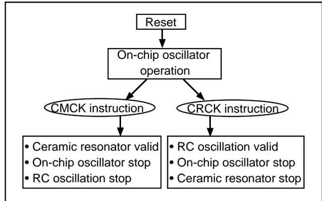
Fig. 48 Switch to ceramic resonance/RC oscillation
