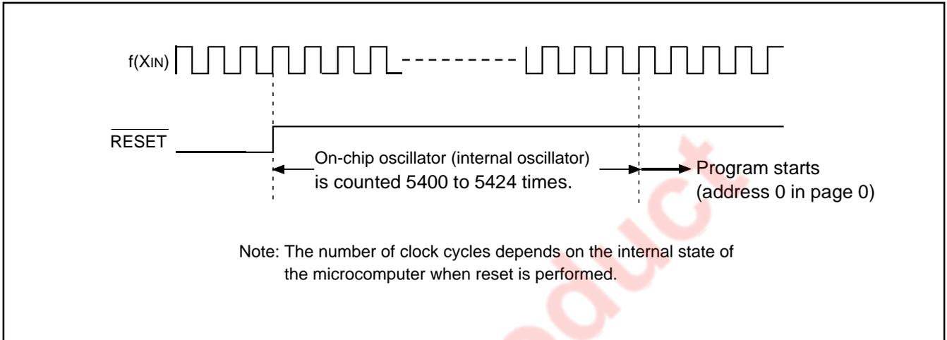
Fig. 37 Reset release timing
