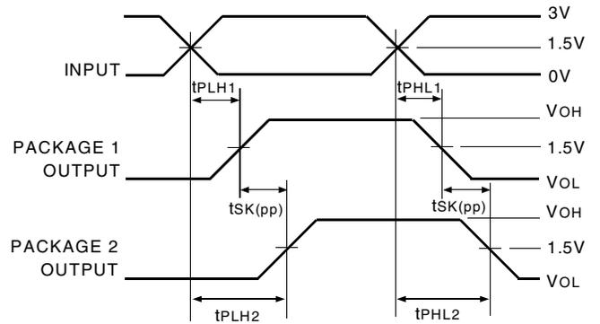
$$tsk(pp) = |t_{PLH2} - t_{PLH1}| \text{ or } |t_{PHL2} - t_{PHL1}|$$
