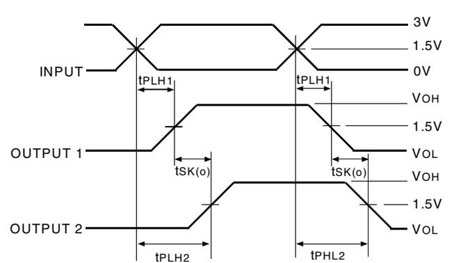
$$tsk(o) = |t_{PLH2} - t_{PLH1}| \text{ or } |t_{PHL2} - t_{PHL1}|$$
