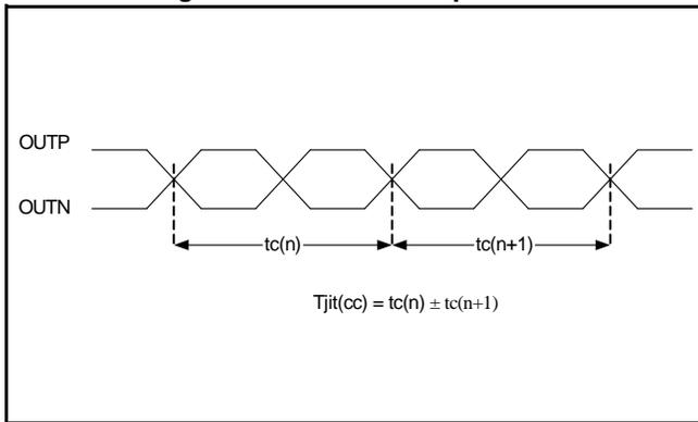
Figure 3: Cycle-cycle jitter
