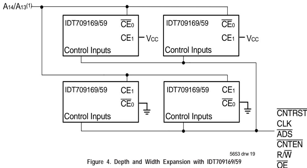
Figure 4. Depth and Width Expansion with IDT709169/59
