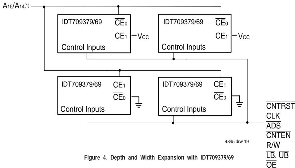
Figure 4. Depth and Width Expansion with IDT709379/69
