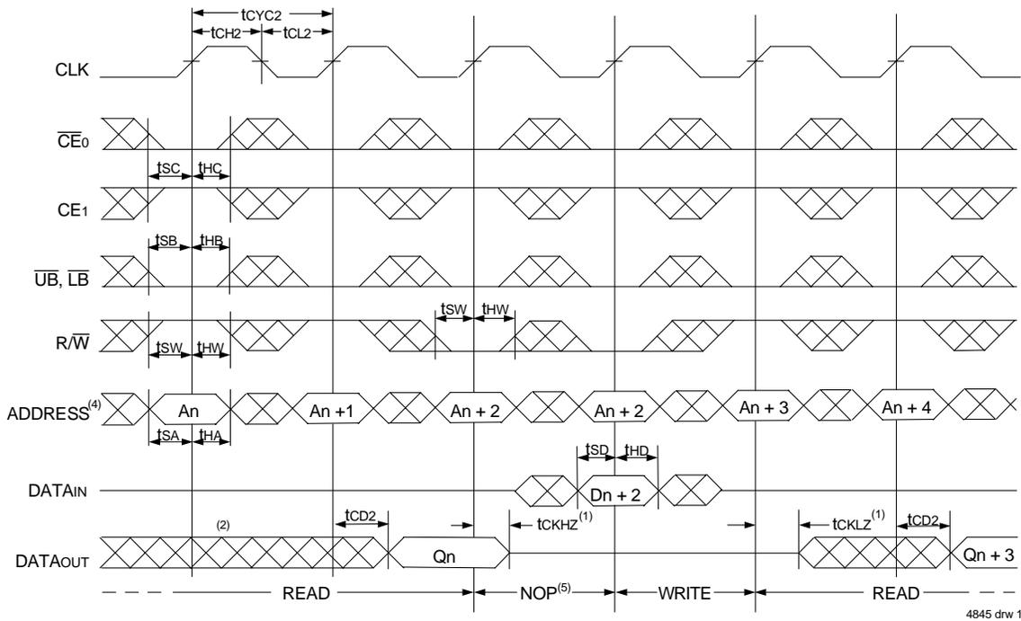
Timing Waveform of Pipelined Read-to-Write-to-Read ( $\overline{OE}$  Controlled)<sup>(3)</sup>
