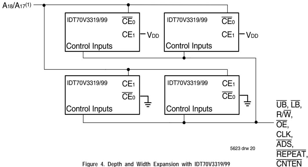
Figure 4. Depth and Width Expansion with IDT70V3319/99
