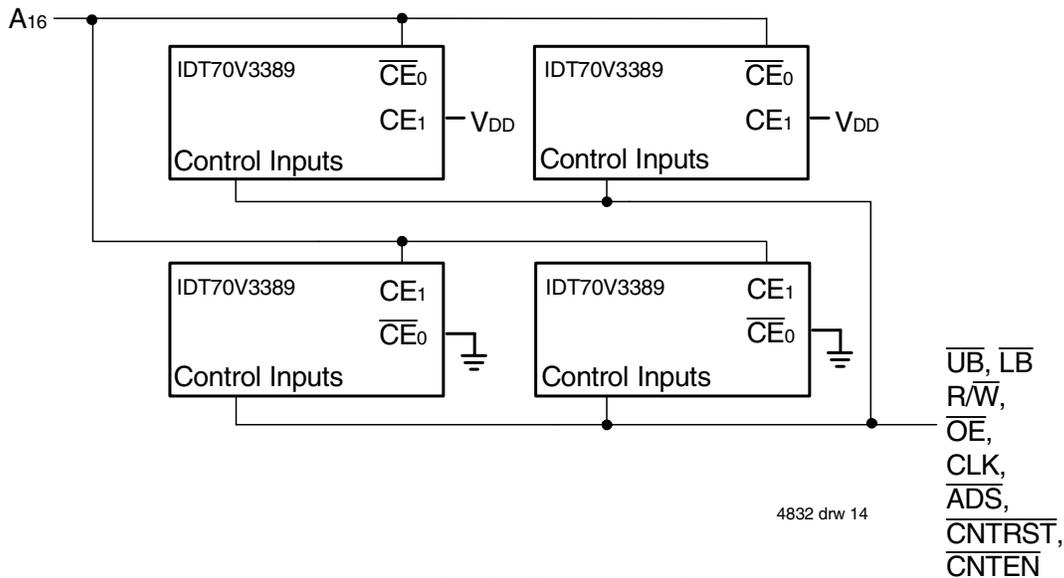
Figure 4. Depth and Width Expansion with IDT70V3389
