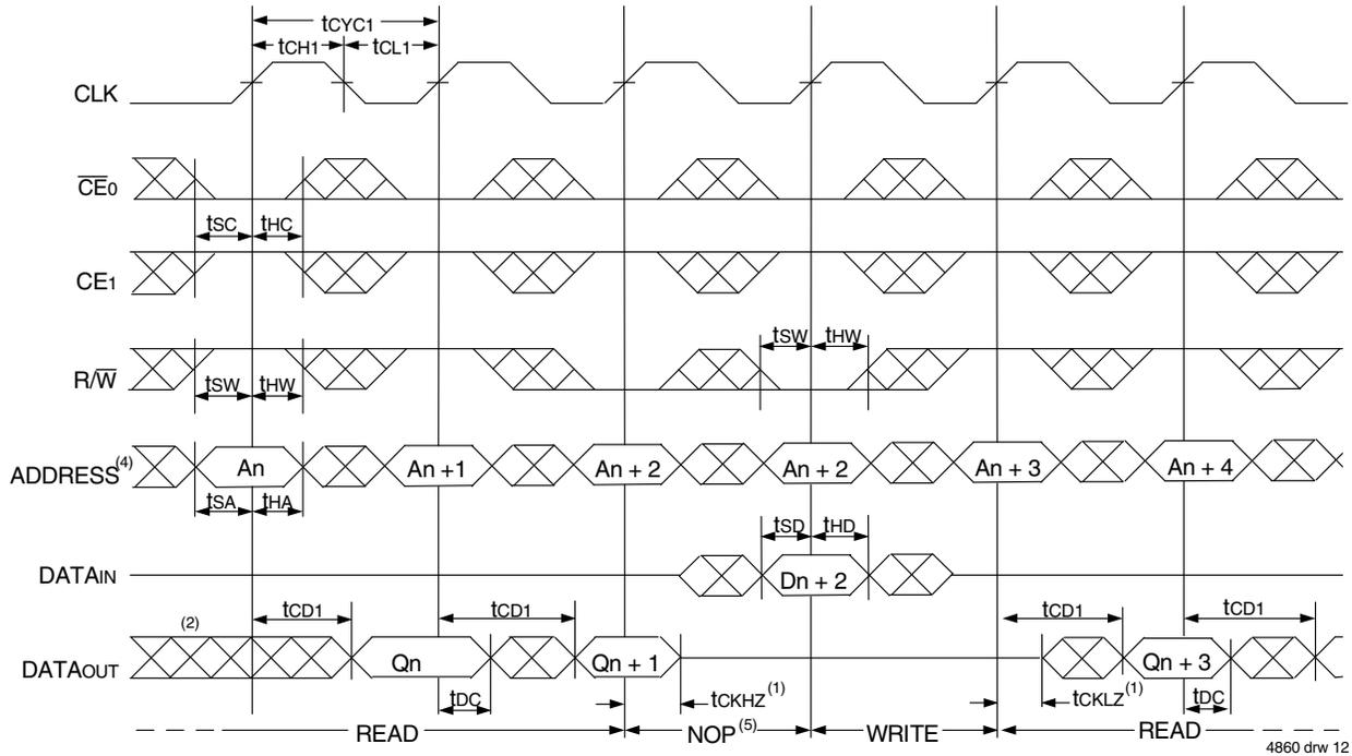
Timing Waveform of Flow-Through Read-to-Write-to-Read ( $\overline{OE}$  Controlled)<sup>(3)</sup>
