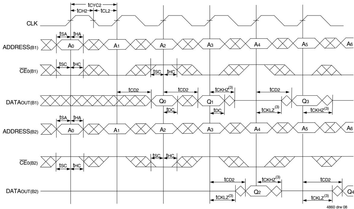
Timing Waveform of a Bank Select Flow-Through Read<sup>(6)</sup>
