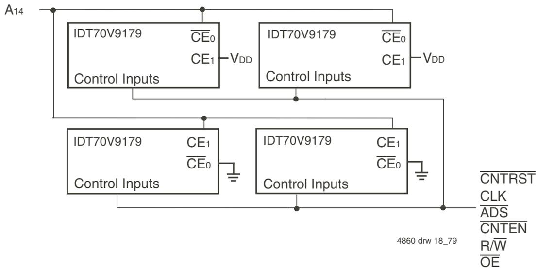
Figure 4. Depth and Width Expansion with IDT70V9179
