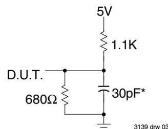
**Figure 1. Output Load**
