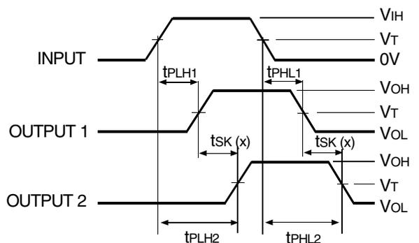
$$tsk(x) = |t_{PLH2} - t_{PLH1}| \text{ or } |t_{PHL2} - t_{PHL1}|$$
