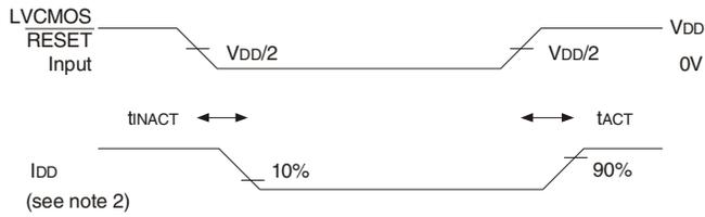
Voltage and Current Waveforms
