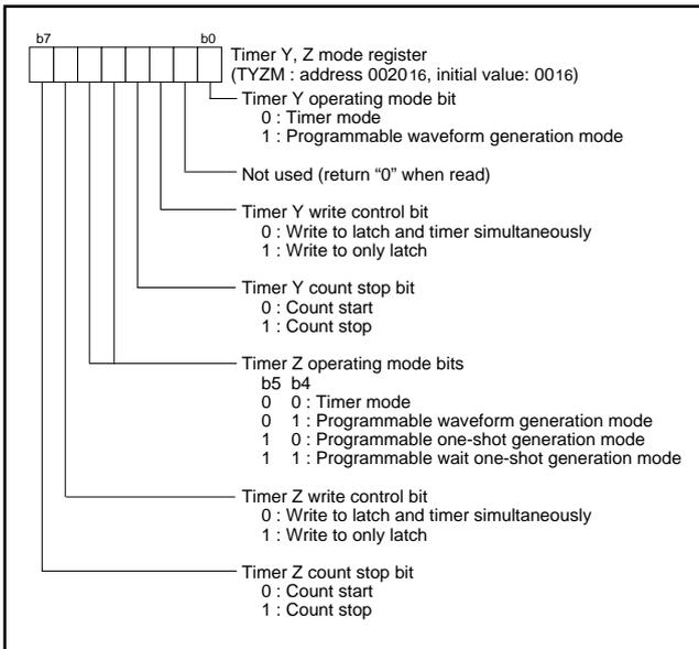
Fig. 25 Structure of timer Y, Z mode register
