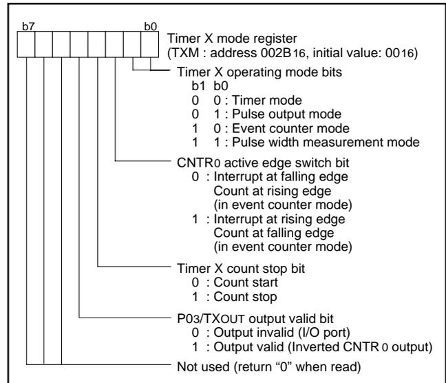
Fig. 23 Structure of timer X mode register
