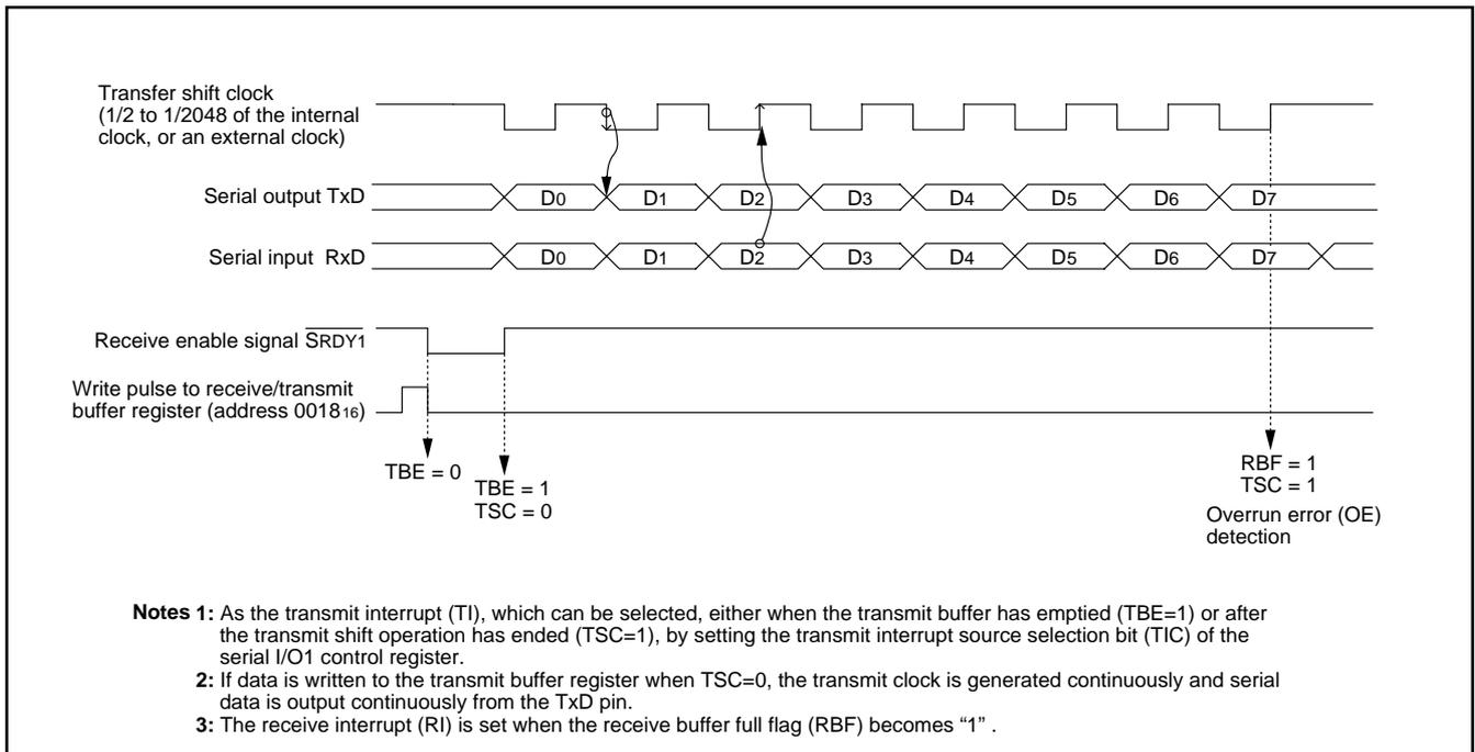
**Fig. 31 Operation of clock synchronous serial I/O1 function**
