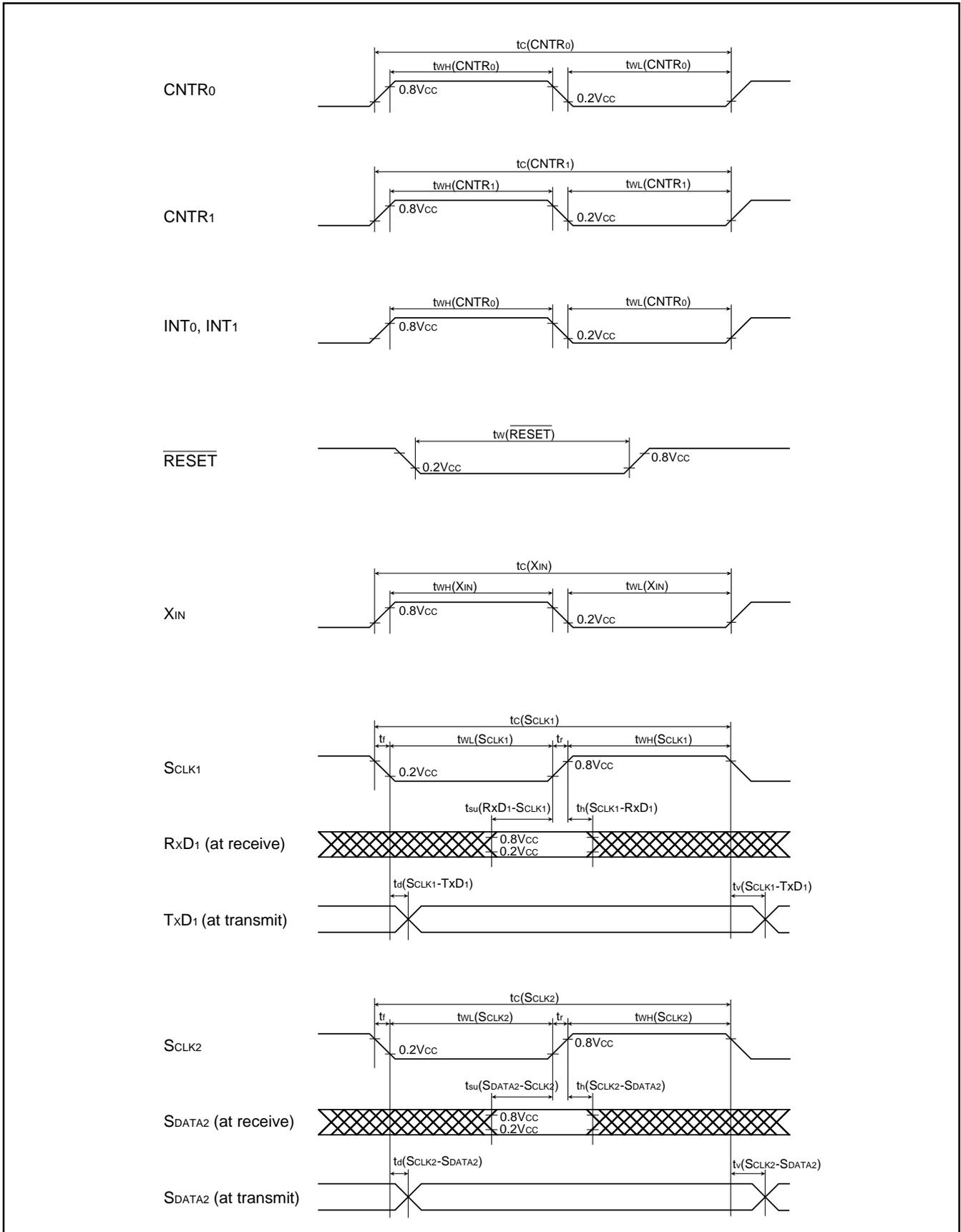
Fig. 57 Timing chart (Extended operating temperature 125 °C version)
