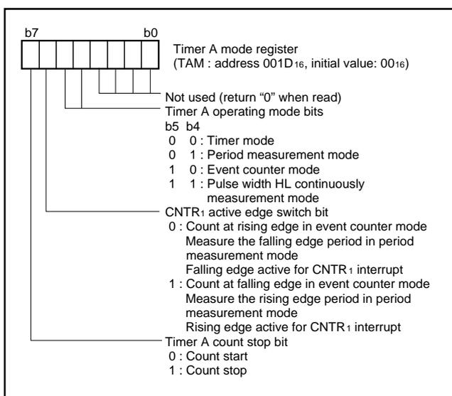
Fig. 22 Structure of timer A mode register
