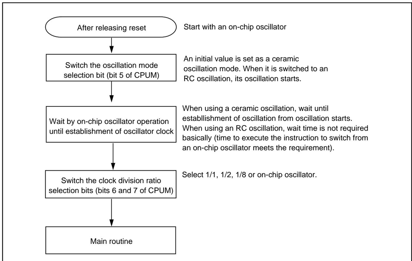
Fig. 12 Switching method of CPU mode register
