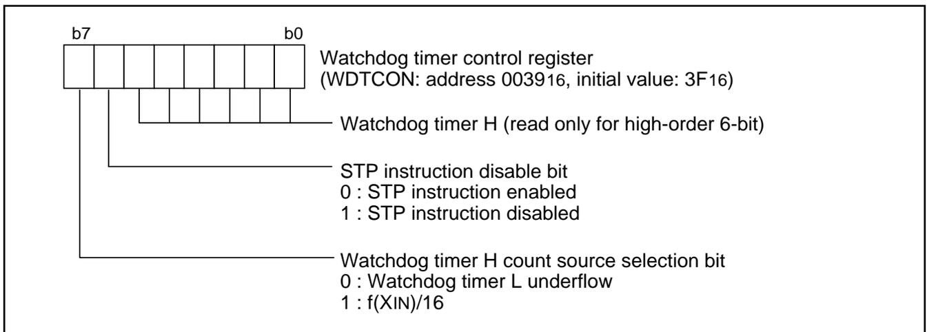
Fig. 42 Structure of watchdog timer control register
