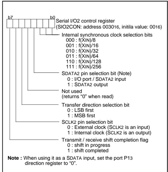
Fig. 35 Structure of serial I/O2 control registers
