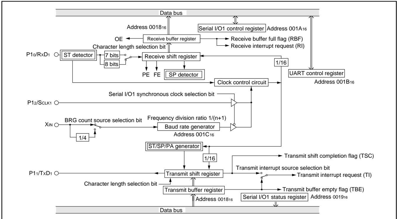
**Fig. 32 Block diagram of UART serial I/O1**
