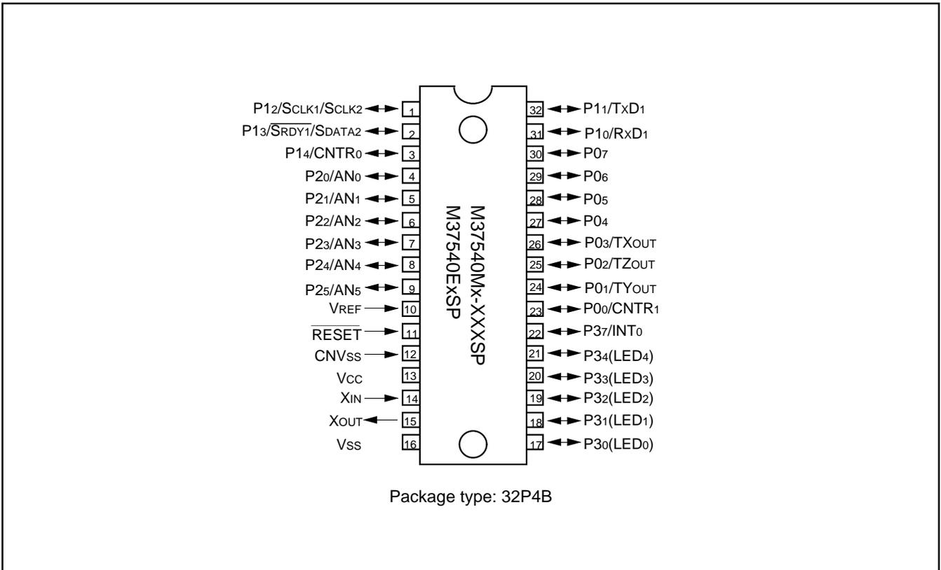
Fig. 3 Pin configuration (32P4B-A type)
