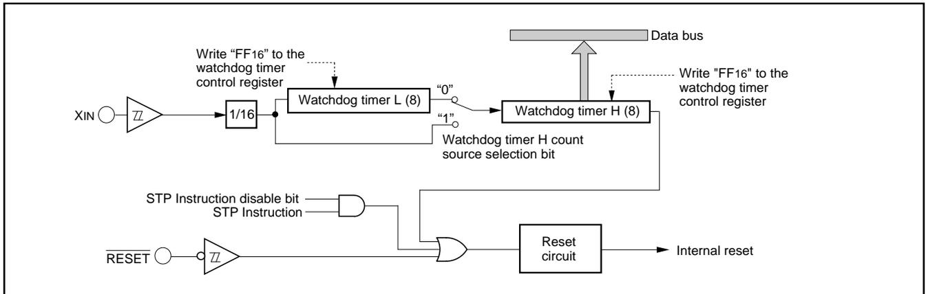
Fig. 41 Block diagram of watchdog timer
