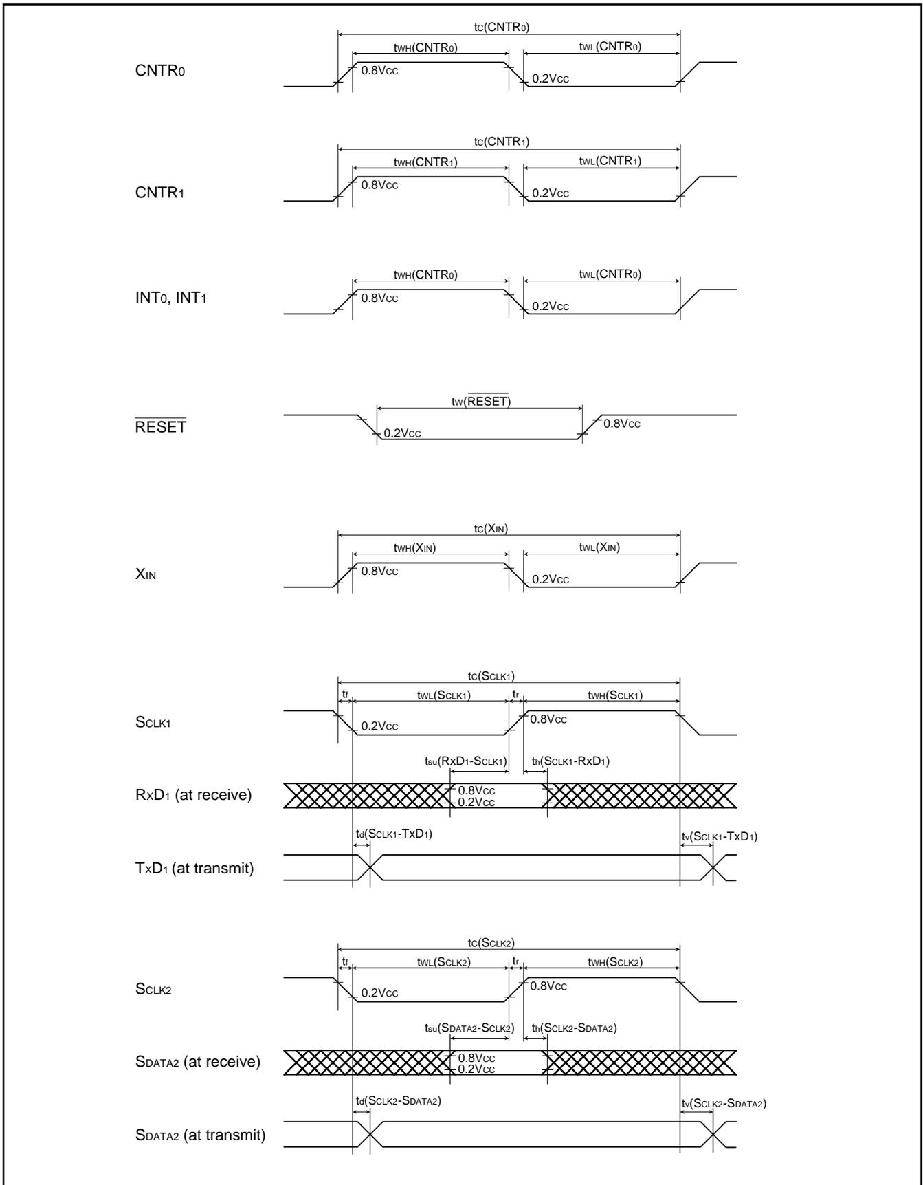
Fig. 56 Timing chart (Extended operating temperature version)
