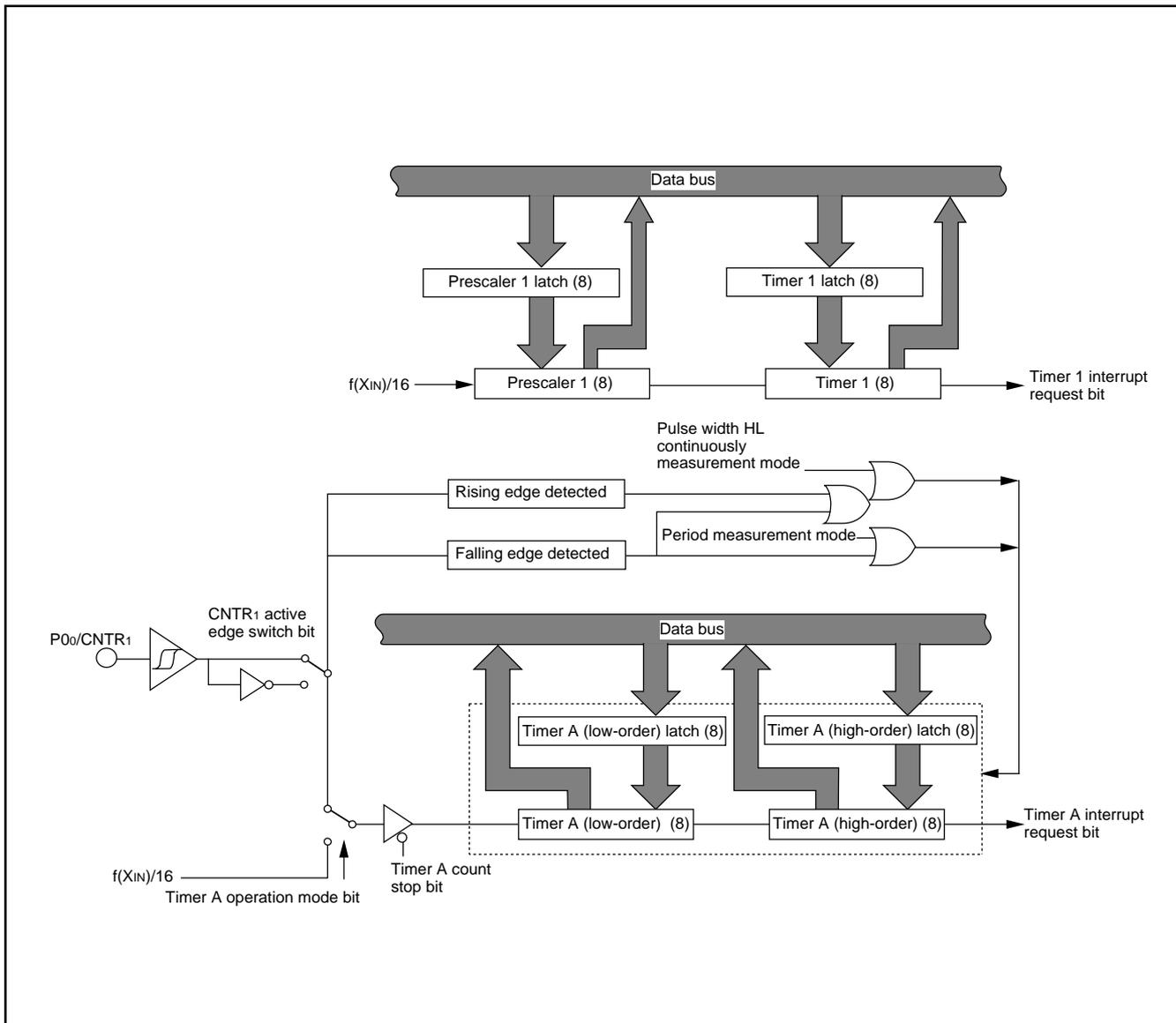
Fig. 28 Block diagram of timer 1 and timer A
