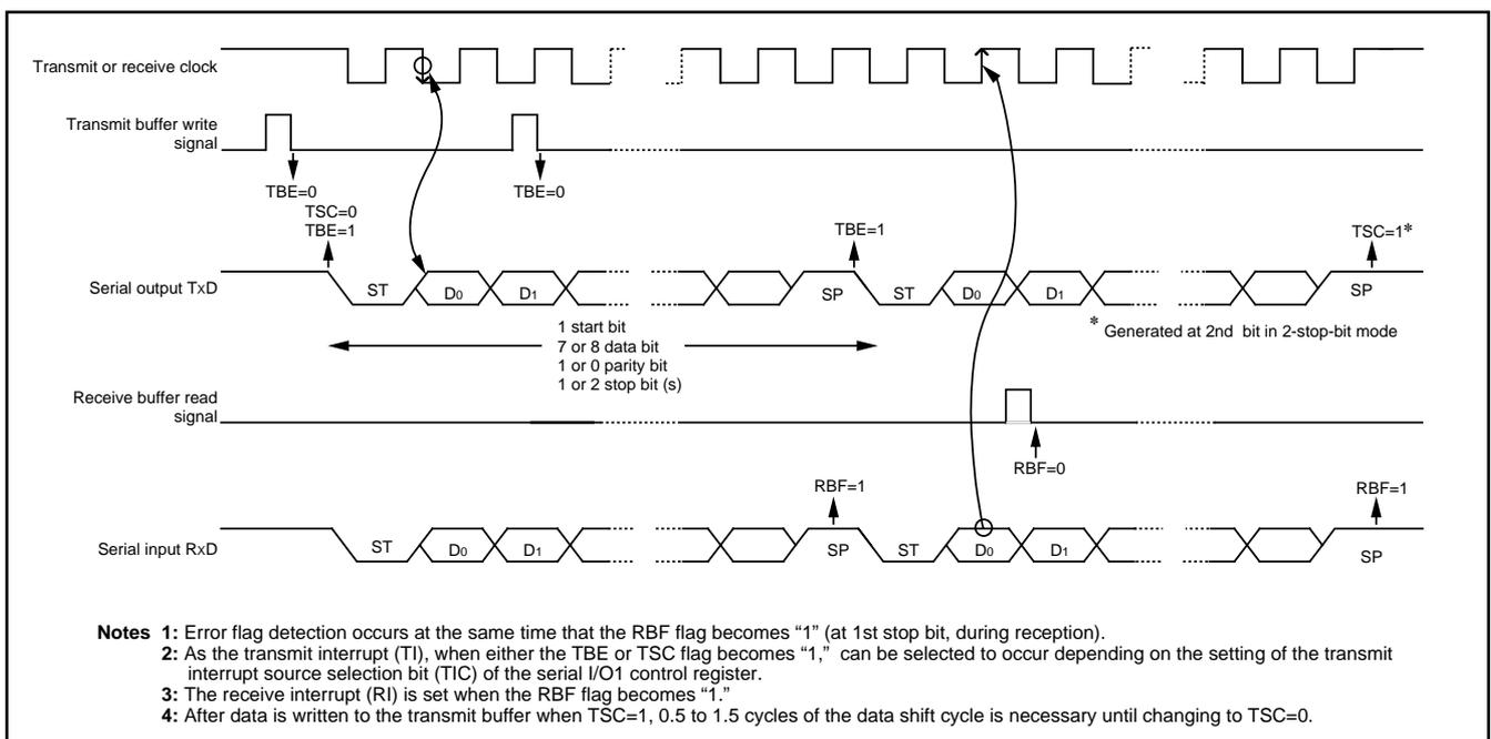
**Fig. 33 Operation of UART serial I/O1 function**
