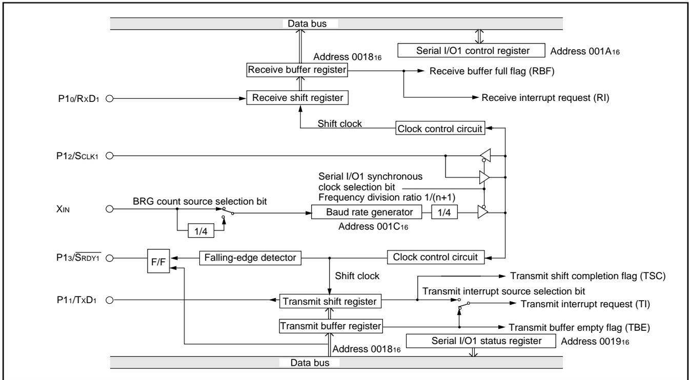
**Fig. 30 Block diagram of clock synchronous serial I/O1**
