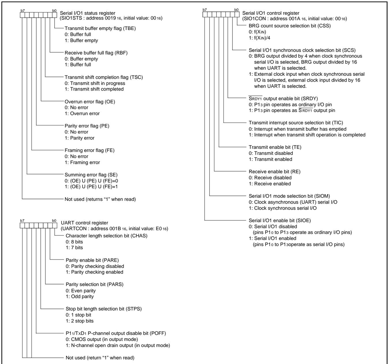
Fig. 34 Structure of serial I/O1-related registers
