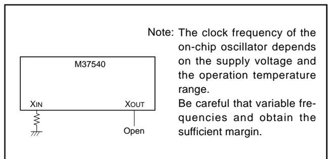
Fig. 49 Processing of XIN and XOUT pins at on-chip oscillator operation
