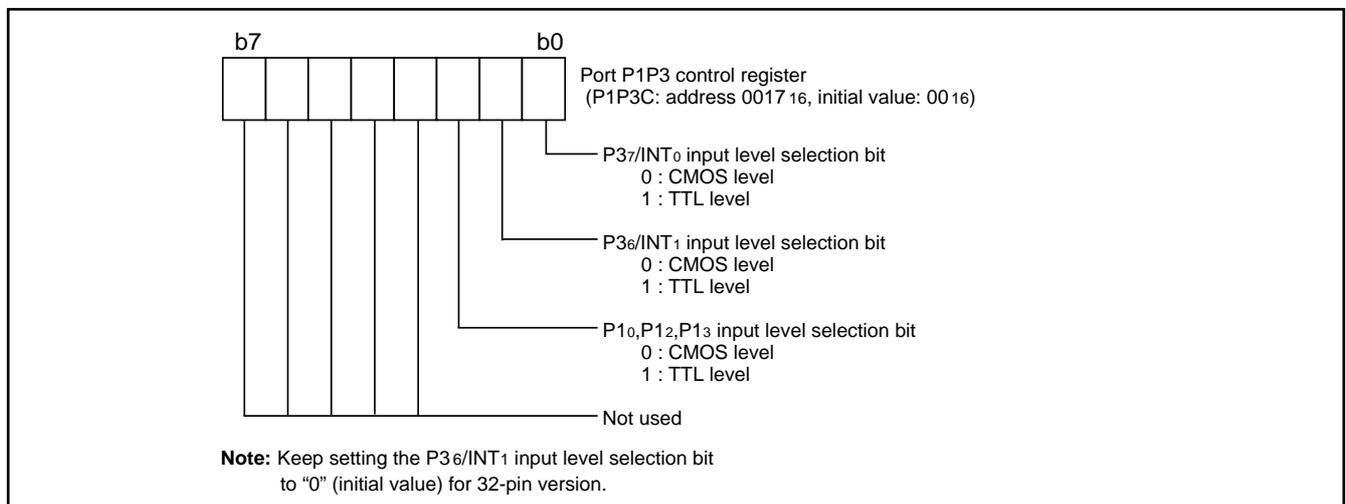
Fig. 16 Structure of port P1P3 control register
