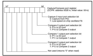
Fig 33. Structure of capture/compare port register
