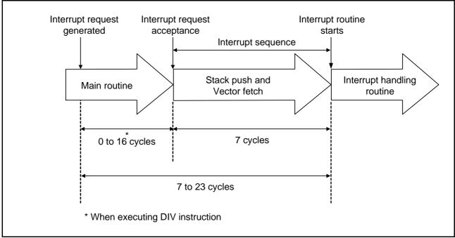
Fig 21. Time up to execution in interrupt routine
