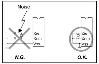
Fig 75. Wiring for clock I/O pins
