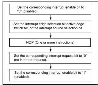
Fig 90. Sequence of changing relevant register
