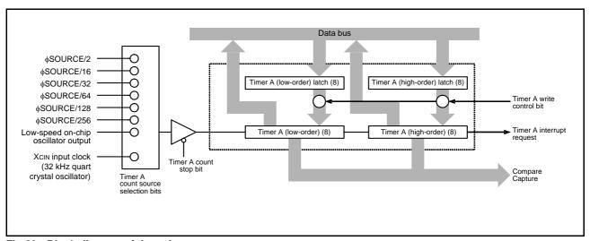
Fig 29. Block diagram of timer A
