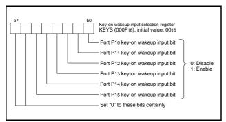
Fig 25. Structure of key input control register
