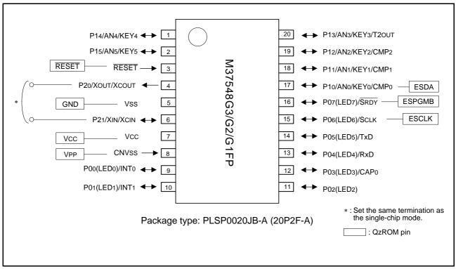
Fig 70. Pin connection diagram (M37548G3/G2/G1FP)
