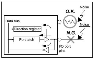
Fig 80. Setup for I/O ports
