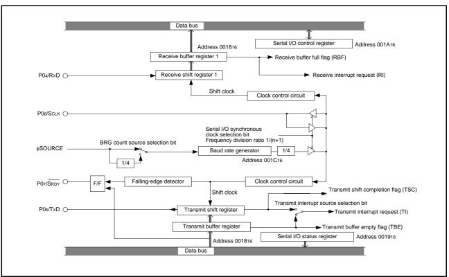
Fig 46. Block diagram of clock synchronous serial I/O
