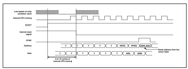
Fig 59. Timing diagram at reset
