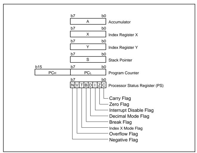
Fig 5. 740 Family CPU register structure
