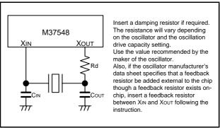
Fig 62. External circuit of ceramic resonator
