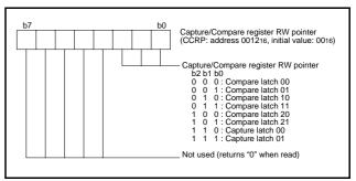
Fig 31. Structure of capture/compare register RW pointer
