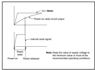
Fig 57. Operation waveform diagram of power-on reset circuit
