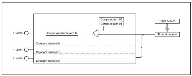
Fig 37. Block diagram of compare output circuit
