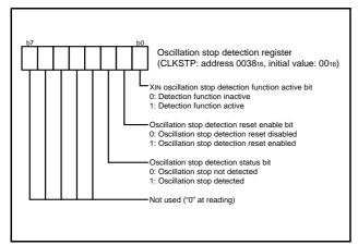
Fig 68. Structure of oscillation stop detection register
