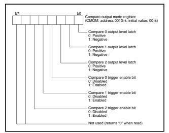
Fig 34. Structure of compare output mode register
