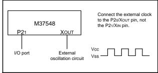
Fig 64. External clock input circuit
