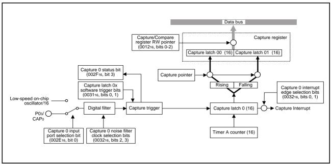
Fig 43. Block diagram of capture channel 0
