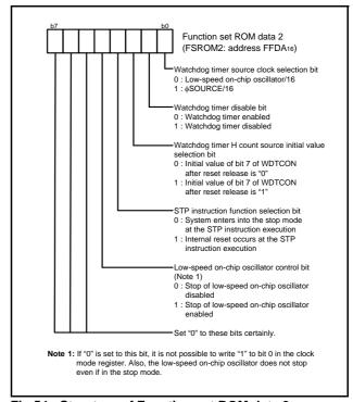
Fig 54. Structure of Function set ROM data 2
