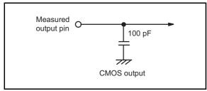
Fig 85. Switching characteristics measurement circuit diagram
