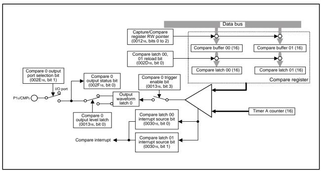
Fig 38. Block diagram of compare channel 0
