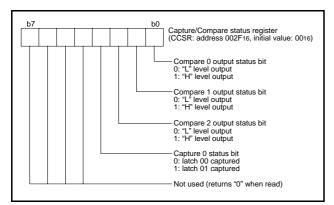
Fig 35. Structure of capture/compare status register
