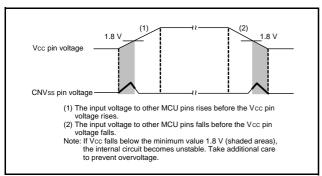
Fig 82. Timing Diagram (bold-lined periods are applicable)
