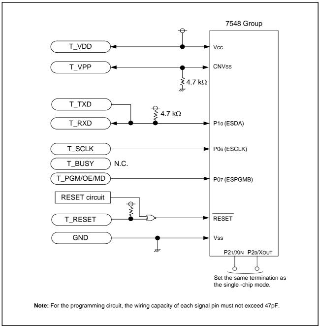
Fig 72. When using programmer of Suisei Electronics System Co., LTD, connection example
