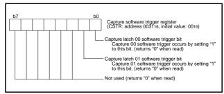
Fig 41. Structure of capture software trigger register
