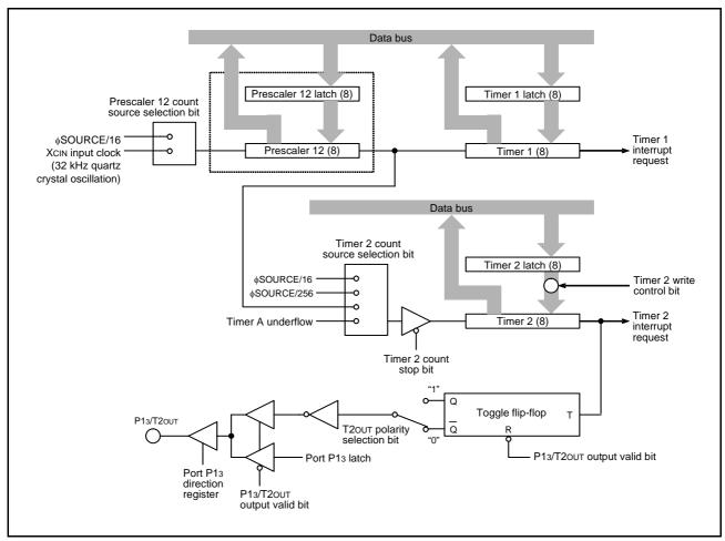
Fig 28. Block diagram of timer 1 and timer 2
