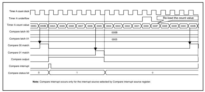
Fig 39. Output compare mode (general waveform)
