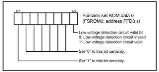
Fig 10. Structure of Function set ROM data 0
