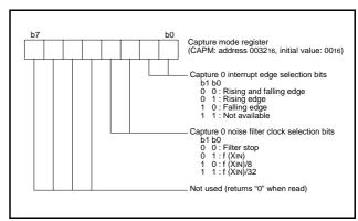
Fig 42. Structure of capture mode register
