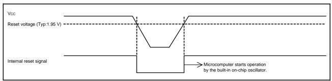
Fig 58. Operation waveform diagram of low voltage detection circuit
