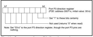
Fig 16. Structure of port P3 direction register
