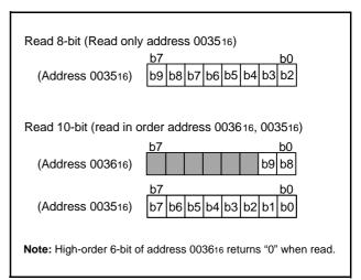
Fig 52. Structure of AD conversion register
