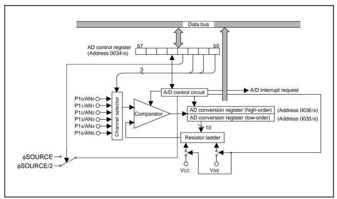
Fig 53. Block diagram of A/D converter
