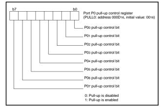
Fig 14. Structure of port P0 pull-up control register
