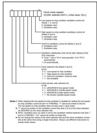
Fig 65. Structure of clock mode register
