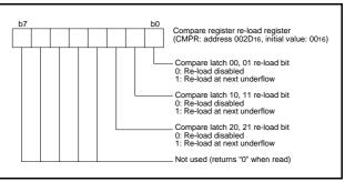
Fig 32. Structure of compare register re-load register
