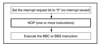
Fig 91. Sequence of check of interrupt request bit
