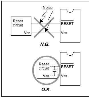
Fig 74. Wiring for the RESET pin
