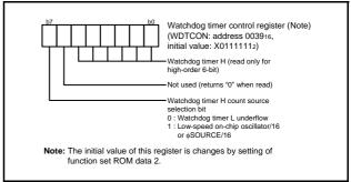
Fig 55. Structure of watchdog timer control register
