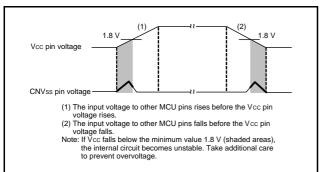
Fig 92. Timing Diagram (bold-lined periods are applicable)
