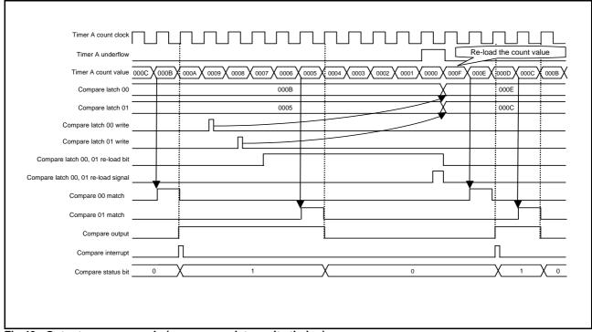
Fig 40. Output compare mode (compare register write timing)
