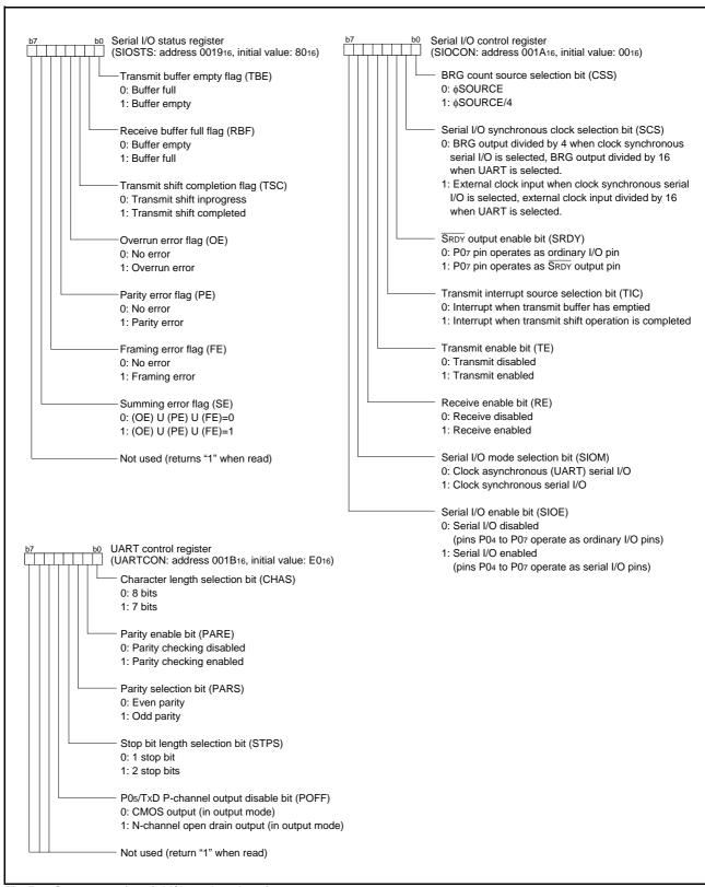
Fig 50. Structure of serial I/O1-related registers
