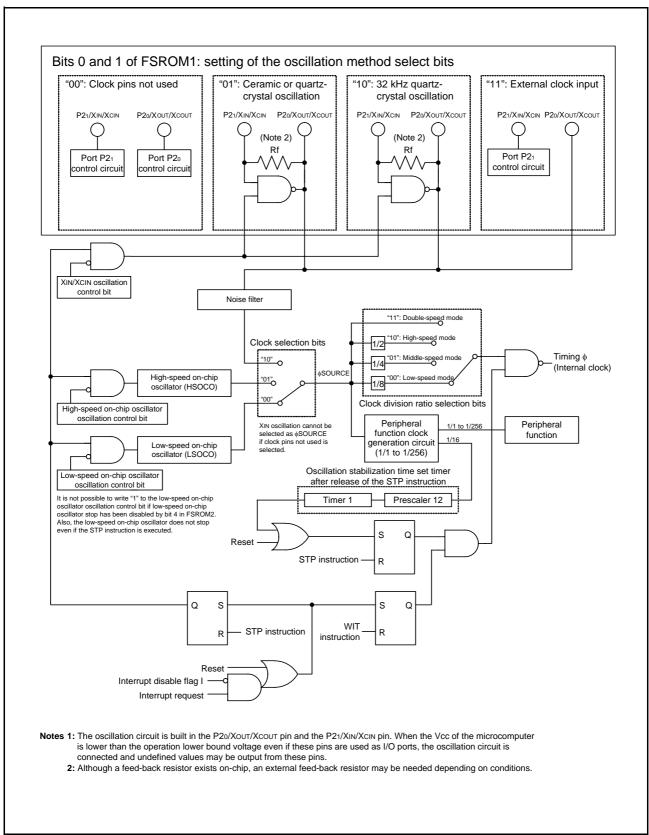
Fig 66. Block diagram of internal clock generating circuit
