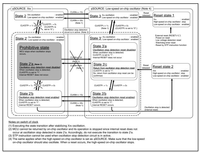
Fig 69. State transition of oscillation stop detection circuit
