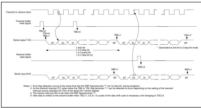
Fig 49. Operation of UART serial I/O function
