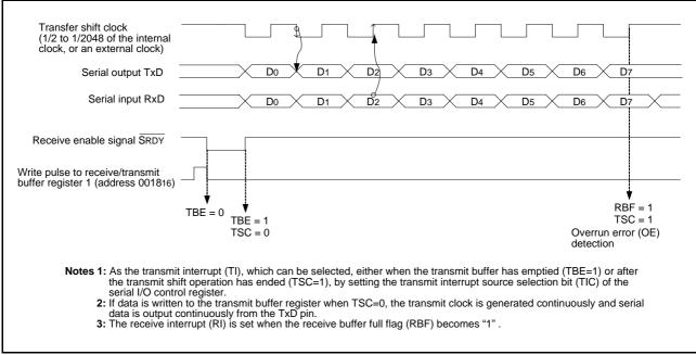
Fig 47. Operation of clock synchronous serial I/O function
