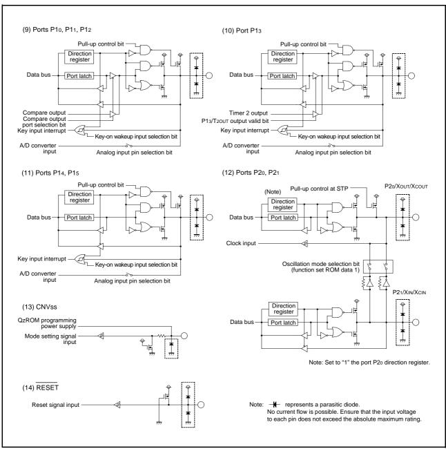
Fig 18. Block diagram of pins (2)
