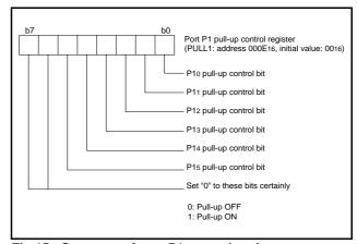
Fig 15. Structure of port P1 control register
