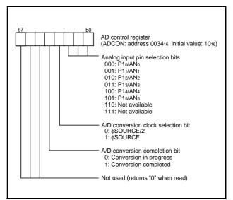
Fig 51. Structure of AD control register
