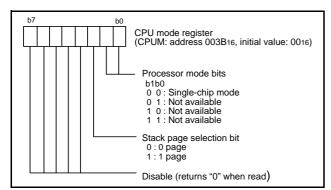
Fig 7. Structure of CPU mode register
