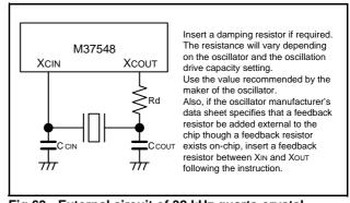
Fig 63. External circuit of 32 kHz quarts-crystal oscillator
