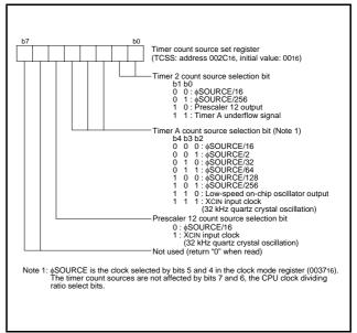
Fig 27. Structure of timer count source set register
