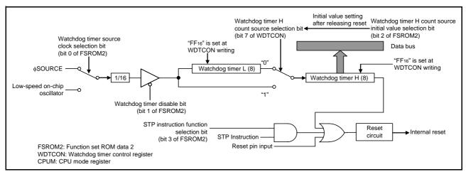
Fig 56. Block diagram of watchdog timer
