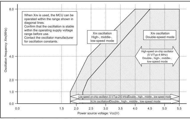
Fig 83. Power source voltage and oscillation frequency
