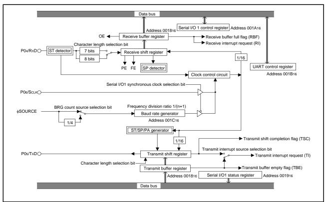
Fig 48. Block diagram of UART serial I/O
