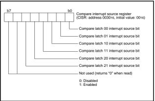
Fig 36. Structure of compare interrupt source register
