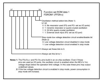
Fig 61. Structure of function set ROM data 1
