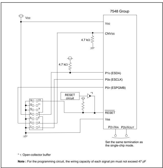
Fig 71. When using E8 programmer, connection example
