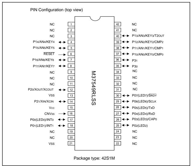
Fig 2. Pin configuration (42S1M type)
