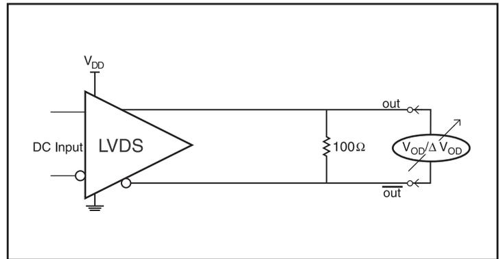
Differential Output Voltage Setup Propagation Delay
