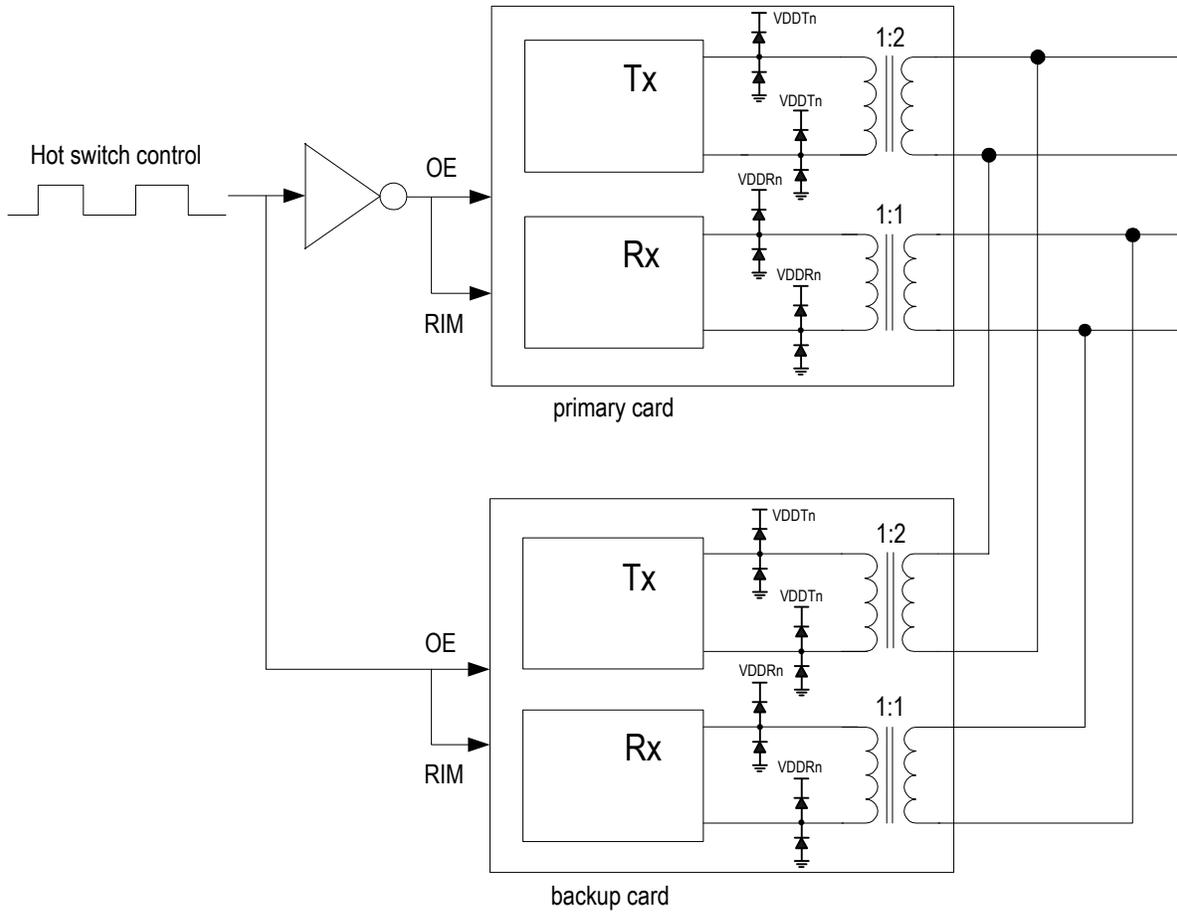
**Rx:** Fully Internal Impedance Matching mode. In this mode, there is no external resistor required. The R\_TERM[2:0] bits (b2~0, RCF0,...) setting is as follows: '010' for E1 120 Ω twisted pair cable and '011' for E1 75 Ω coaxial cable.
