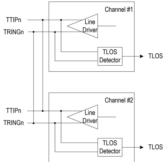
Figure-16 TLOS Detection Between Two Channels
