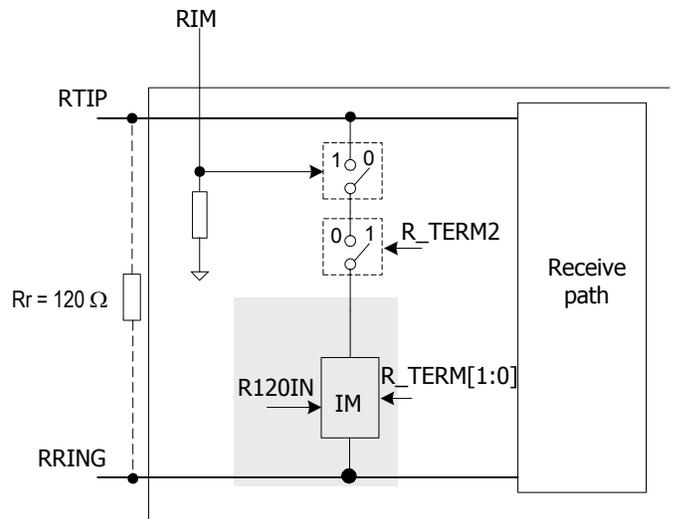
Figure-3 Switch between Impedance Matching Modes
