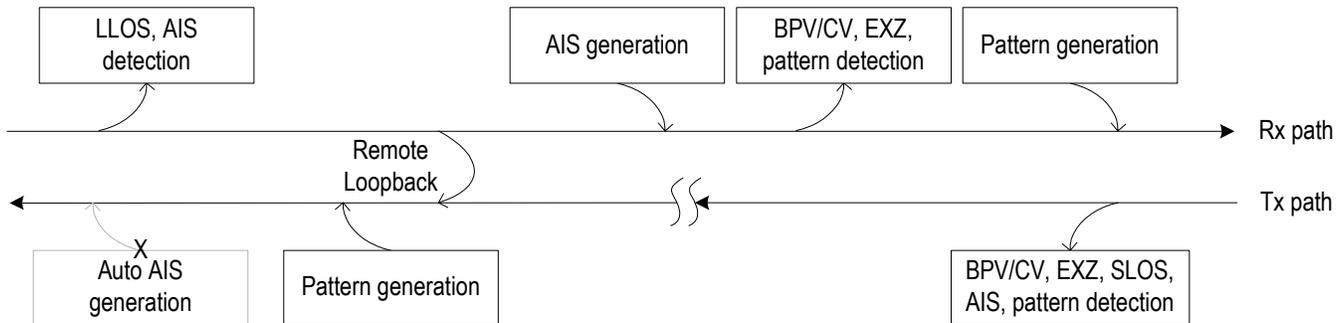
**Figure-24 Priority Of Diagnostic Facilities During Manual Remote Loopback**
