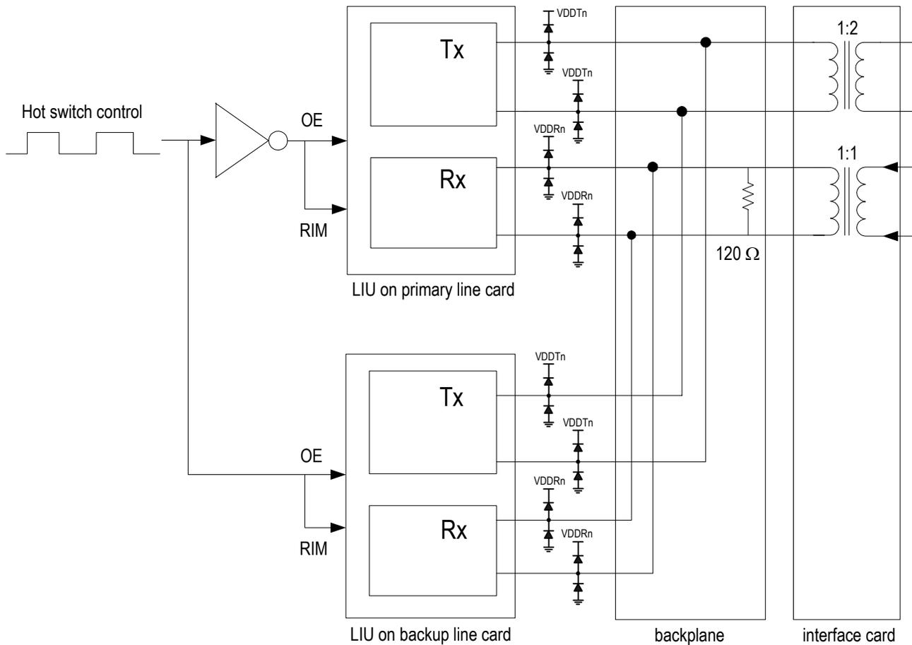
**Rx:** Partially Internal Impedance Matching mode. A fixed external 120 Ω resistor is placed on the backplane and provides a common termination for E1 applications. The R\_TERM[2:0] bits (b2~0, RCF0,...) setting is as follows: '010' for E1 120 Ω twisted pair cable and '011' for E1 75 Ω coaxial cable.
