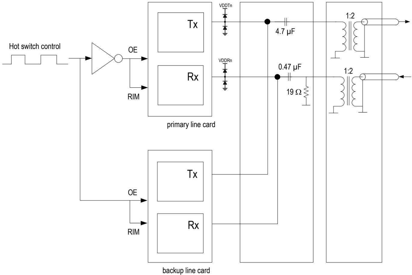
**Rx:** 75 Ω External Impedance Matching mode. In this mode, there is no external resistor required. The RIM pin should be left open and the configuration of the R\_TERM[2:0] bits (b2~0, RCF0,...) is ignored.
